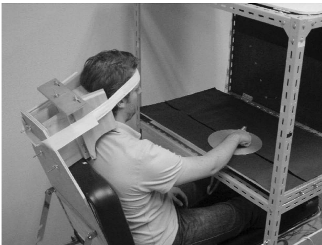
Figure 2. Apparatus and patient positioning for the subjective straight-ahead test.
