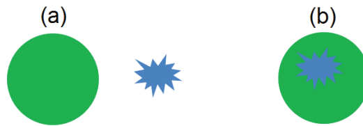
Figure 1.2 Illustration of the external (a) and internal (b) mixing of atmospheric particles.
