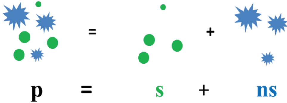
Figure 2.3 Scheme of a two-component particle external mixture composed of spherical and nonspherical particles. The backscattering coefficient \beta_p of the particle mixture is the sum of the backscattering coefficient of each component (i.e. \beta_s and \beta_{ns} ).
