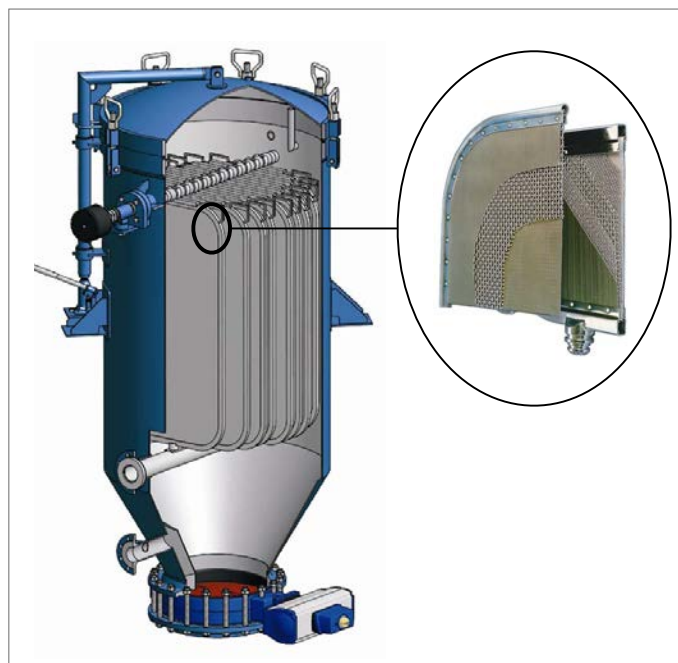
Figure 9. Vertical pressure leaf filter. Highlighted area illustrates a sectional view of a leaf. (Source: Filter MVDCD, © MAHLE Industrial Filtration, Alkmaar, The Netherlands)
