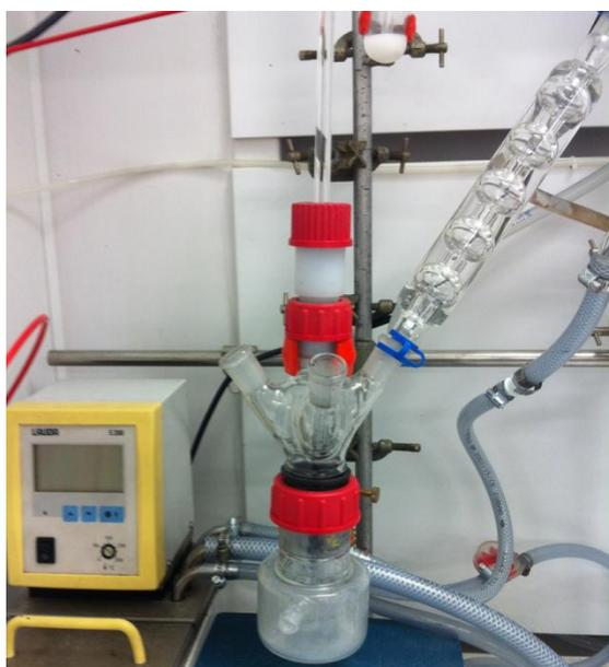
**Figure 8.** Picture of the 50 mL polymerization reactor
