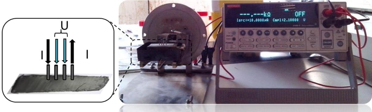
*Figure 3. Four-probe galvanometer equipment*
