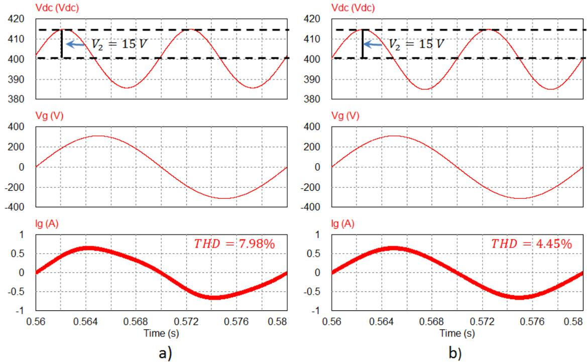
Fig. 4.14. Influence of the voltage ripple in the current harmonic distortion ( $L = 10$  mH,  $C = 27$   $\mu$ F):
