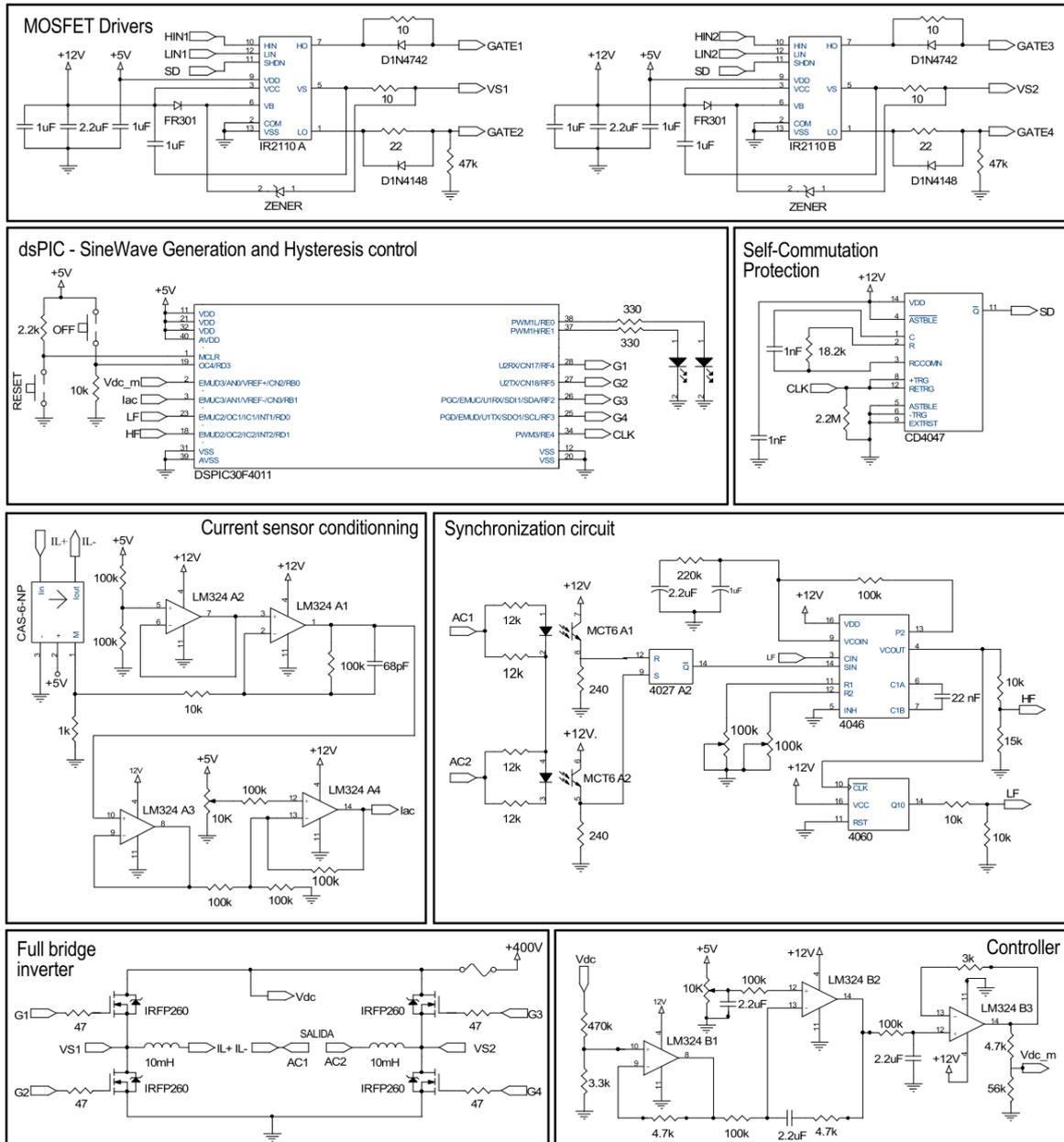
Fig. 4.25. Schematic circuit diagram of the power source inverter
