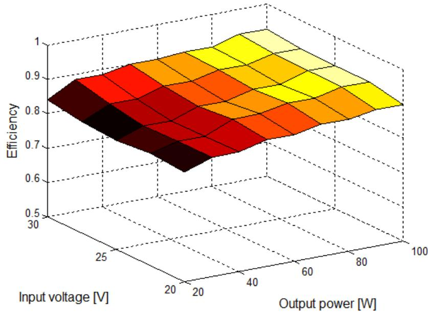
Fig. 3.32. Efficiency surface as a function of the input voltage and the output power
