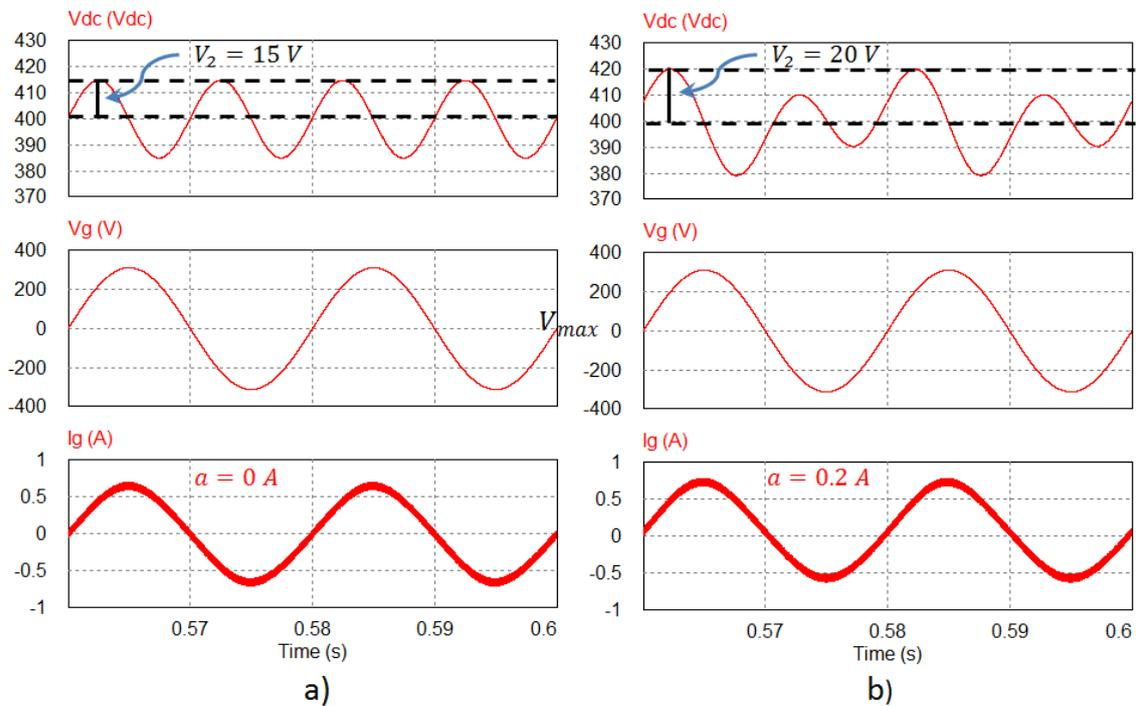
Fig. 4.15. Simulated voltage ripple on the DC bus: a) without DC component; b) with DC component.
