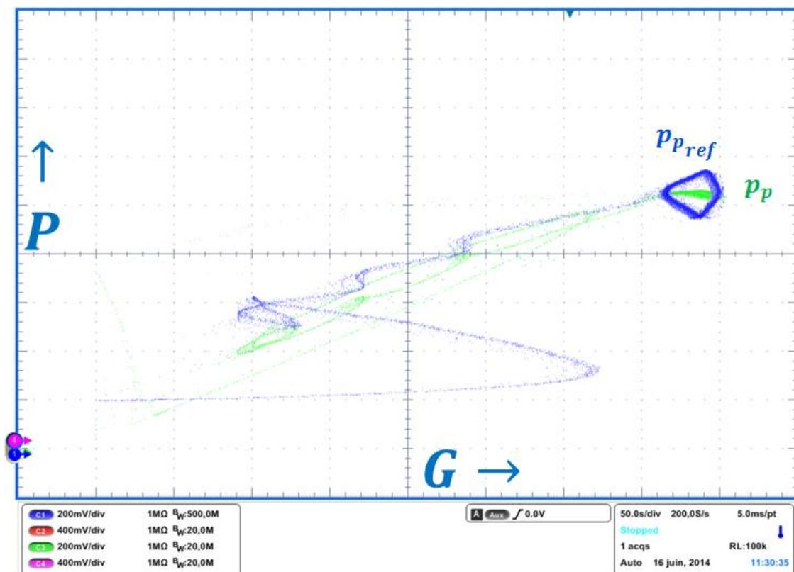
Fig. 2.31. Steady-state behavior of the proposed MPPT algorithm
