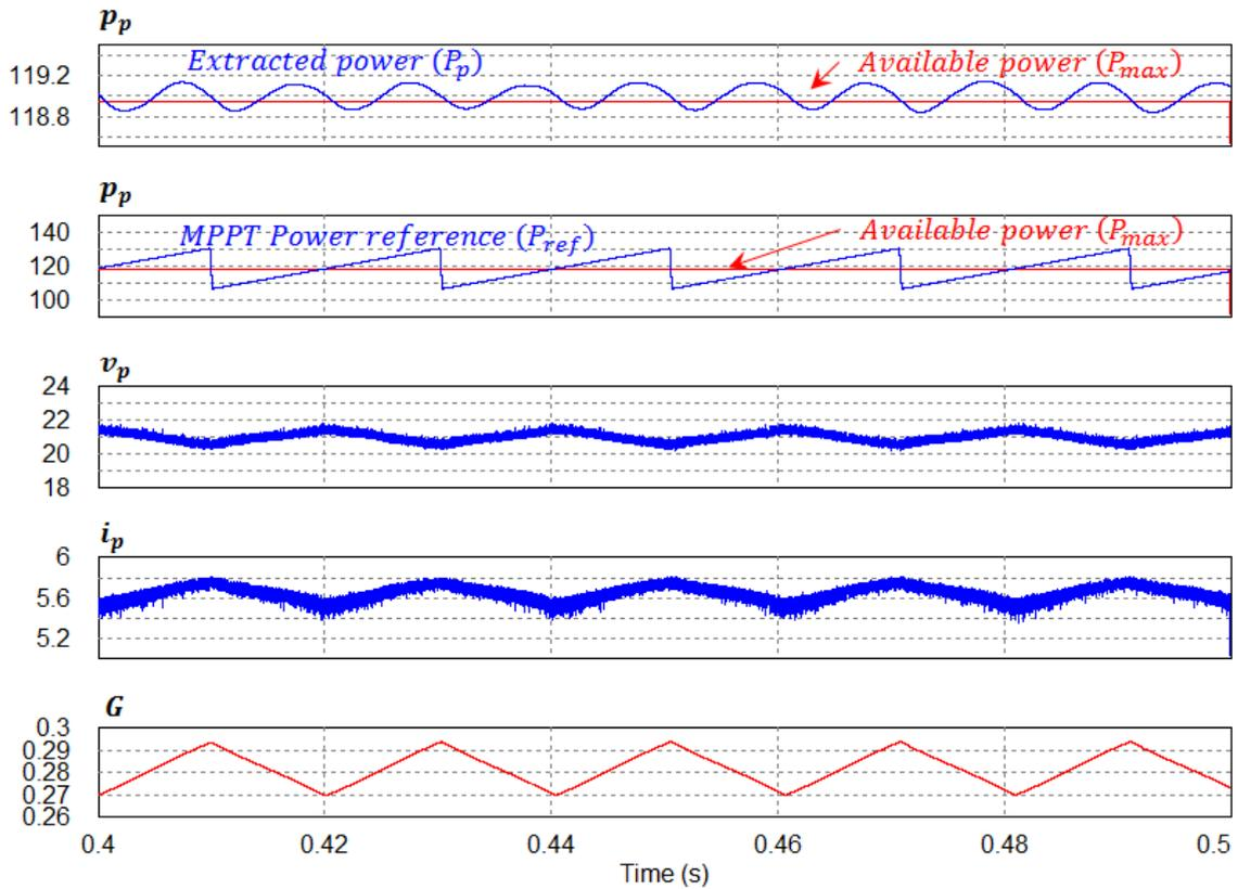
Fig. 5.13. Detail of the steady state of the current, voltage and power waveforms at the PV module side.
