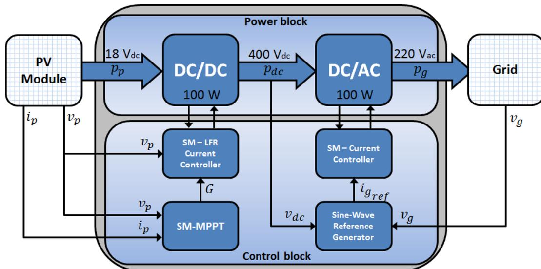
Fig. 1.4. General scheme of the sliding-mode controlled microinverter
