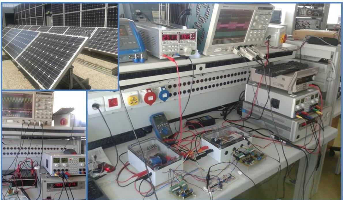
Fig. 5.16. Microinverter prototype and experimental set-up
