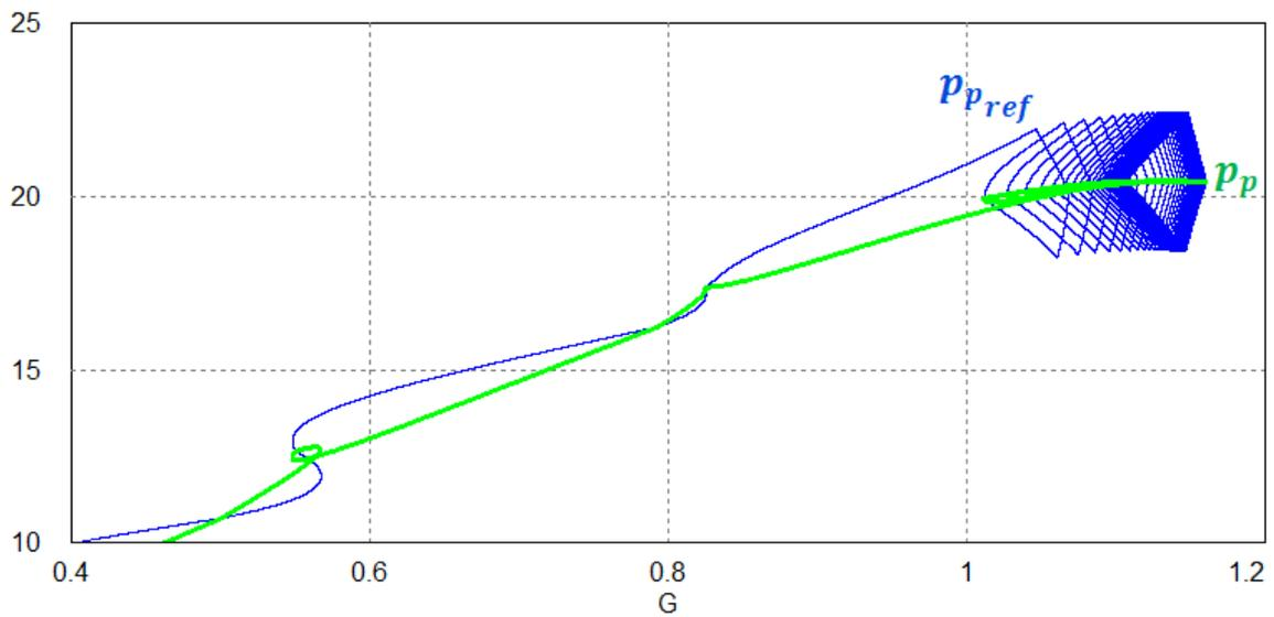
Fig. 2.18. Steady-state behavior of the proposed MPPT algorithm
