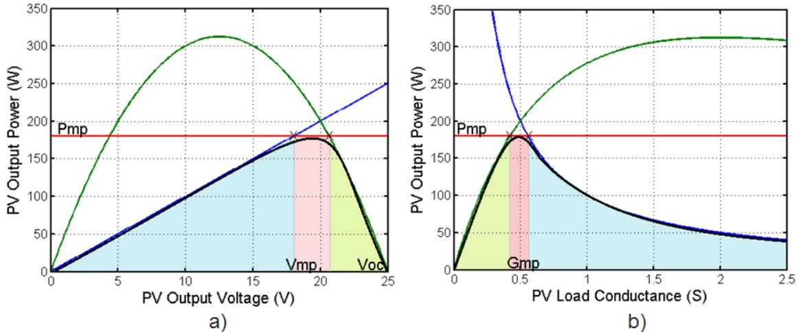
Fig. 2.2. Asymptotic approach of the characteristic curves of the PV module: a) P-V; b) P-G.
