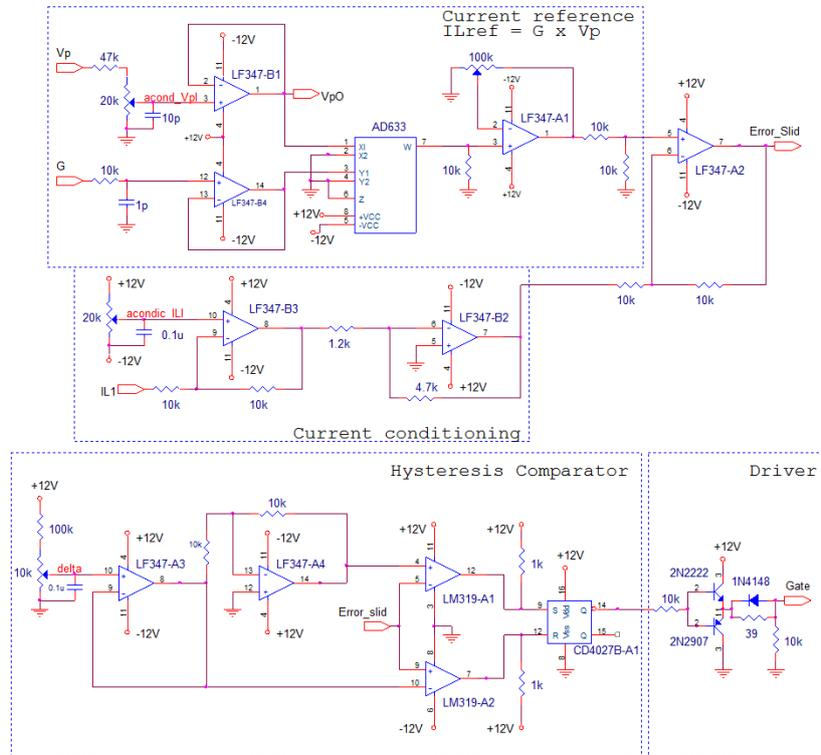
Fig. 3.26. Schematic circuit of the control board of the DC-DC converter
