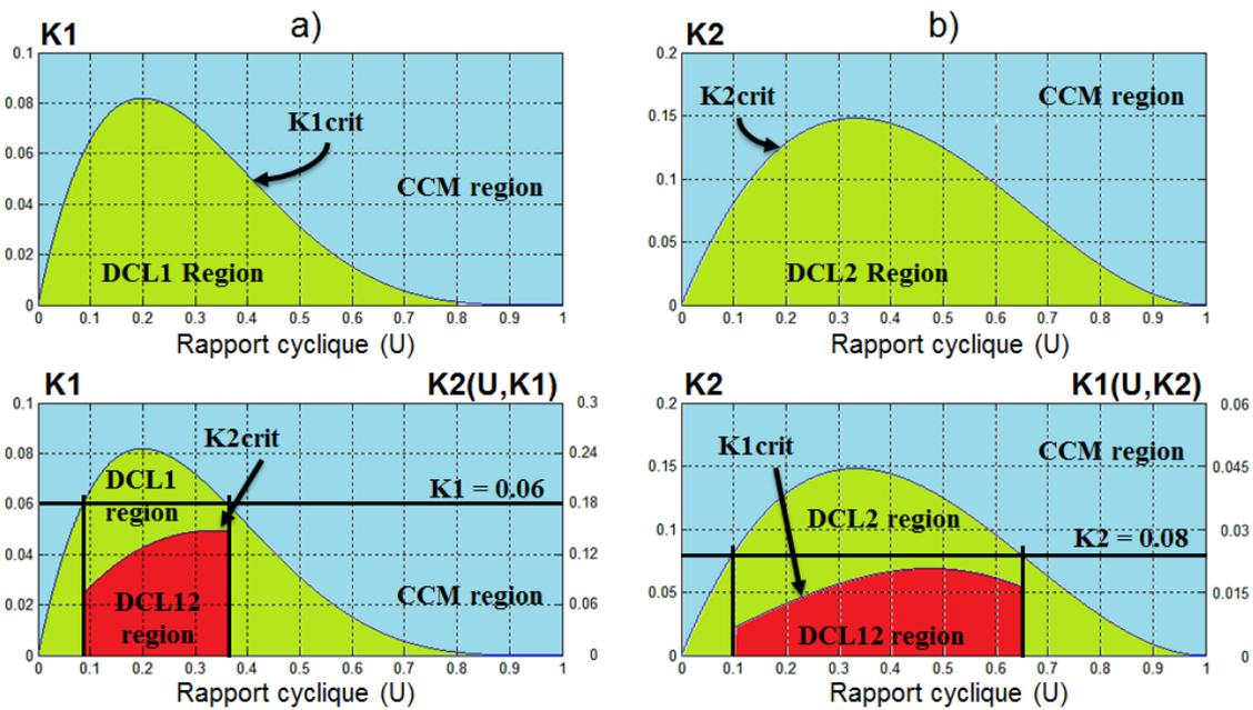
Fig. 3.8. Graphical representation of the critical values  $K_{1crit}$  and  $K_{2crit}$  as functions of the duty cycle  $U$ : a) CCM and DCL1 mode ( $K_1$  vs.  $U$ ), b) CCM and DCL2 mode ( $K_2$  vs.  $U$ ), c) CCM, DCL1 mode and DCL12 mode ( $K_2$  vs.  $U$ ,  $K_1$ ); d) CCM, DCL2 mode and DCL21 mode ( $K_1$  vs.  $U$ ,  $K_2$ ).
