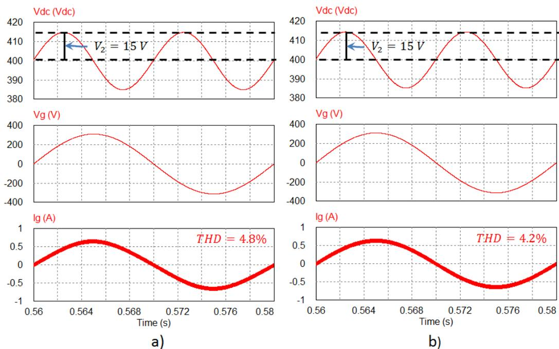
Fig. 4.18. Influence of the voltage ripple in the current harmonic distortion ( $L = 10 \text{ mH}$ ,  $C = 27 \text{ }\mu\text{F}$ ): a) case 1 ( $L = 100 \text{ mH}$ ,  $C = 27 \text{ }\mu\text{F}$ ); b) case 2 ( $L = 10 \text{ mH}$ ,  $C = 47 \text{ }\mu\text{F}$ ).
