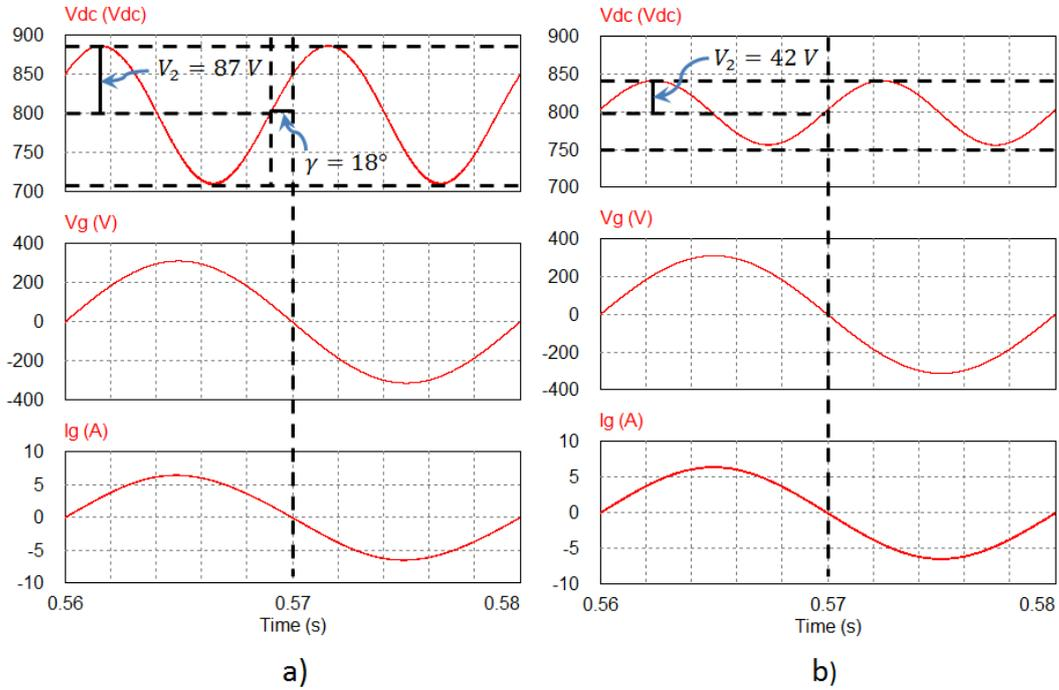
Fig. 4.12. Validation of the predicted parameters of the ripple in the voltage of the DC bus
