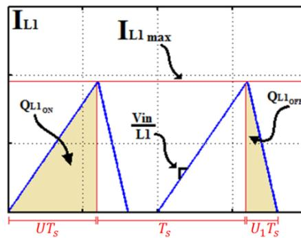
Fig. 3.5. Current waveform of the inductor L1 when the converter operates in DCL1 mode.
