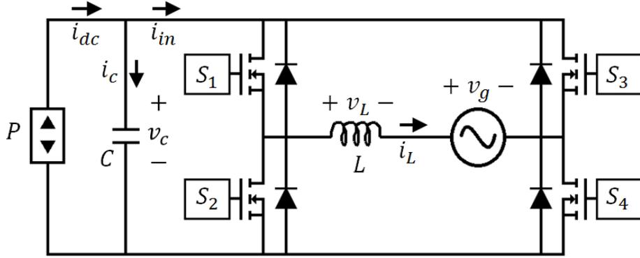
Fig. 4.19. Currents in the H-bridge grid-connected PSI.
