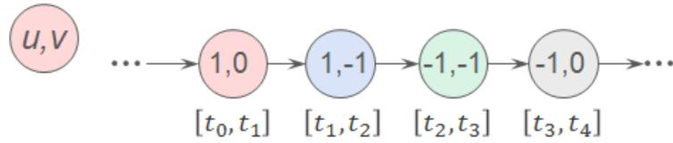
The trajectory induced by the repeated sequences in power characteristic is shown in figure 2.6. If  $P_{p_{ref}}(t_4) > P_{p_{ref}}(t_0)$ , after each sequence,  $P_{p_{ref}}(t)$  is growing up as shown in figure 2.6. Now, we will try to find the conditions under which the previous assertion is true.
