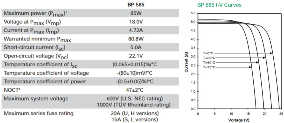
Fig. 5.17. Technical specification of the PV module BP585
