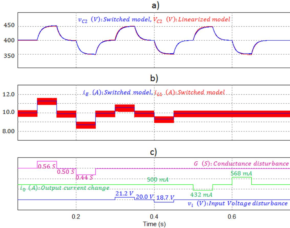
Fig. 3.19. Time response of the switching model compared with the linearized model when the converter operates with an input current controller (Parameters:  $L_1=120\ \mu\text{H}$ ,  $L_2=4.7\ \text{mH}$ ,  $C_1=C_2=11\ \mu\text{F}$ ): a) output voltage  $V_{C_2}(s)$ , b) input current compared with the input current reference, c) input waveforms  $G(s)$ ,  $V_i(s)$  and  $I_0(s)$ .
