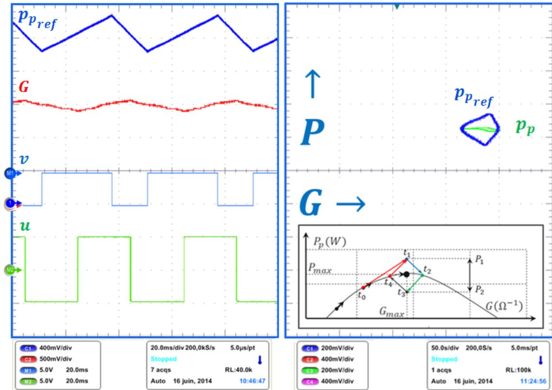
Fig. 2.32. Steady-state behavior of the proposed MPPT algorithm
