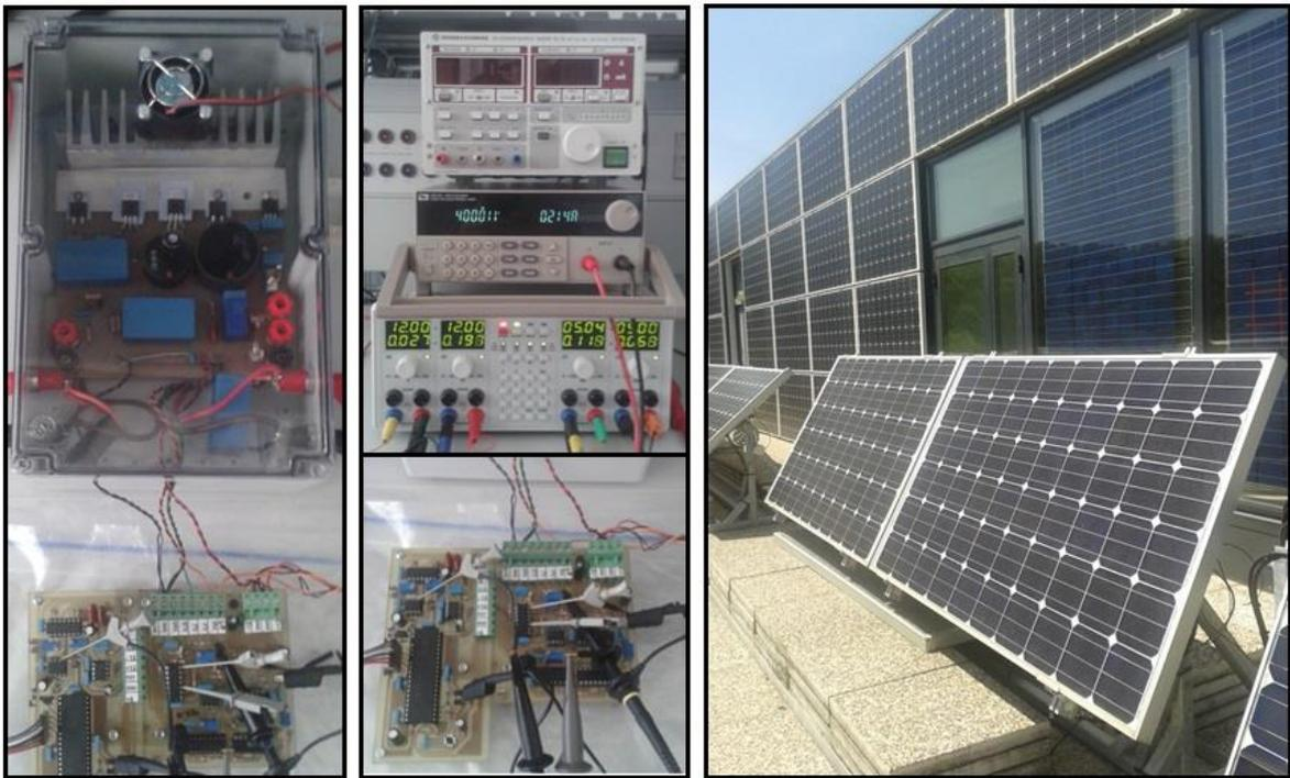
Fig. 2.28. Converter and MPPT prototypes ,and experimental set-up
