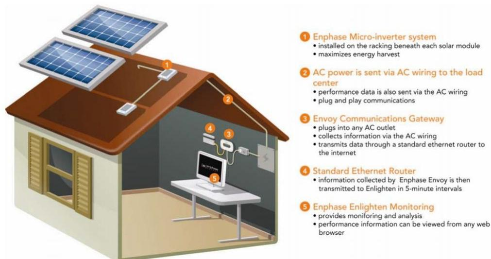
Fig. 1.2. Photovoltaic system based on “microinverters”. [Source: [www.enphase.com](http://www.enphase.com)]
