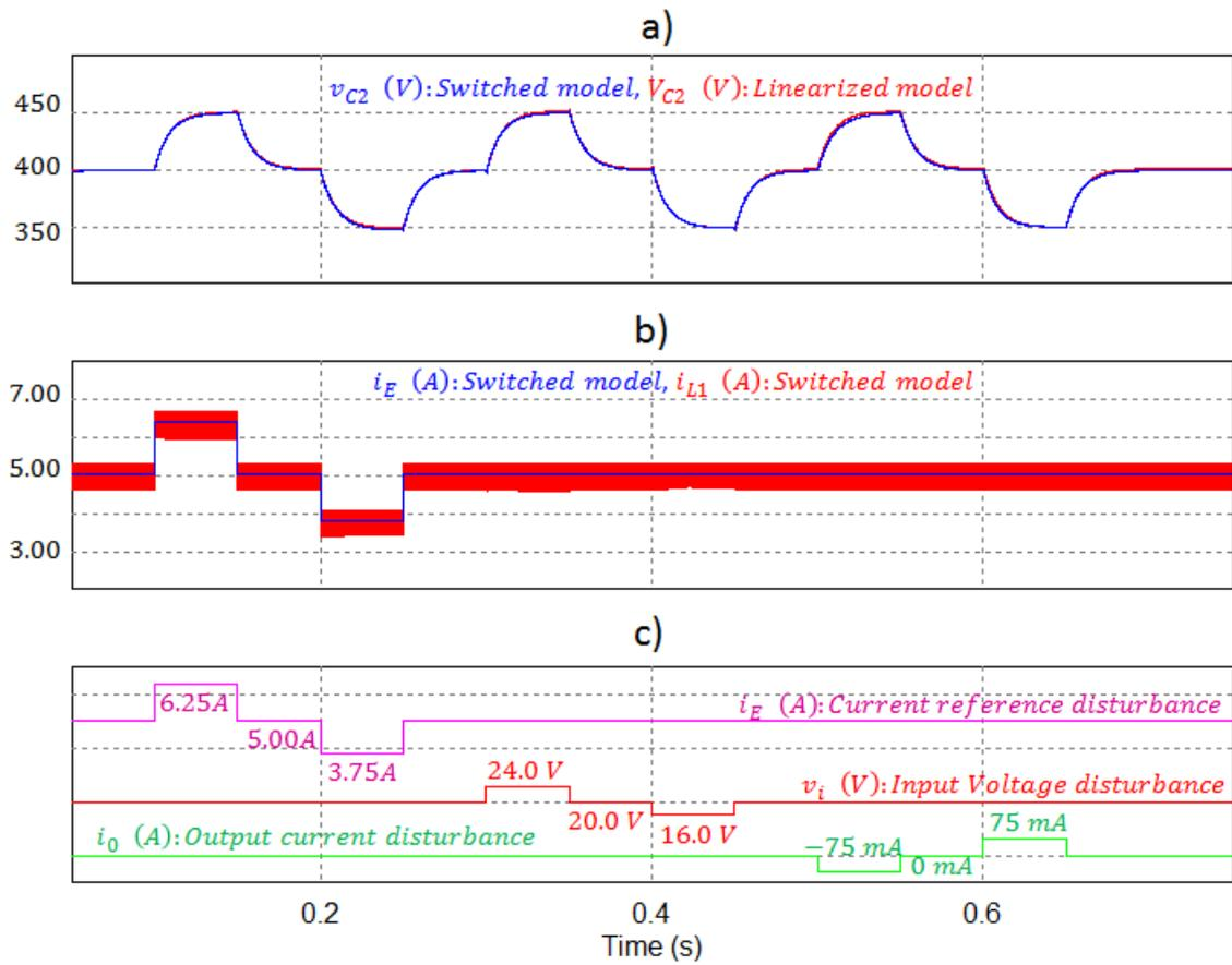
Fig. 3.14. Time response of the switching model compared with the linearized model when the converter operates with an input current controller (Parameters:  $L_1=120 \mu\text{H}$ ,  $L_2=4.7 \text{ mH}$ ,  $C_1=C_2=11 \mu\text{F}$ ,  $R=1600 \Omega$ ): a) output voltage  $V_{C2}(s)$ , b) input current compared with the input current reference, c) input waveforms  $I_E(s)$ ,  $V_i(s)$  and  $I_0(s)$ .
