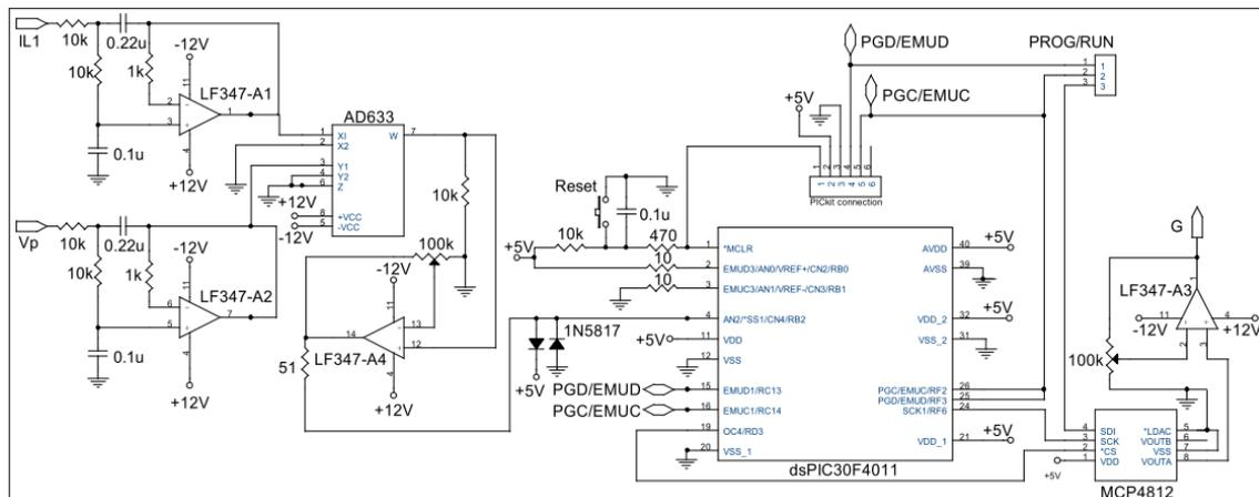
Fig. 2.27. Schematic electronic circuit for the MPPT algorithm
