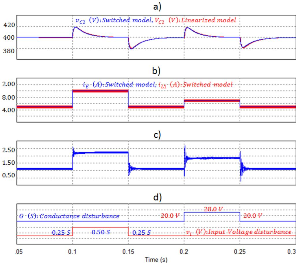
Fig. 3.20. Comparison of the switching model with the linearized model when the converter operates as a SM-LFR with output voltage regulation via output current (Parameters:  $L1=120 \mu\text{H}$ ,  $L2=4.7 \text{ mH}$ ,  $C1=C2=11 \mu\text{F}$ ,  $Kp=0.01$  and  $Ki=1$ ): a) output voltage  $v_{C2}(t)$ ; b) input current  $i_{L1}(t)$  and current reference  $i_E(t)$ ; c) current on inductor L2  $i_{L2}(t)$ ; and d) input disturbance waveforms  $G(s)$  and  $V_i(s)$ .
