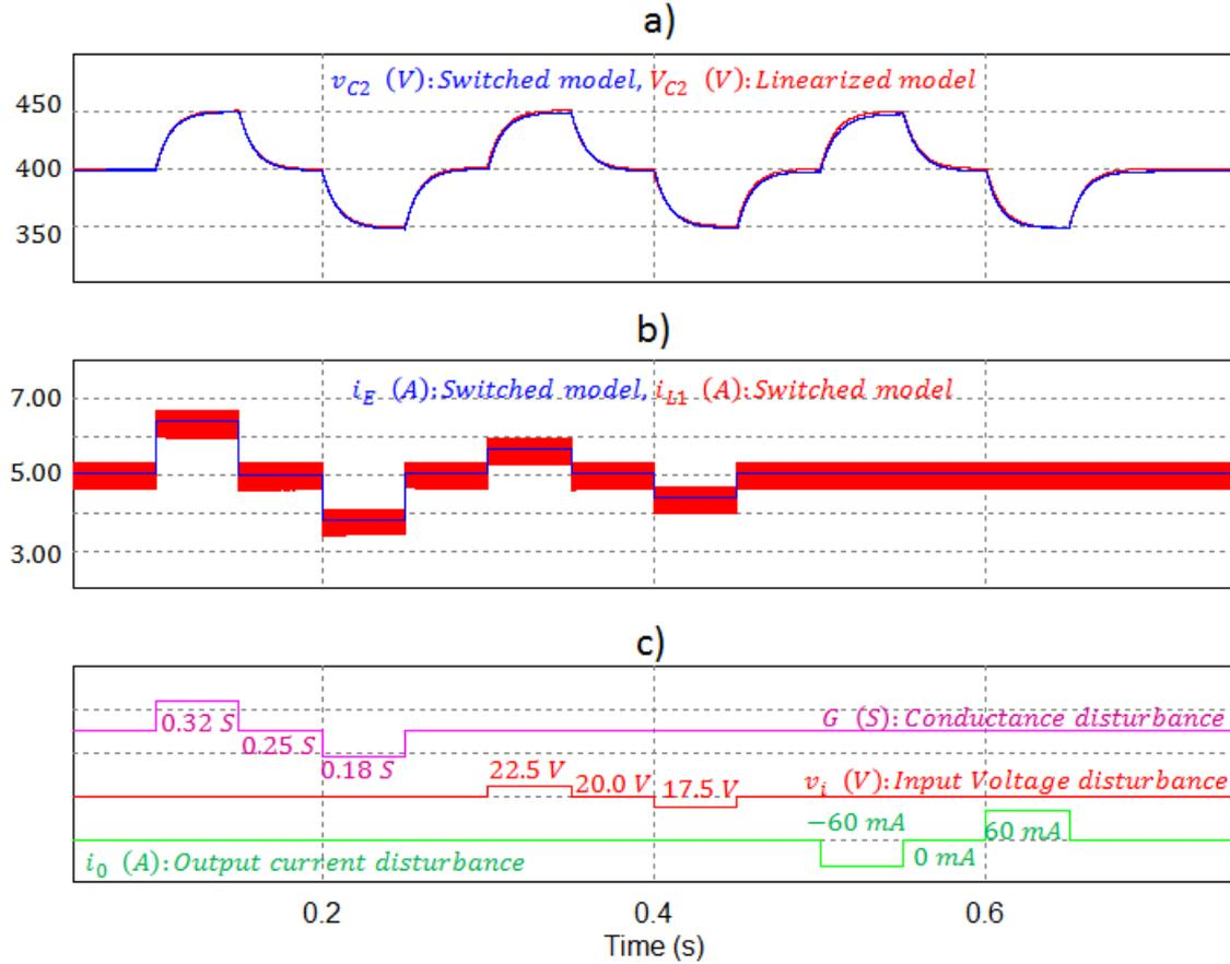
Fig. 3.18. Time response of the switching model compared with the linearized model when the converter operates with an input current controller (Parameters:  $L_1=120 \mu\text{H}$ ,  $L_2=4.7 \text{ mH}$ ,  $C_1=C_2=11 \mu\text{F}$ ,  $R=1600 \Omega$ ): a) output voltage  $V_{C2}(s)$ , b) input current compared with the input current reference, c) input waveforms  $G(s)$ ,  $V_i(s)$  and  $I_0(s)$ .
