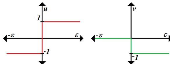
Fig. 2.4. Ideal switching functions of the proposed sliding-mode MPPT.
