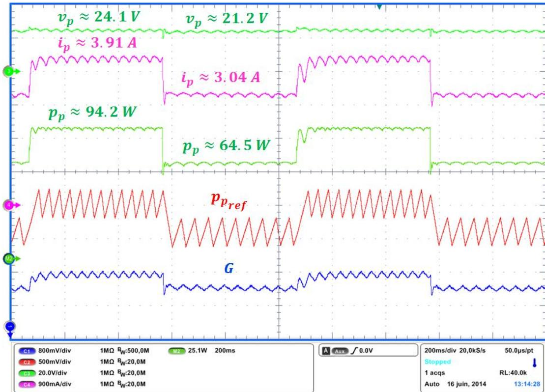
Fig. 2.38. Experimental results for 30 W sudden changes in the P-V characteristic curve.
