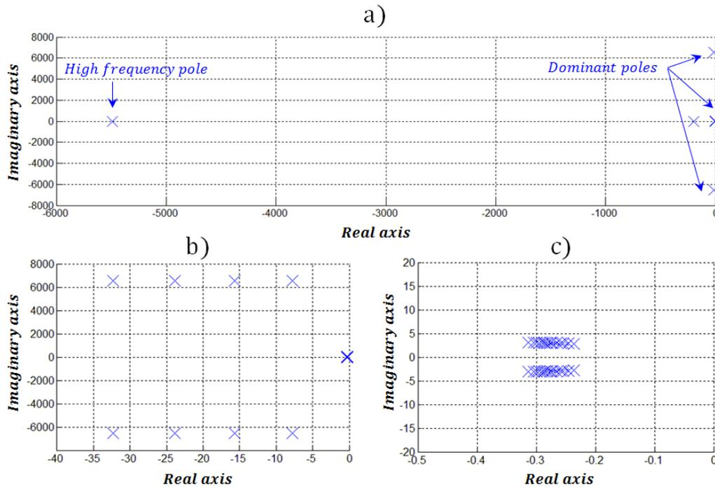
Fig. 5.4. Roots of the closed- loop system in the complex plane for different equilibrium points.
