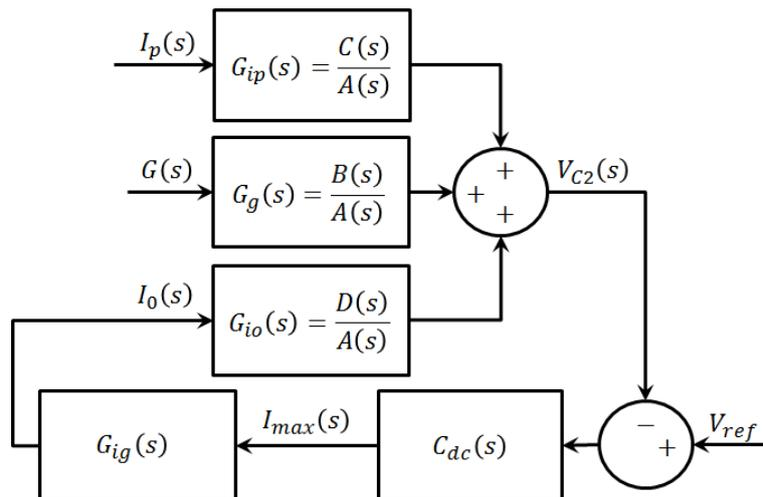
Fig. 5.2. Block diagram of the linear approach coupling the DC-DC stage and the DC-AC stage
