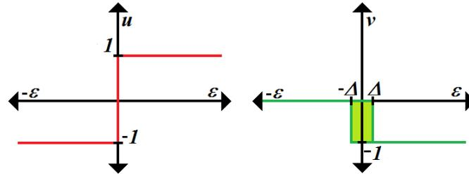
Fig. 2.5. Switching functions of the proposed sliding-mode MPPT.
