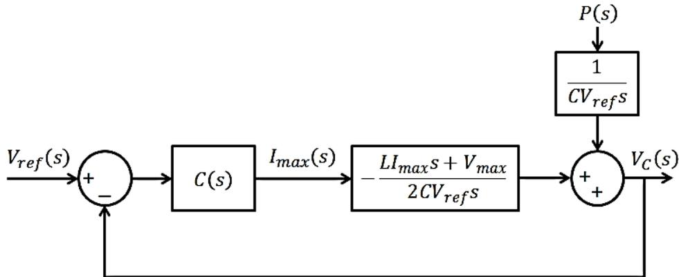
Fig. 4.5. Block diagram of the closed-loop control system.
