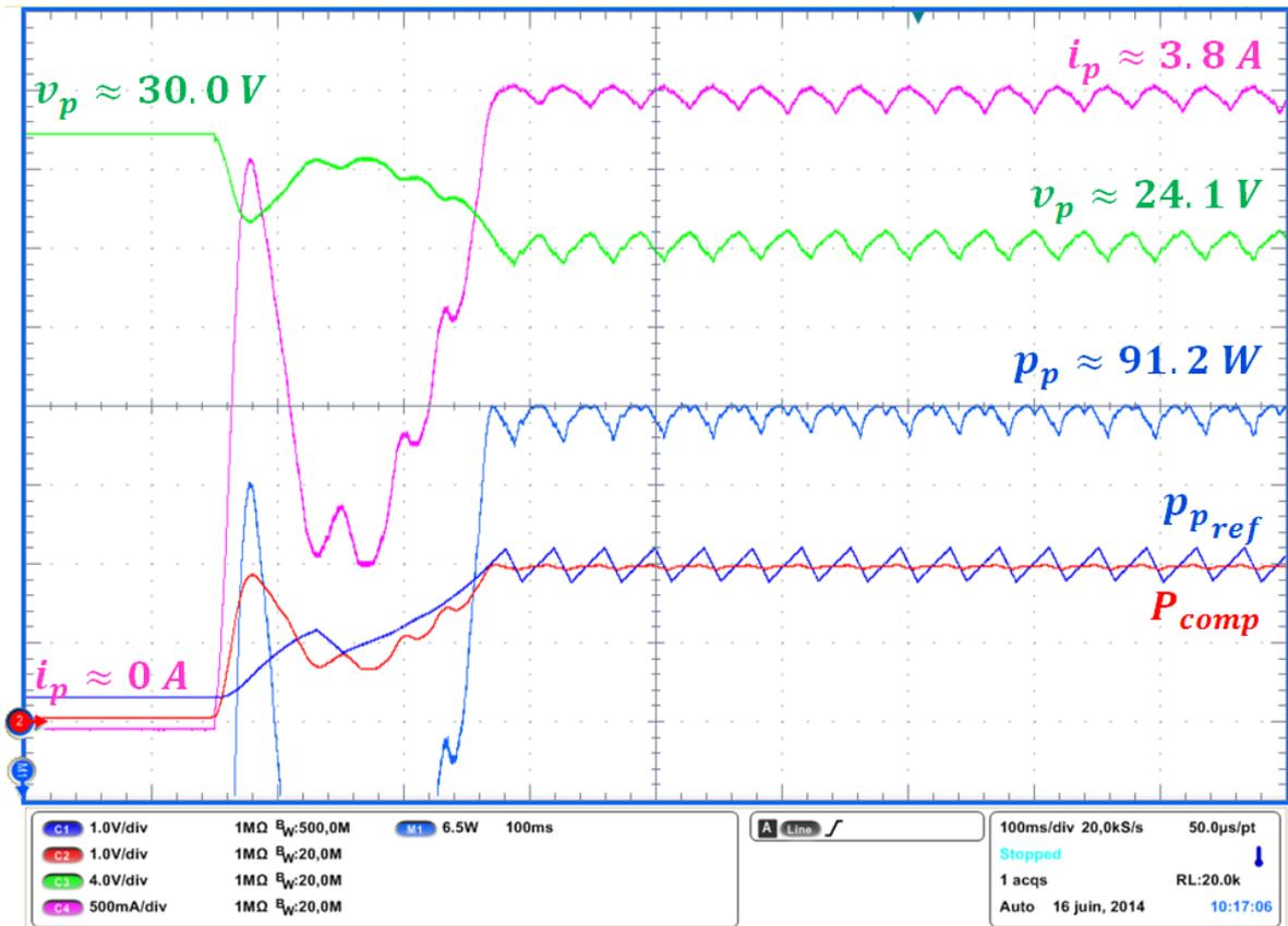
Fig. 2.36. Time response of the voltage, current and power of the system during a start-up
