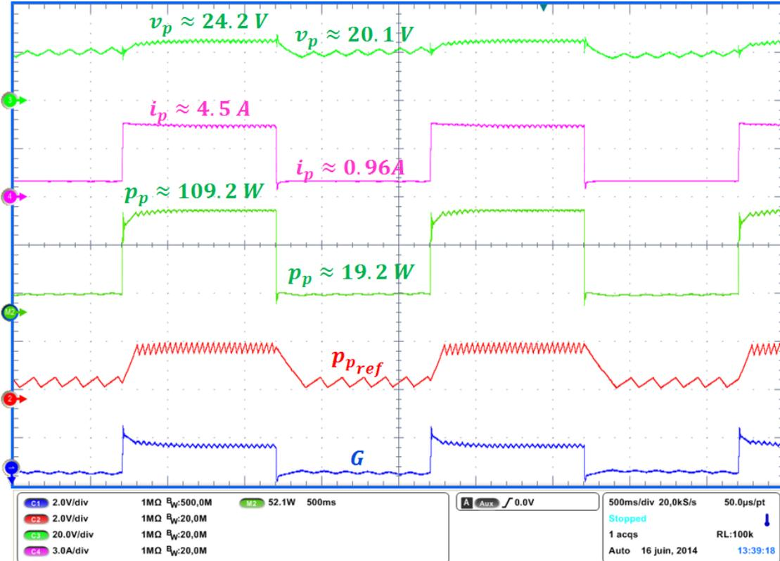
Fig. 2.39. Experimental results for 80 W sudden changes in the P-V characteristic curve.
