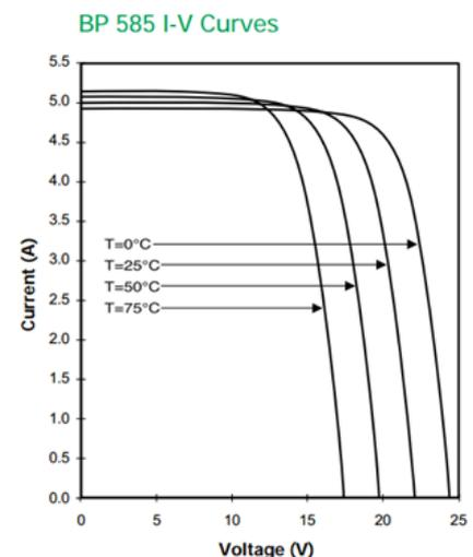
Fig. 2.29. Technical specifications of the PV module BP585
