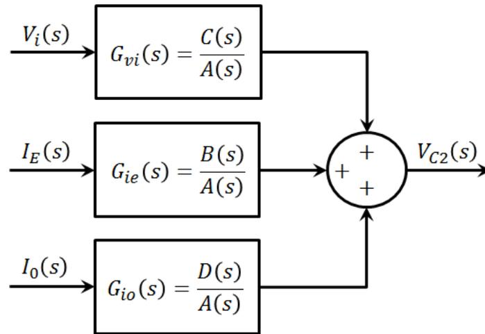
Fig. 3.13. Block diagram of the linearized model
