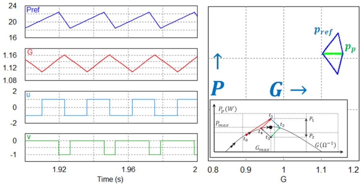
Fig. 2.19. Steady-state behavior of the proposed MPPT algorithm
