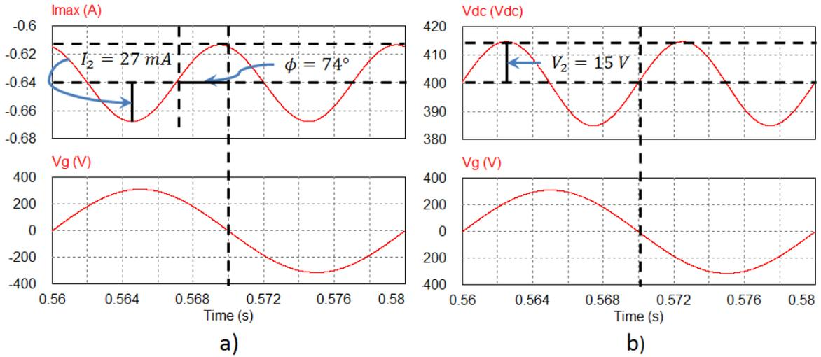
Fig. 4.13. Validation of the predicted parameters of the current amplitude  $i_{max}$  ( $L = 10\text{mH}$ ,  $C = 47 \mu\text{F}$ ).
