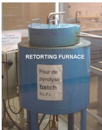
Figure 2.2: Retorting Furnace for LHR-char preparation (RF)
