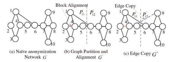
Figure 2.4: Graph partition and edge copy: edge between nodes 2 and 4 and crossing edge between 5 and 9 are added in the anonymized graph.
