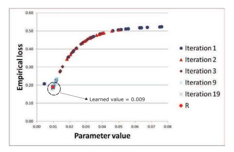
Figure 5.7: EDA behavior with one parameter (n = 1). At the first step of the algorithm the population is initialized to a uniform distribution over admissible solutions. After 19 iterations the learned value is close to the optimum one.
