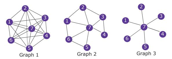
Figure 5.2: Example for local clustering coefficient: three graphs used to illustrate how the clustering coefficient is computed.
