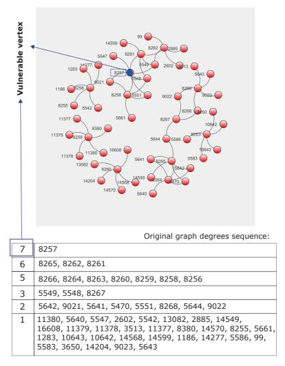
Figure 5.3: Baseline: original graph and the corresponding vertices degree hashtable; node 8257 is the most vulnerable in the graph according to its degree.
