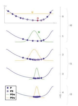
Figure 4.3: Estimation of distribution algorithm: for each step candidates solutions are generated. At step 0, population is initialized from a uniform distribution over admissible solutions (P). The most promising candidates (PS) are selected and a new population is generated at each step following a normal distribution N with the distribution parameters PDe.
