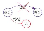
Figure 6.5: Replace right operation: destination vertex of the edge is replaced by a random vertex.
