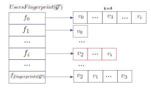
Figure 6.11: Hashtable containing as key the fingerprints and as value the list of the vertices characterized by the corresponding fingerprint in  $\mathcal{G}'$ .
