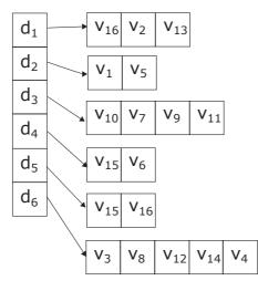
Figure 5.1: Vertices degree hashtable: it stores for each degree  $d_i$  present in the graph the corresponding list of vertices of degree  $d_i$ .
