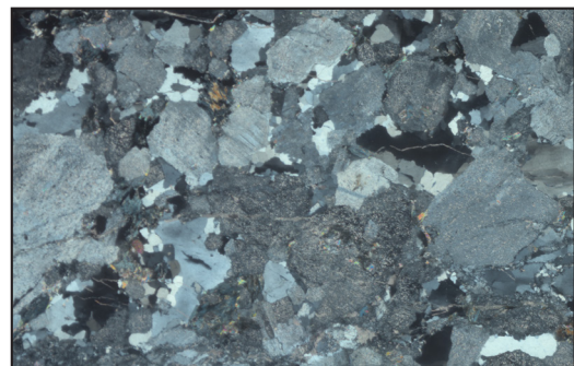
Figure A3. Mineralogical study of fault rocks from extensional detachment. Mineralogical recognition was done using optical microscopy and XRD of bulk rock and clay fraction (<2 micrometers). The sample is the Albula granite outside the fault zone of the Err detachment. It is little affected by fluid-rock interactions.
