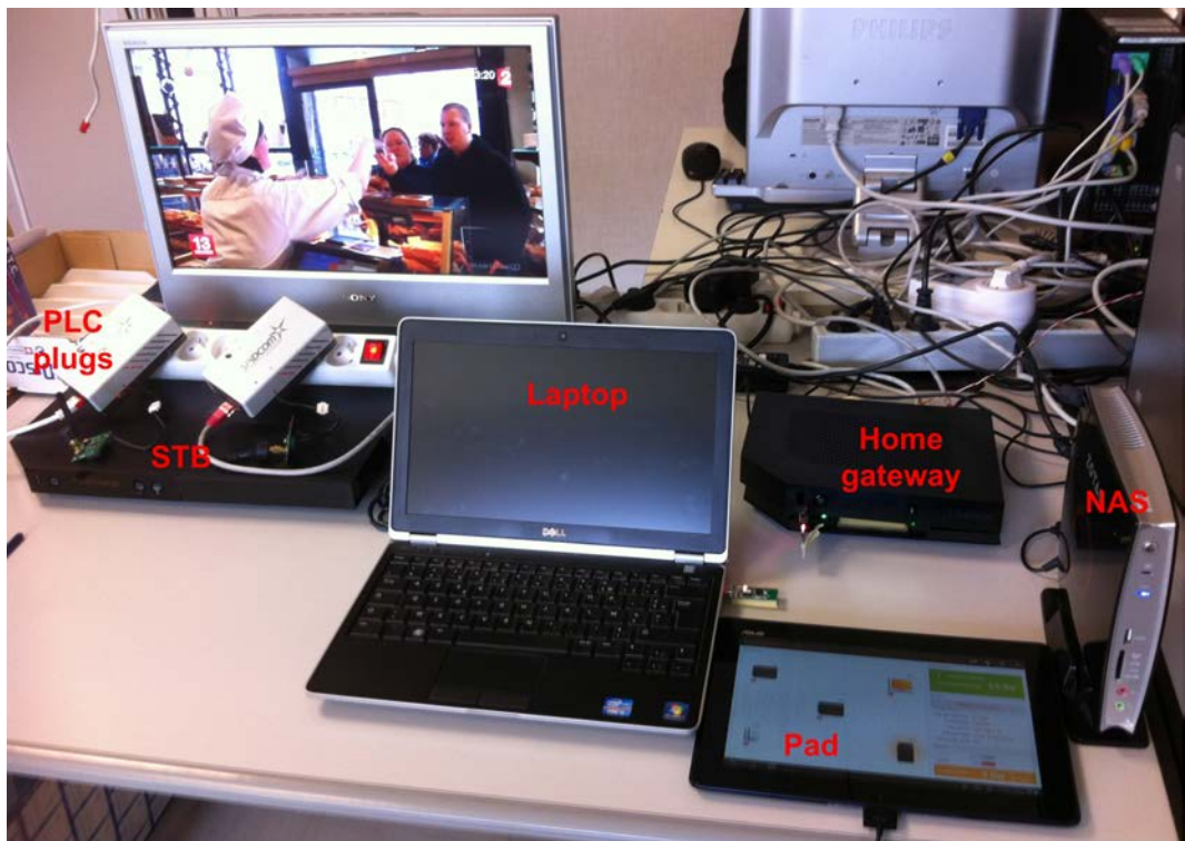
Figure 5.7: The testbed of the H0me Power Energy system
