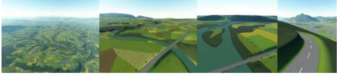
Figure 2.1: Real-time rendering of terrains using quadtrees [BN08], where the terrain’s level of detail is automatically adapted to the camera position. The terrain is subdivided in square cells of various sizes, depending on their distance to the camera, and the color texture and heightfield are computed independently for each cell. When the camera moves, the structure is updated (i.e., cells are merged or subdivided) and their textures recomputed. This method enables real-time rendering of very large terrains, even planets.
