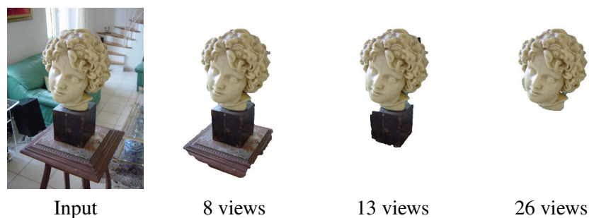
FIGURE 5.9: Results on BUSTE dataset with different numbers of views. For the 8 views result, the table is seen by all the views. With 13 views some cameras eliminate parts of the table and it is thus classified as background. Finally with all the views, the black elements in the background appear close and similar to the black pedestal. Thus, only the head is identified as foreground in this case.
