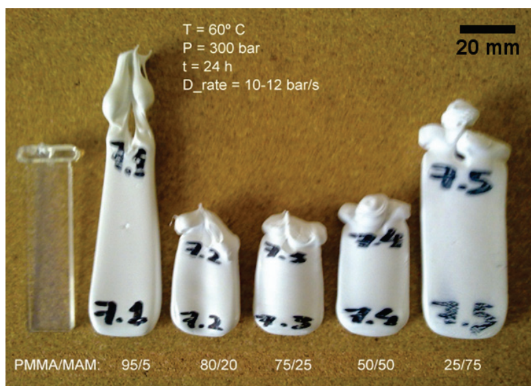
Figure II.21: Macroscopic shape of foams produced at 30 MPa and 60° C from different PMMA/MAM blends compared to the solid precursors shape and dimensions (left). The saturation time was 24 hours and the depressurization rate was around 30 MPa/min.
