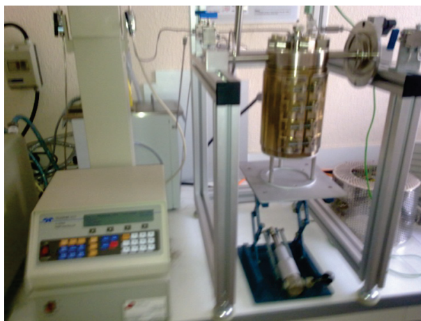
Figure II.19: Teledyne ISCO pressure pump (left), and TOP Industrie high pressure vessel (right).
