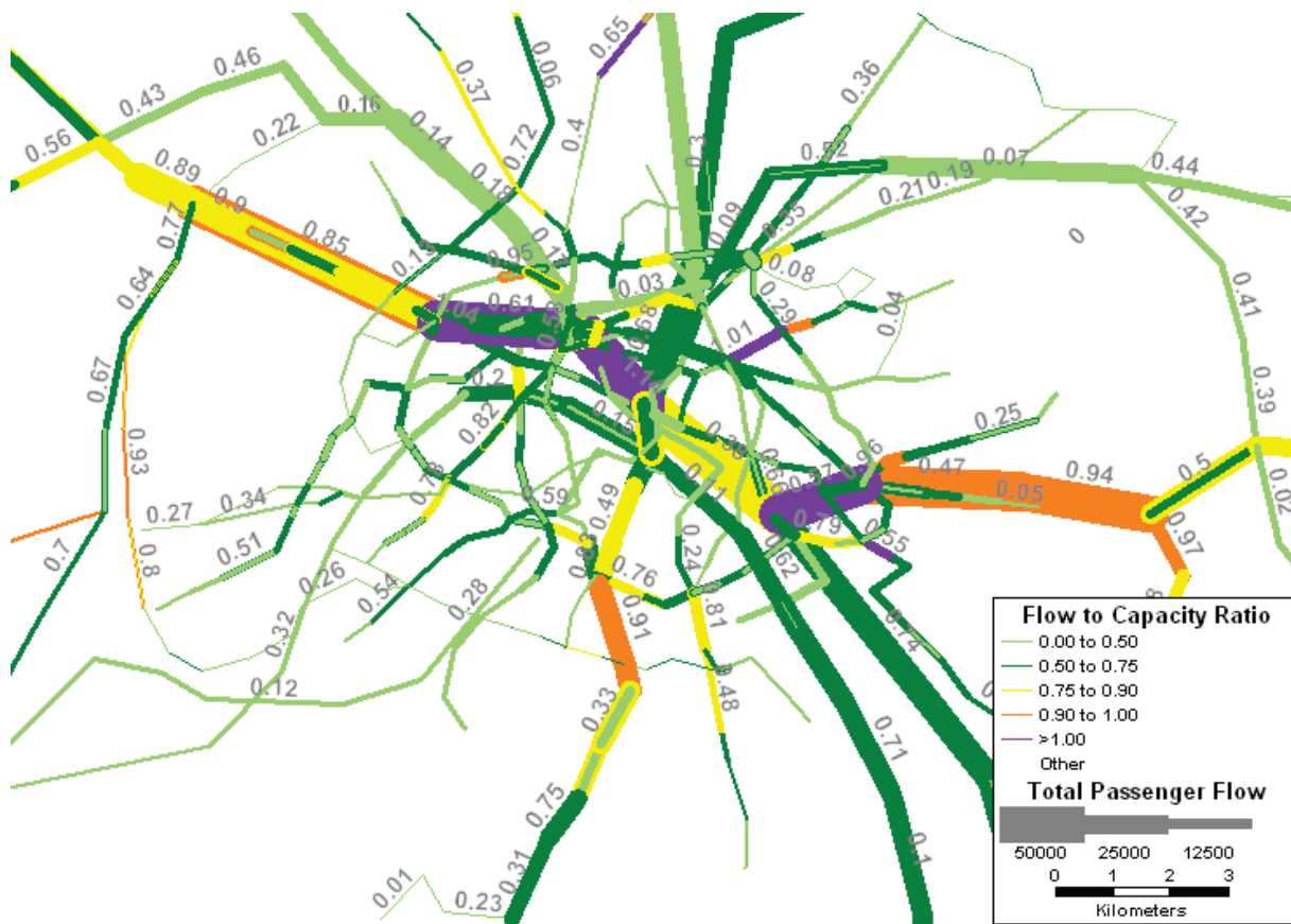
Figure 38: Passenger flows and the ratio of flow to operative capacity for the bounded model
