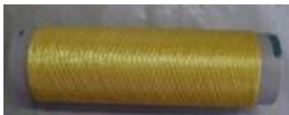
Figure V-5 Curative Fibre spool, provided by Cytec
