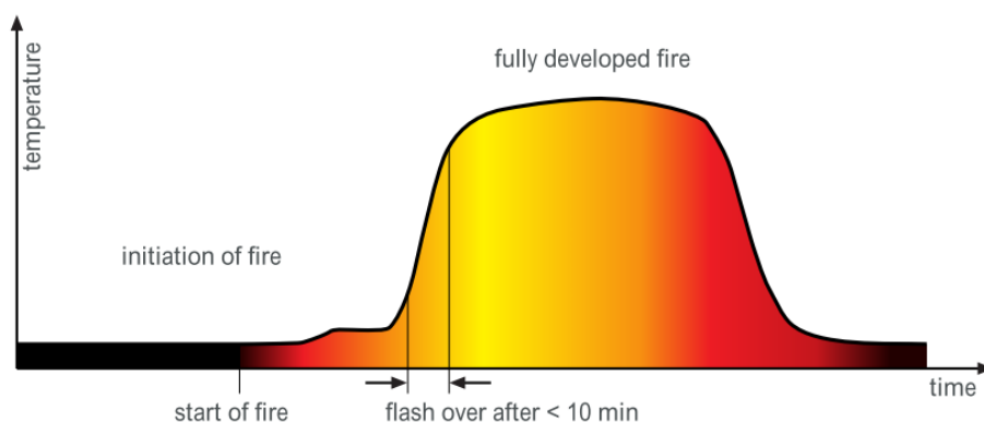
Figure I-1 Fire scenario as observed from its temperature profile [3]
