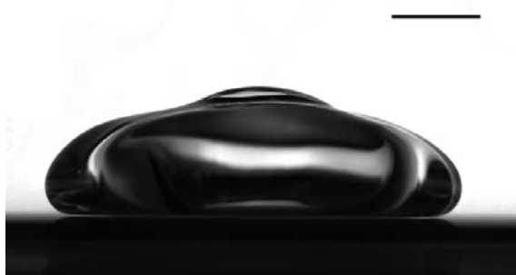
Figure I.20 – Side view of a Leidenfrost drop puddle deformed by a chimney instability. Vapor underneath is less dense than liquid on top. As the interface is deformable, buoyancy effects make the vapor try to escape upwards and form a dome before bursting. Scale shows 5 mm.
