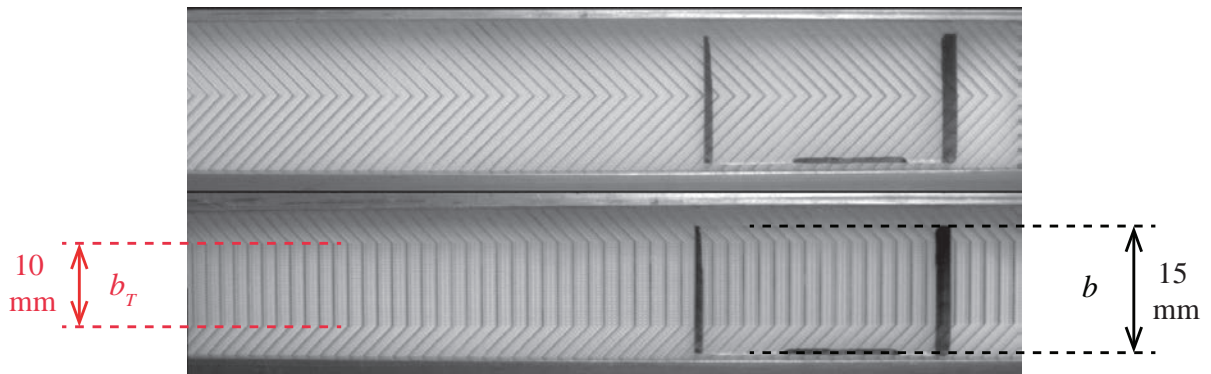
Figure III.9 – Comparison between two textures entraining a glass slider of length a = 30 mm, width b = 15 mm and thickness c = 1 mm (resulting in a weight M around 1 mg). Top texture is the “classical” herringbone. Bottom one corresponds to the “truncated” herringbone, which has a central straight section of length b_T (fixed to 10 mm) perpendicular to motion, hence having a null viscous propelling contribution.
