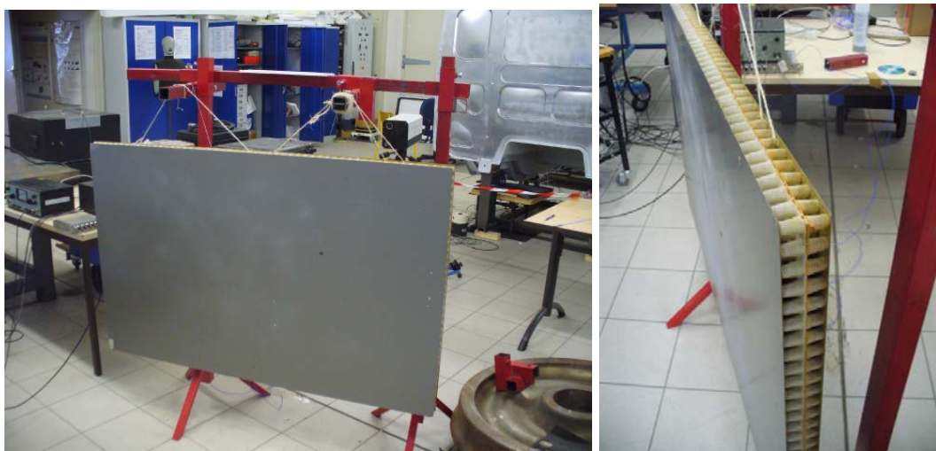
Figure 4.17: Double-faced thick composite panel represents a structure with complex behaviour at higher frequencies.
