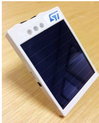
Figure 2.3: GREENNET node with its photovoltaic cell and control LEDs
