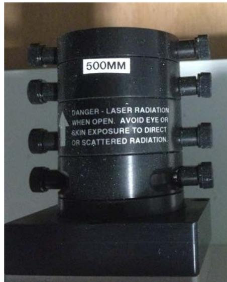
Figure 2.15 – The lenses to expand the laser beam to a sheet
