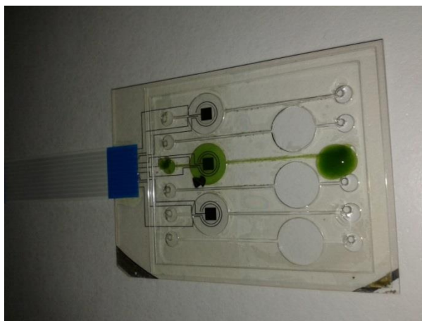
Figure 5.6. Algal test solution inserted in one of the chambers of the lab-on-chip device.
