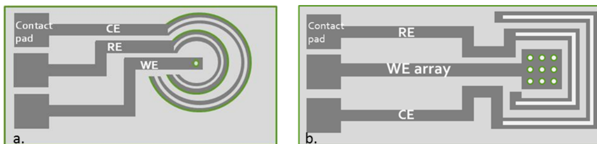
Figure 3.1. Schematic representation of concentric configurations tested: a) single microelectrode b) UME array.
