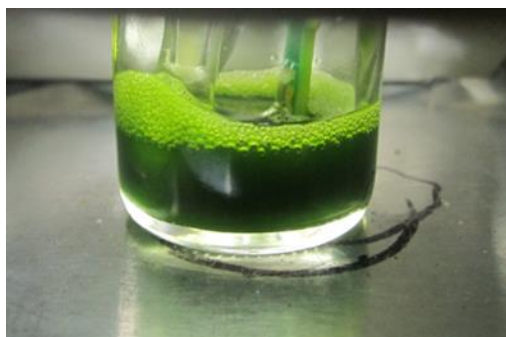
Figure 5.2. Silicon-based oxygen sensor in algal solution.
