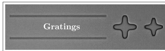
FIGURE 4.31: Optical image of the epi-wafer after the definition of gratings
