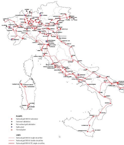
Figure 5:1 The 380kV Italian Power Transmission Network (IPTN380) (Zio and Sansavini, 2011a).
