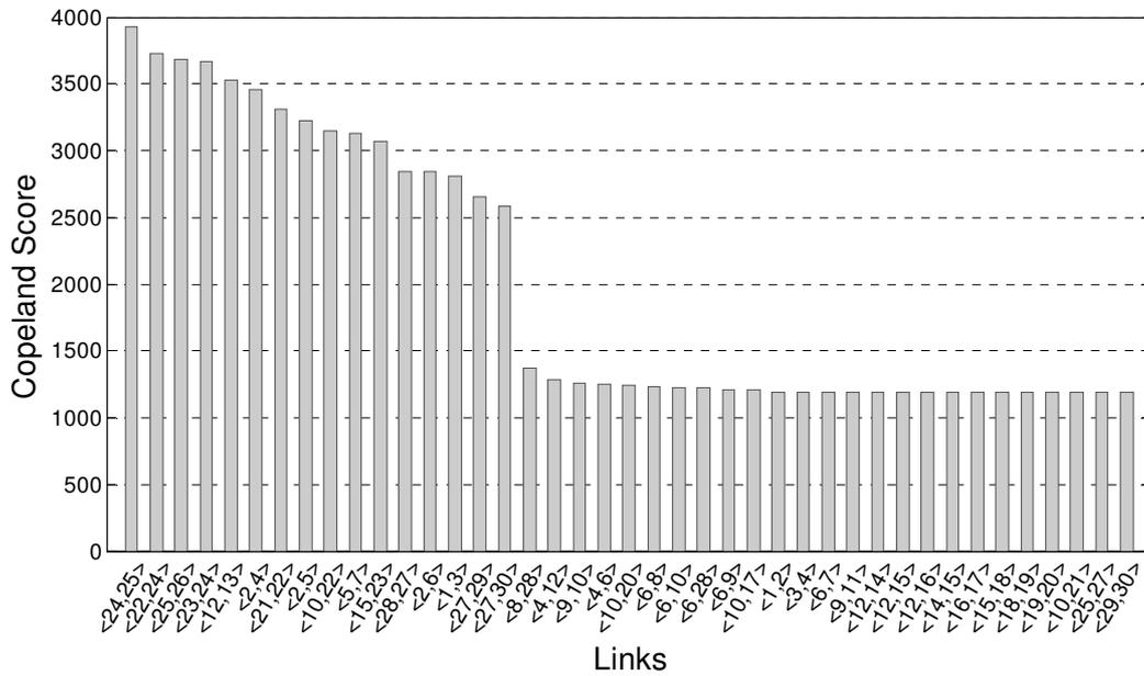
Fig. 8. Copeland score ranking of the resilience reduction worth  $RRW_{ij}(\Delta t_0 = 3)$  for all IEEE 30 Bus network links.
