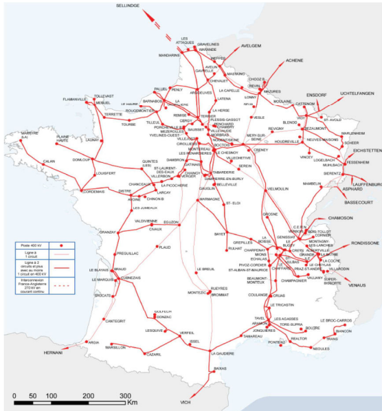
Fig. 1. The 400kV French power transmission network (FPTN400) [37].
