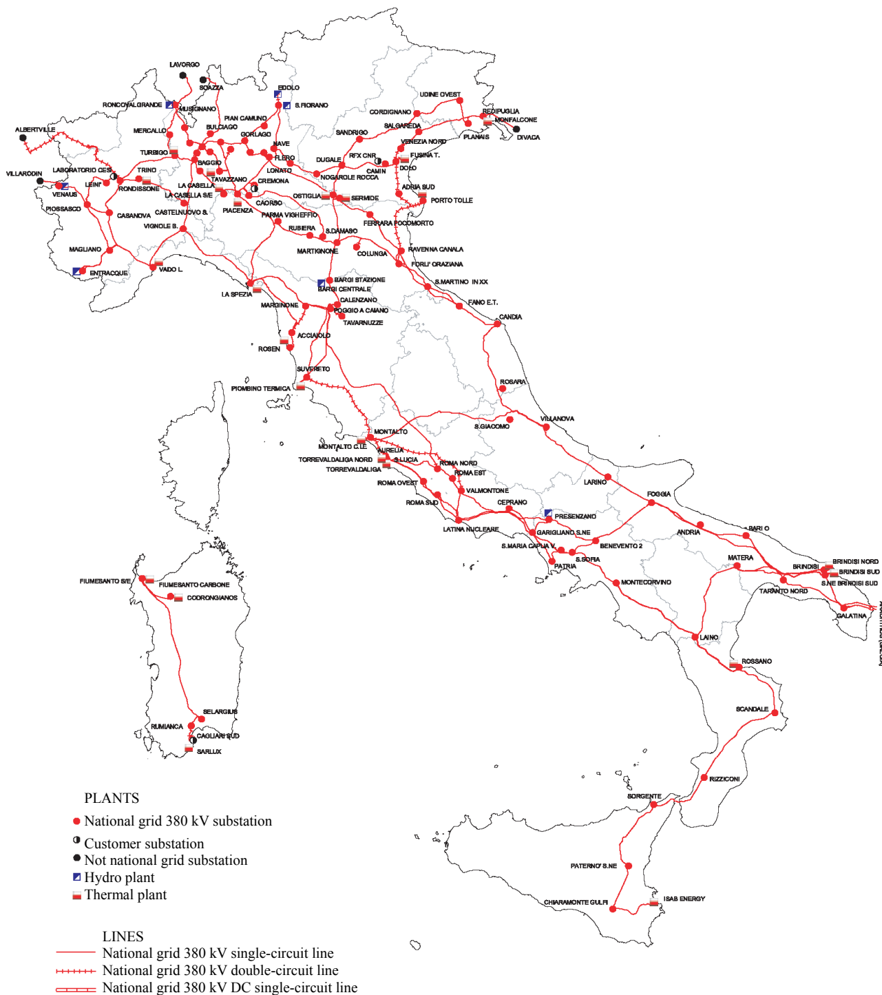
Figure 1. The 380 kV Italian power transmission network.
