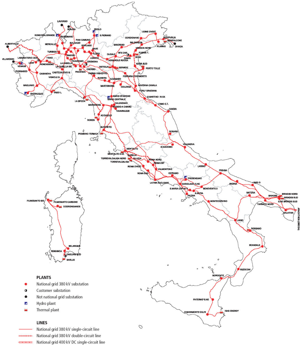
Fig. 1. The 380 kV Italian power transmission network.
