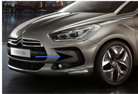
(a) Passive blowing to lower drag induced by the wheels
