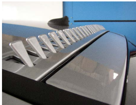
(b) Active vortex generators on the concept Citroën C-Airlounge
