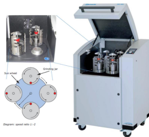
Fig.2.2. Planetary ball mill-Retsch PM 400 (taken from Retsch web page).
