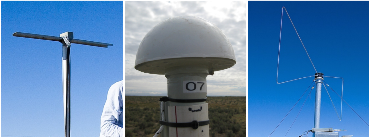
Figure 5.3 Left: fat dipole antenna installed in the hexagon in 2011 for MHz measurements. Middle: feed horn LNBF GI-301SC antenna installed (7 in 2011 and 54 more in 2012) for the GHz measurements. Right: one of the butterfly antennae installed in 2013 for MHz measurements.
