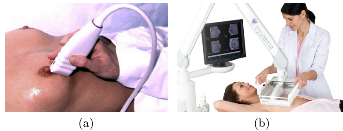
Figure 1.5: Conventional hand-held US and ABUS acquisition devices comparison. (a) Conventional hand-held US imaging acquisition device. (b) ABUS acquisition device.
