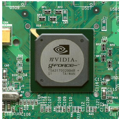
leading to the term GPGPU (General Purpose Graphics Processing Unit). GPGPU is considered as a modified form of stream processor. This concept turns the massive computational power of a modern graphics accelerator's shader pipeline into a general-purpose computing power. In some applications requiring massive vector operations, this can yield several orders of magnitude higher performance than a conventional CPU.
