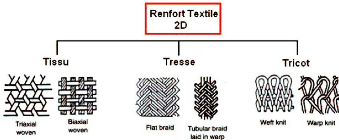
Figure 1-4. Classification des principales structures textiles 2D [27].
