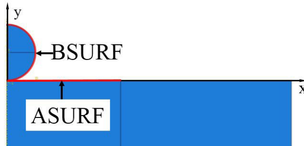
Figure 2.3: Schematic diagram of surface-to-surface contact.
