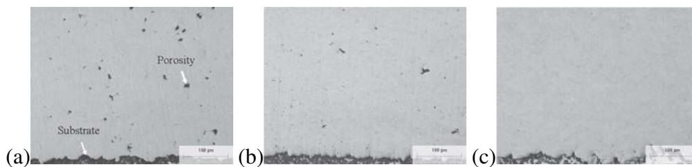
Figure 1.13: Porosity formation in cold sprayed microstructure for gas temperatures of (a) 300 °C, (b) 420 °C and (c) 630 °C [ZAH 06].
