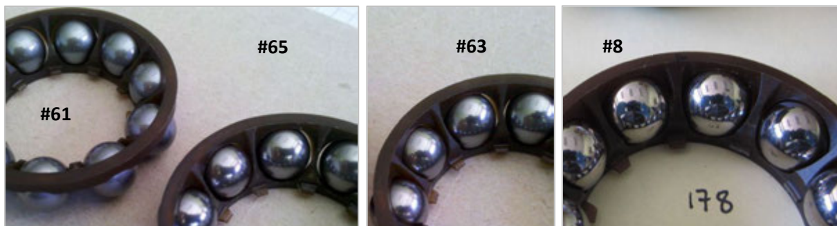
Fig. 4.5: WEC-affected ACBB #61 balls with a matt grey coloration; WEC-free ACBB #65 and #63 balls with a shiny aspect; WEC-affected ACBB #8 balls with also a shiny aspect.
