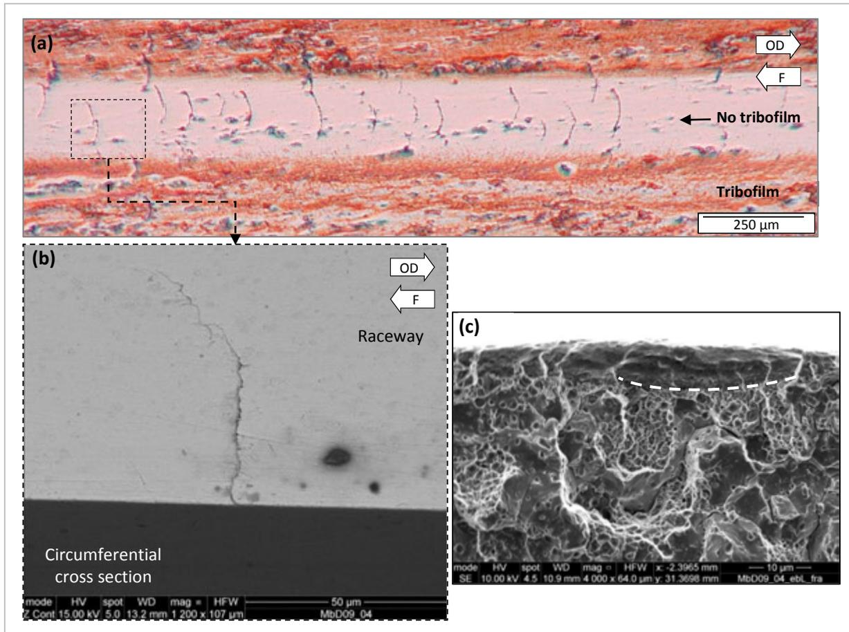
**Fig. 5.12:** TDM09\_04 crowned roller typical raceway center topview (a), SEM  $\frac{3}{4}$  view of a circumferential cross section (b), and SEM analysis of a raceway fractographs opening a shallow surface microcrack (initiation phase;  $1.9 \times 10^7$  cycles, 2 GPa, 7% SRR, follower, lubricant A at 50°C).
