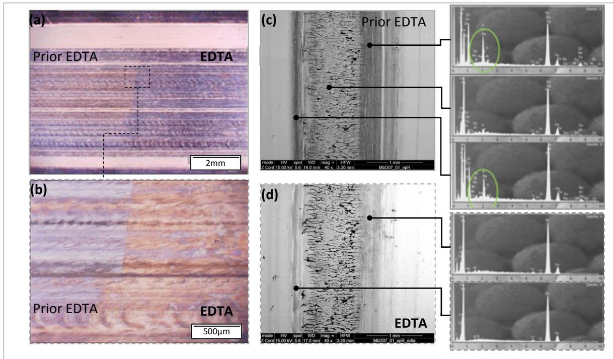
**Fig. 2.18:** Efficiency of EDTA to remove tribofilm deposits (1) illustrated by the clear frontier between the untouched left side and the EDTA tissue-cleaned right side of a TDM raceway observed on (a) side-angled LOM and (b) co-axial LOM close-up (Appendix H ref TDM12\_07) and (2) confirmed by SEM-EDX analysis on a different TDM raceway (Appendix H ref TDM07\_01\_II) (c) prior and (d) after EDTA ultrasound bath rising where no more traces of sulfur and phosphorus remain.
