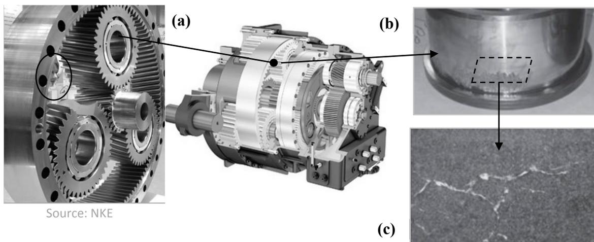
**Figure 8:** (a) Multi-MW wind turbine gearbox layout and size compared to a human head; (b) Example of wind turbine REB fatigue failure [7] associated to (c) the formation of White Etching Cracks (WEC) [7].
