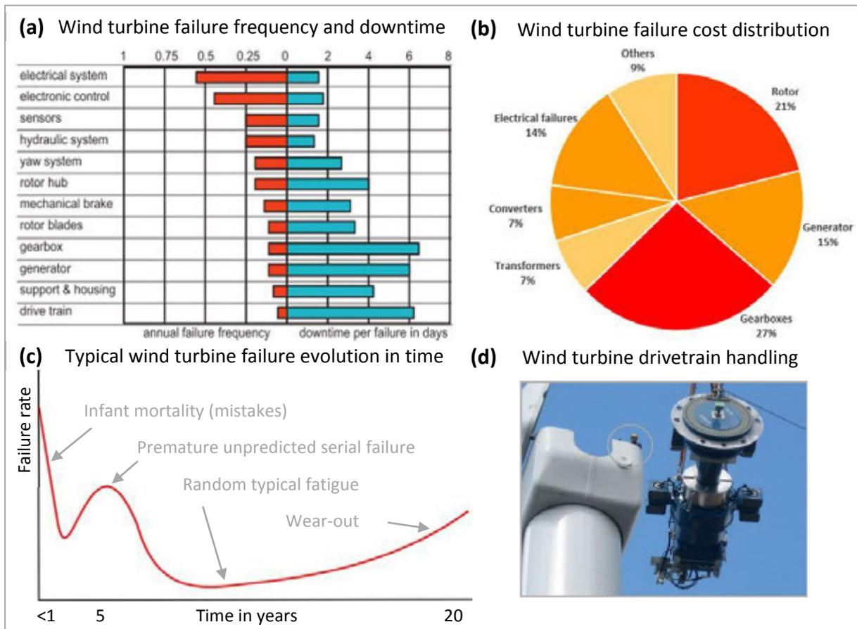
**Figure 7:** (a) (b) Wind turbine failures distribution in 2009 and the impact on the O&M costs [5]; (c) typical wind turbine failure rate evolution in time with premature failures; (d) wind turbine drivetrain handling.
