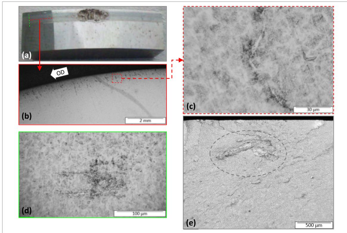
**Fig. 3.5:** WEC reproduction on the artificial H-precharged TDM roller of TDM08\_01: (a) premature spall, (b) circumferential LOM revealing WEC, (c) close-up on a WEC in the depth of maximum shear stress, (d) axial LOM revealing WEC; (e) axial fractograph revealing a brighter WEC network.
