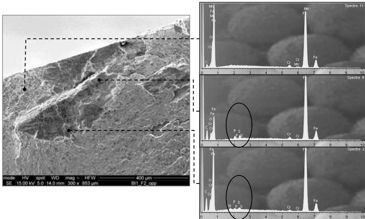
**Fig. 3.15:** SEM-EDX analysis of a WEC fractograph of neutral IR #61 revealing the presence of lubricant compounds all the way down to the crack tip and a wide vertical connection to the raceway (IR cleaned by ethanol ultrasound bath rinsing and immediately put in SEM chamber after fracture).
