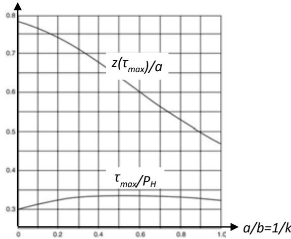
**Fig. 1.10:** Tresca shear stress  $\tau_{max}$  and respective depth  $z(\tau_{max})$  at  $x=0$  function ratio of the degree of ellipticity: case of a line contact for  $a/b=0$  with  $\tau_{max}=0.3P_H$  at  $\xi=0.78a$ ; case of a circular contact for  $a/b=1$  with  $\tau_{max}=0.31P_H$  at  $\xi=0.48a$  (plot adapted from [17]).
