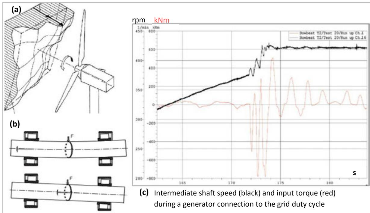
**Fig. 1.23:** Examples of wind turbine loadings affecting the REB tribological contacts: (a) wind fluctuations; (b) REB misalignments due shaft displacement (bottom) or bending (top); typical transient events in wind turbine gearboxes (from [9]).
