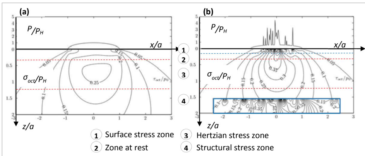
**Fig. 1.12:** (a) Octahedral stress contours and pressure distribution of a Hertzian line contact with a typical friction coefficient  $\mu=0.05$ ; (b) identical as (a) but contacting typical rough surfaces acting as stress raisers (surface zoom) (adapted from [48]).
