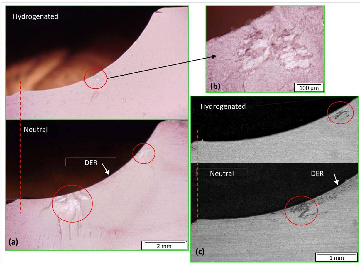
**Fig. 3.10:** WEC different position versus the contact area: (a) fractographs of the H-precharged IR # 28 aligned with that of the neutral IR #7 (opposite side of **Fig. 2.21** (e) ); (b) close-up on the small WEC network of IR #28 at the angle of contact (SEM imaging in **Fig. 3.4** (d)); (c) axial LOM of IR #28 and neutral IR #9 aligned confirming the WEC offset to the border of the DER region in neutral IRs.
