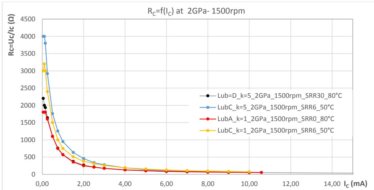
Fig. 2.12: Evolution of the contact resistance  $R_C$  as a function of the input current  $I_C$  for different TDM contacts at  $P_H=2$  GPa,  $U_r=11$  m/s for varying lubricant, temperature, SRR and ellipsoid ratio  $k$ .
