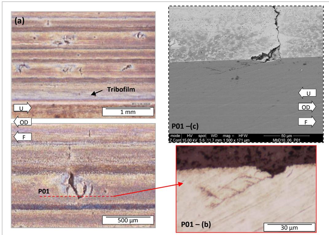
**Fig. 5.11:** TDM10\_06 crowned roller typical raceway topview (a), circumferential LOM (b) and SEM  $\frac{3}{4}$  view of the circumferential cross section and raceway microcrack revealing some crack ramifications opposite to OD without adjacent WEA (propagation phase,  $2.9 \times 10^7$  cycles, 3 GPa, 30% SRR, driver, 85°C water contamination, and regular EDTA cleaning of the tribofilm, subsequent to microcrack pre-initiation with a dented counter-roller).
