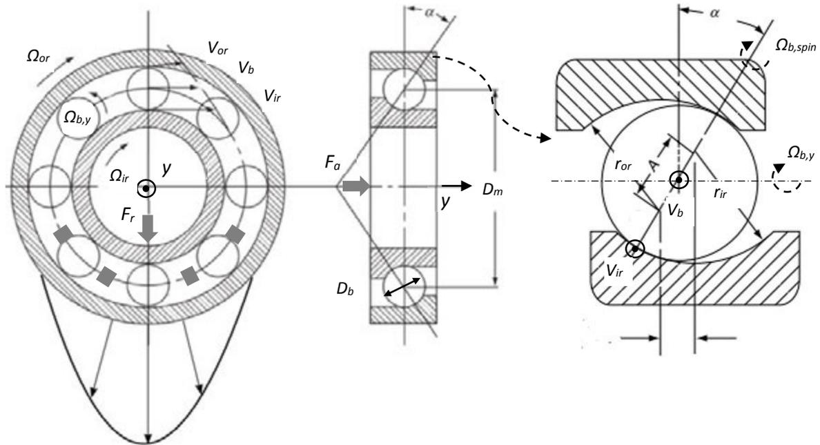
**Fig. 1.16:** Basic rolling kinematics of an angular contact ball bearing under a typical load illustrating the different velocities, contact angle, osculation and dynamic effects of the cage (adapted from [17]).
