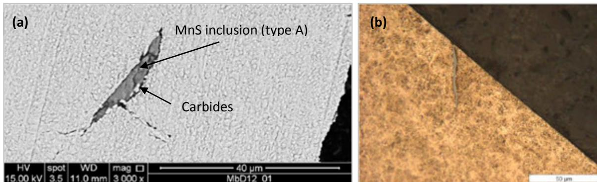
**Fig. 1.4:** (a) SEM image of a manganese sulfide (MnS) inclusion and (b) optical micrograph of another MnS emerging inclusions both found in a 100Cr6 D2 specimen.
