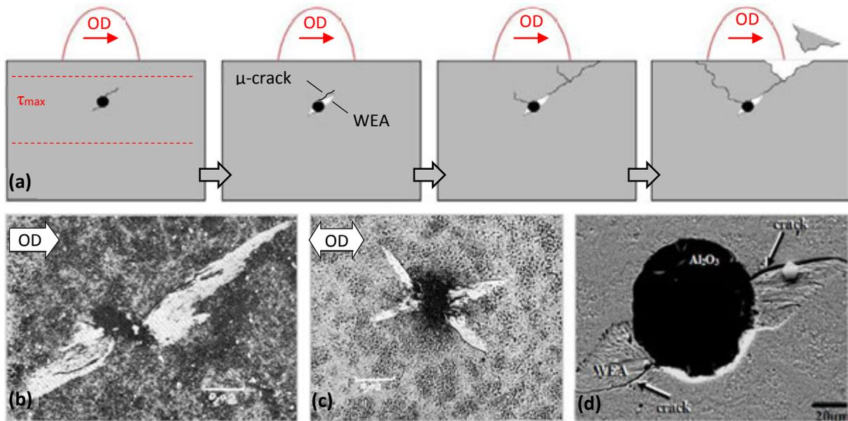
Fig. 1.32: (a) Development of a butterfly in the Hertzian shear stress zone leading to subsurface initiated spalling; (b) Typical development of the butterfly wings at  $\sim 45^\circ$  versus the surface in the direction of OD [125]; (c) Double-winged butterfly in case of alternating OD [125]; (d) Typical SEM analysis of an incipient butterfly composed of lateral micro-cracks and WEA (from [124]).
