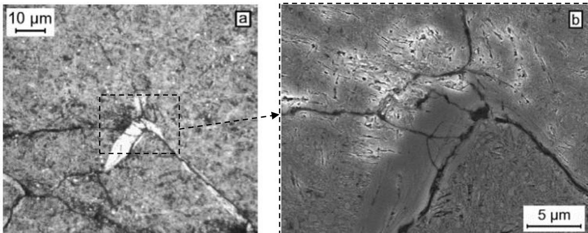
**Fig. 1.40:** Typical WEA bordering cracks of a multi-branching WEC network in (a) a LOM and (b) SEM micrographs of an etched cross section of a gearbox TRB IR (from [29]).
