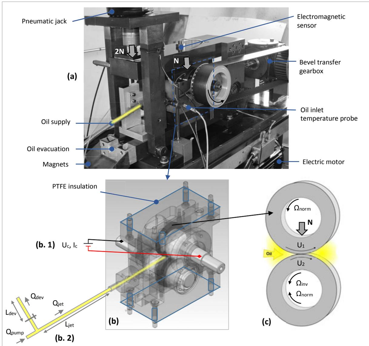
**Fig. 2.6:** LaMCoS TDM RCF test rig: (a) Main operational components and sensors; (b) Scheme of the roller mounting and optional specific installations to (1) impose an electric potential or current through the contact and to (2) regulate the jet oil flow  $Q_{jet}$  by varying the relative pipe losses of an opened deviation; (c) Scheme of the twin-disc tribological contact parameters.
