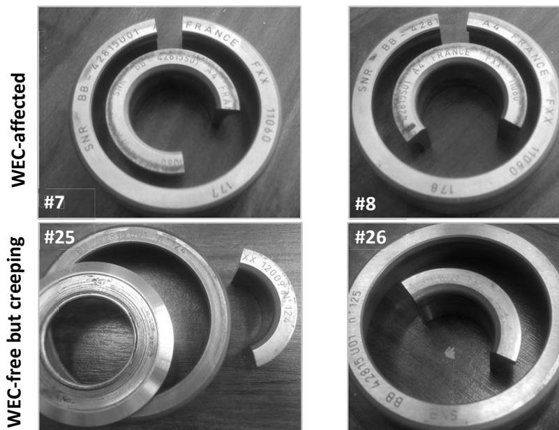
Fig. 4.7: ACBB ring flanges aspect after RCF tests.
