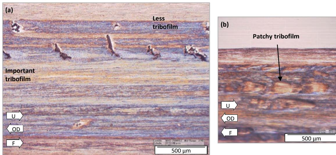
Fig. 5.13: Typical TDM13\_02 raceway topview of (a) cylindrical follower roller and (b) crowned driver roller ( $2.5 \times 10^7$  cycles, 3 GPa, 30% SRR, lubricant B at 85°C, water contamination and 50mA).
