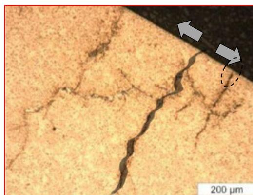
**Fig. 2.23:** Circumferential cross sections of a WEC suggesting a preferential plane of fracture under three point bending tensile induced stress which would not reveal the circled WEC link to surface (original figure available in **Fig. 1.39** (b)).
