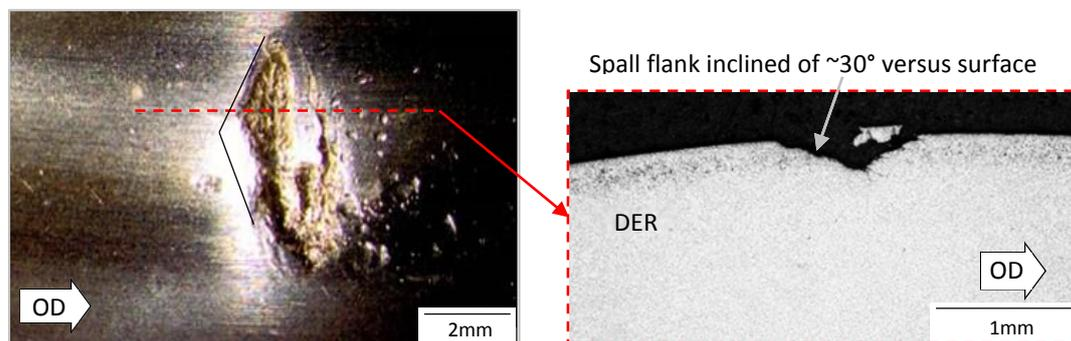
**Fig. 1.33:** Topview and corresponding circumferential metallographic cross section of a surface initiated spall on an ACBB IR during after  $\sim 50 \times 10^6$  cycles of in-house testing: the V-shape indicates the position of the initial detrimental dent.
