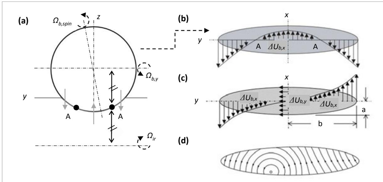
**Fig. 1.17:** (a) Heathcote conforming osculation with two lines of pure rolling in A; (b) ball contact sliding velocities in a radial loaded DGBB representing Heathcote slip; (c) ball contact sliding velocities in an ACBB accounting for transverse spinning motions; (d) overall sliding velocity lines in an ACBB without considering skidding (b, c, and d adapted from [17]).
