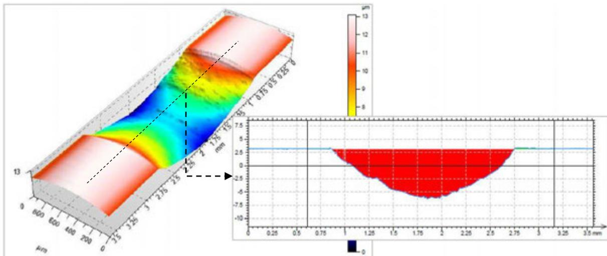
**Fig. 1.26:** Significant mild wear profile of a 100Cr6 driver roller after  $10^6$  cycles with important material removal measured by SENSOFAR PLu neox optical profilometer (Appendix H ref TDM09\_04).
