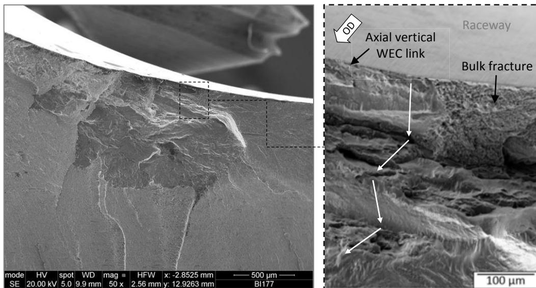
**Fig. 3.12:** Fractograph SEM close-up on the WEC connection to the surface revealing a smooth vertical preexistent axial crack consistent with those observed in surface analyses (**Fig. 3.3** (b)). The white arrows suggest a stair-like top down growth in the direction of OD (neutral IR #7).
