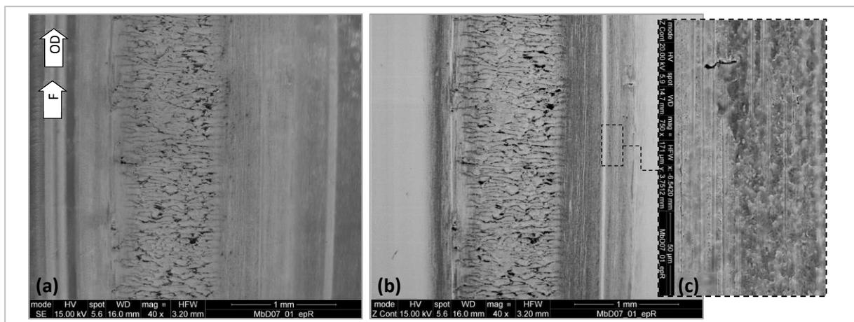
**Fig. 2.17:** SEM-EDX analysis led on a TDM specimen subjected to high surface distress and tribofilm deposit (Appendix H ref TDM07\_01\_II): (a) SE imaging; (b) BSE imaging revealing chemical deposits; (c) magnification of tribofilm deposit further confirmed by EDX analysis.
