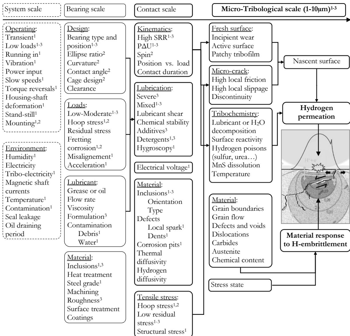
**Fig. 5.1:** Partial overview of influent drivers on WEC formation from macro to tribo-scales suggested by <sup>1</sup>wind turbine REB, <sup>2</sup>ACBB and <sup>3</sup>CRTB WEC occurrences. Examples of interactions suggested by arrows.
