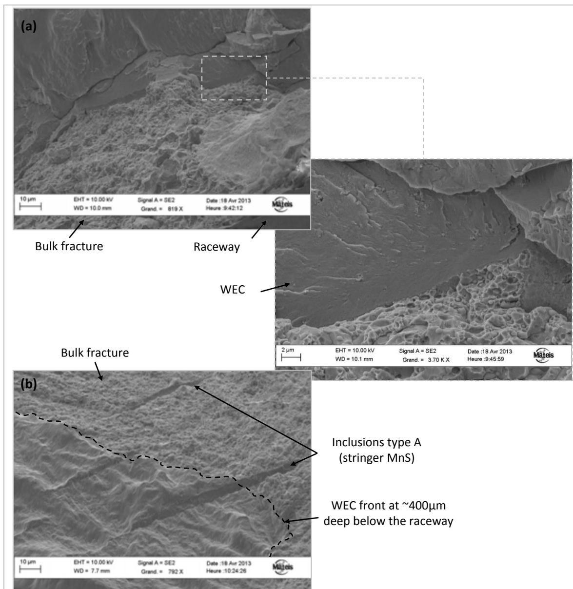
**Fig. 3.9:** SEM top view imaging of a WEC fractograph at the contact border of neutral IR #7 (SEM SUPRA 55 VP available at MATEIS): (a) close-up on the striated preexistent WEC crack flank near the raceway; (b) close-up on type A MnS inclusions in the vicinity of WEC crack tip far beneath the raceway.
