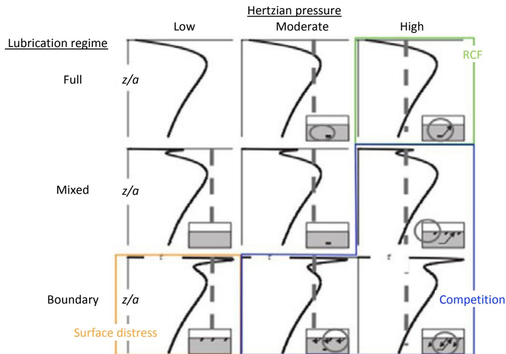
**Fig. 1.35:** Competition between surface distress and RCF failure modes of REBs depending on the tribological operating conditions and induced subsurface shear stress (adapted from [114]).
