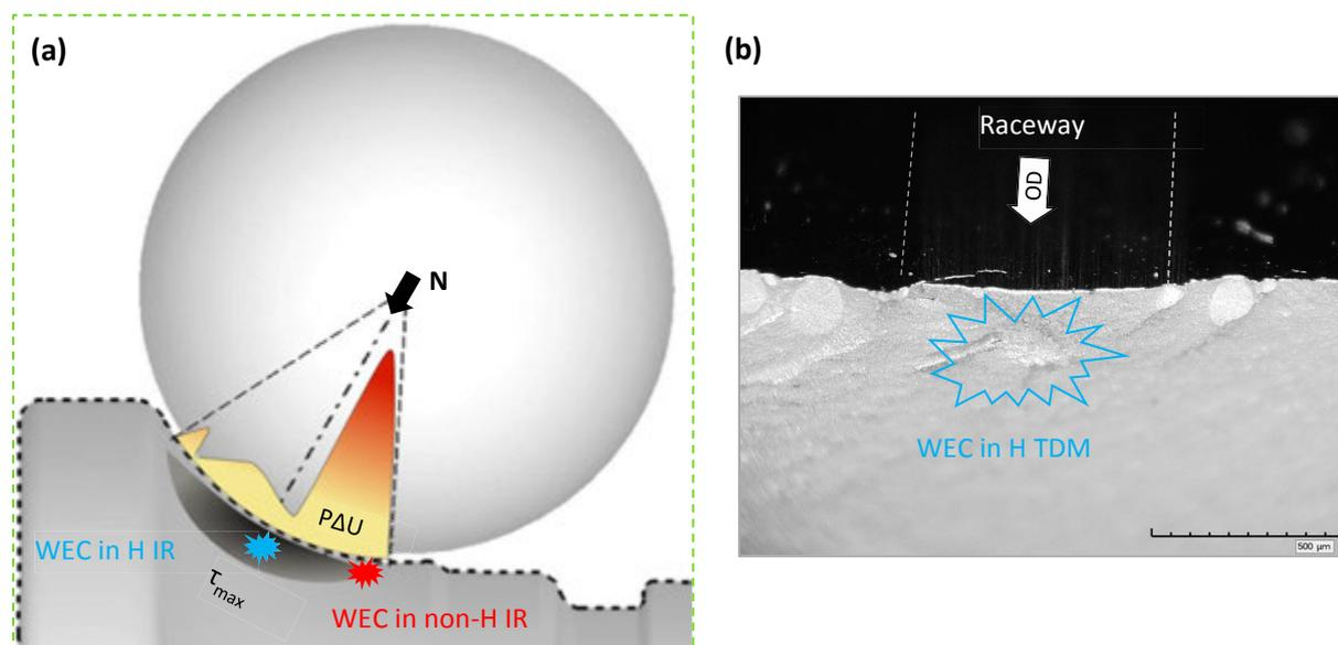
**Fig. 3.11:** (a) Scheme illustrating the WEC location versus the contact area in non-H-precharged and H-precharged ACBB IR; (b) Three-quarter view of the H-precharged (H) TDM roller fractograph revealing a WEC at the center of contact below the raceway (cf. **Fig. 3.5**).
