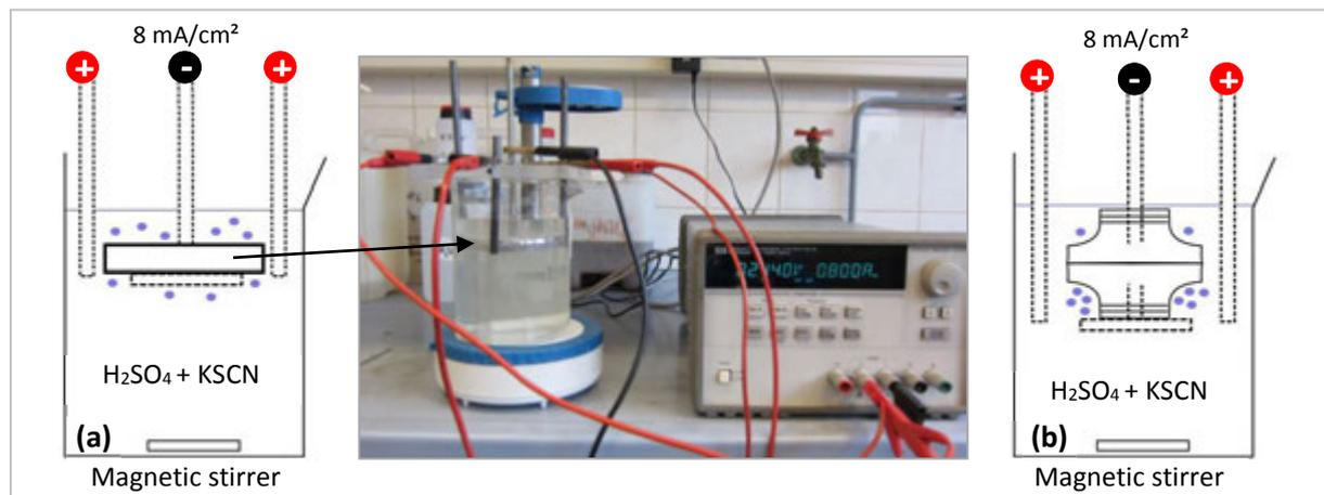
**Fig. 3.1:** Electrolytic hydrogen charging protocol of TDM specimens (a) and Machine S ACBB IR (b).
