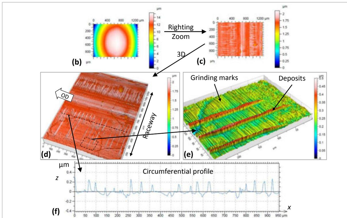
**Fig. 2.16:** Example of topography measurement by SENSOFAR PLu neox post-treated with MountainsMap (Appendix H ref TDM12\_02): (a) raw measurement of a crown disc; (b) zoom at the raceway after righting; (c) 3D visual; (d) Close-up on features perpendicular to the circumferential grinding marks; (e) circumferential profile confirming regular transverse stripes of material deposit.
