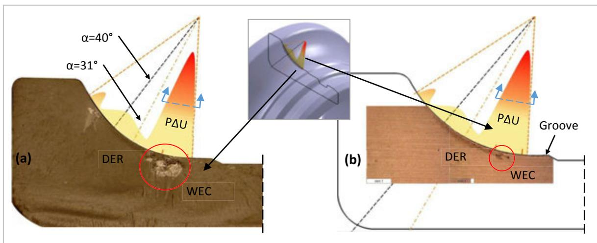
**Fig. 4.14:** Superposition of the  $P.\Delta U$  profile along the major axis of the most loaded ball/IR contact (contact angle  $\alpha=30.7^\circ$ ) for the ACBB tests load case 1: (a) fractographs of IR #9 and (b) stitched axial LOM of IR #7. Repositioning is achieved by aligning the respective grooves and flanges.
