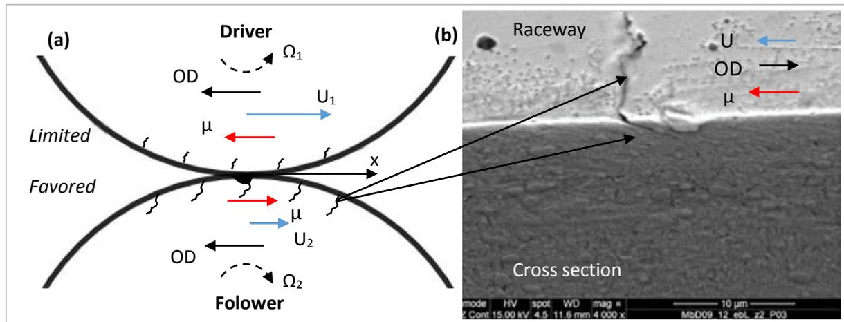
**Fig. 1.28:** (a) Scheme of microcrack development function of the contact kinematics and friction forces illustrating that surface microcrack propagation is favored on the follower surface; (b) SEM analysis of a 100Cr6 follower roller revealing a typical incipient surface microcrack (Appendix H ref TDM09\_12).
