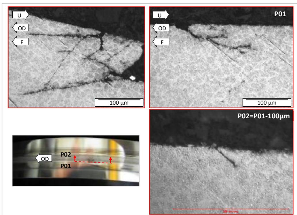
**Fig. 5.10:** TDM07\_01\_II cylindrical roller circumferential LOM (propagation phase,  $3.0 \times 10^7$  cycles, 3.4 GPa, 30% SRR, driver, subsequent to microcrack pre-initiation with a dented counter-roller).
