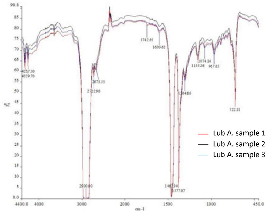
Fig. 4.12: Infrared transmission spectrometry assessment on three different samples of lubricant A
