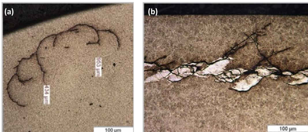
**Fig. 1.44:** (a) LOM of an automotive wheel ACBB through-hardened 100Cr6 ball;
