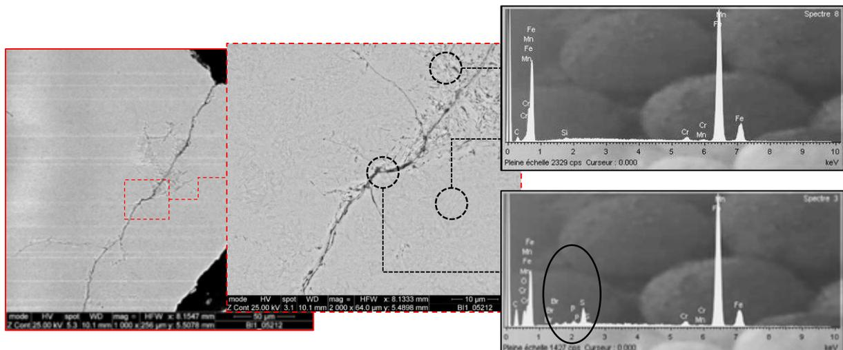
**Fig. 3.16:** SEM-EDX analysis of a circumferential cross section of neutral IR #61 revealing a WEC network connected to the surface with the presence of lubricant compounds deep into the primary crack but not in the adjacent WEA.
