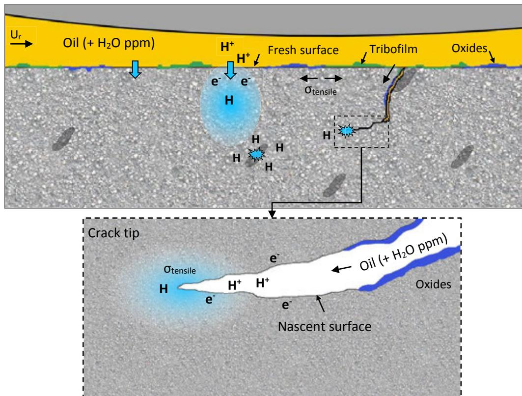
**Fig. 4.18:** Scheme of hydrogen permeation into the steel: lubricant or water molecules are chemisorpted at tensely stressed nascent metal surfaces at the raceway or at microcrack tips liberating highly diffusible hydrogen that is eventually trapped in the vicinity of defects such as inclusions.
