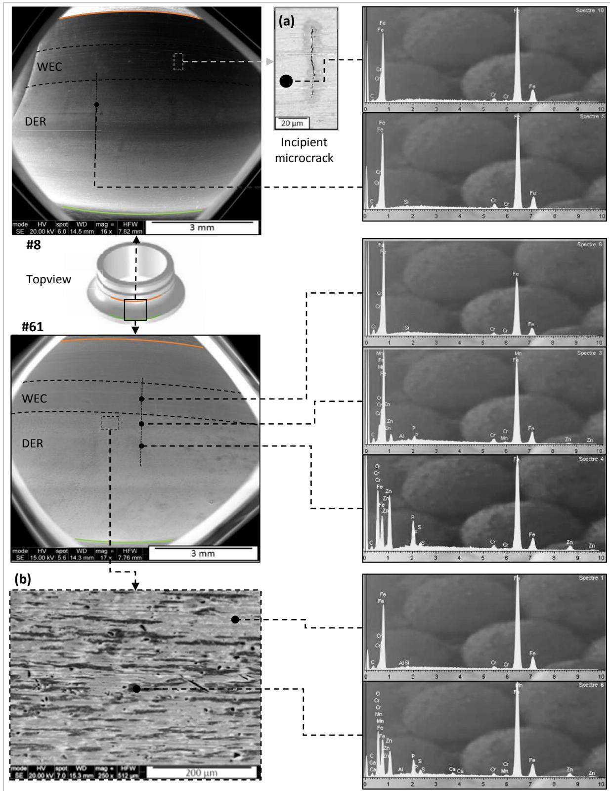
**Fig. 4.9:** Typical results of SEM EDX linear tribefilm analysis performed on raceway topview of *WEC*-affected IR #8 (standard cage clearance) and #61 (oblong cage clearance) providing close-ups on (a) an axial incipient microcracks positioned at  $\sim 2$  mm from the groove in the *WEC* region, and on (b) heterogeneous and stripped tribefilm at the contact border nearby the *WEC* region (N.B. the size of the EDX spot represented is not scaled but is here as a reminder).
