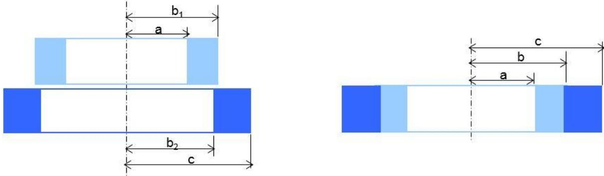
The following equations allow to approximate the stresses induced by fitting a ring on a shaft by the geometry of the above schemes for a given fit value  $\delta = b_1 - b_2$ . The press-fit pressure at the interface  $P_{fit}$  is given by:
