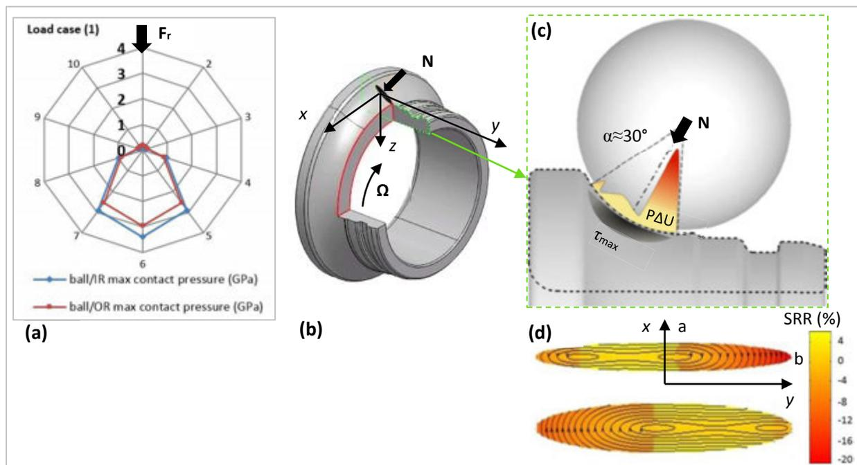
**Fig. 2.4:** (a) Contact pressure distribution in the ACBB; (b) Scheme of a cross sectioned IR of the tested ACBB; Schemes of the tribological parameters for the most loaded ball/IR contact in load case (1) with (b) illustrating the effective contact angle, subsurface shear stress and P $\Delta$ U sliding energy criterion, and (c) the SRR lines in the IR and OR respective contact ellipsoid.
