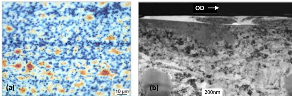
**Fig. 1.21:** (a) Optical image of a typical spotted ZDDP tribofilm (from [85]); (b) Typical cross section of a wear track revealing the heterogeneous structure of a MoS<sub>2</sub> based tribofilm (from [83]).
