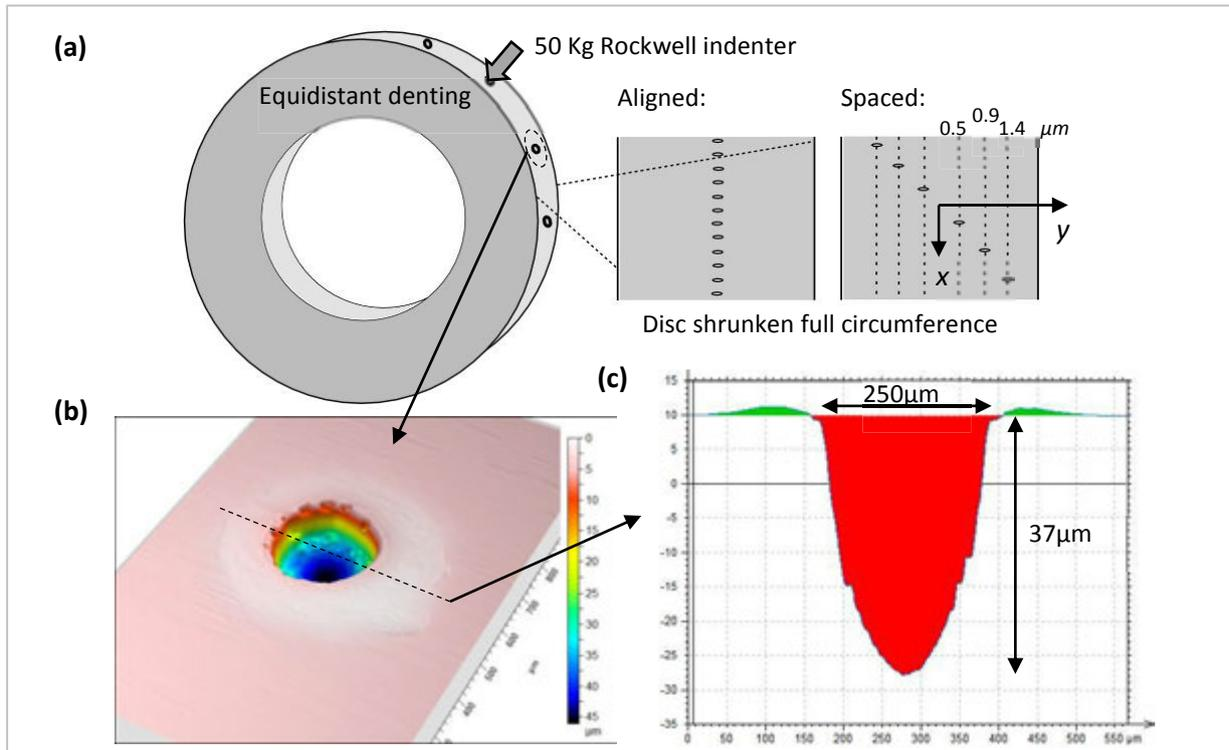
**Fig. 2.10:** Artificial dent analysis prior to RCF testing: (a) schemes of different dent positionings on the disc circumferences; (b) 3D dent topography and (c) profile measured with SENSOFAR PLu neox.
