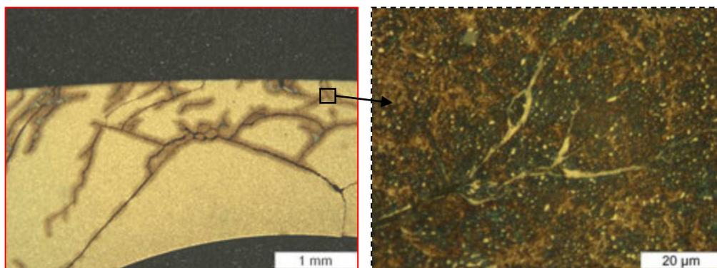
**Fig. 5.14:** Circumferential LOM of TDM11\_00 cylindrical roller with holes inducing additional structural stresses (3.5 GPa, 7% SRR, driver, lubricant PAO8 at 80°C) (cracks are emphasized due to etchant trap in their vicinity).
