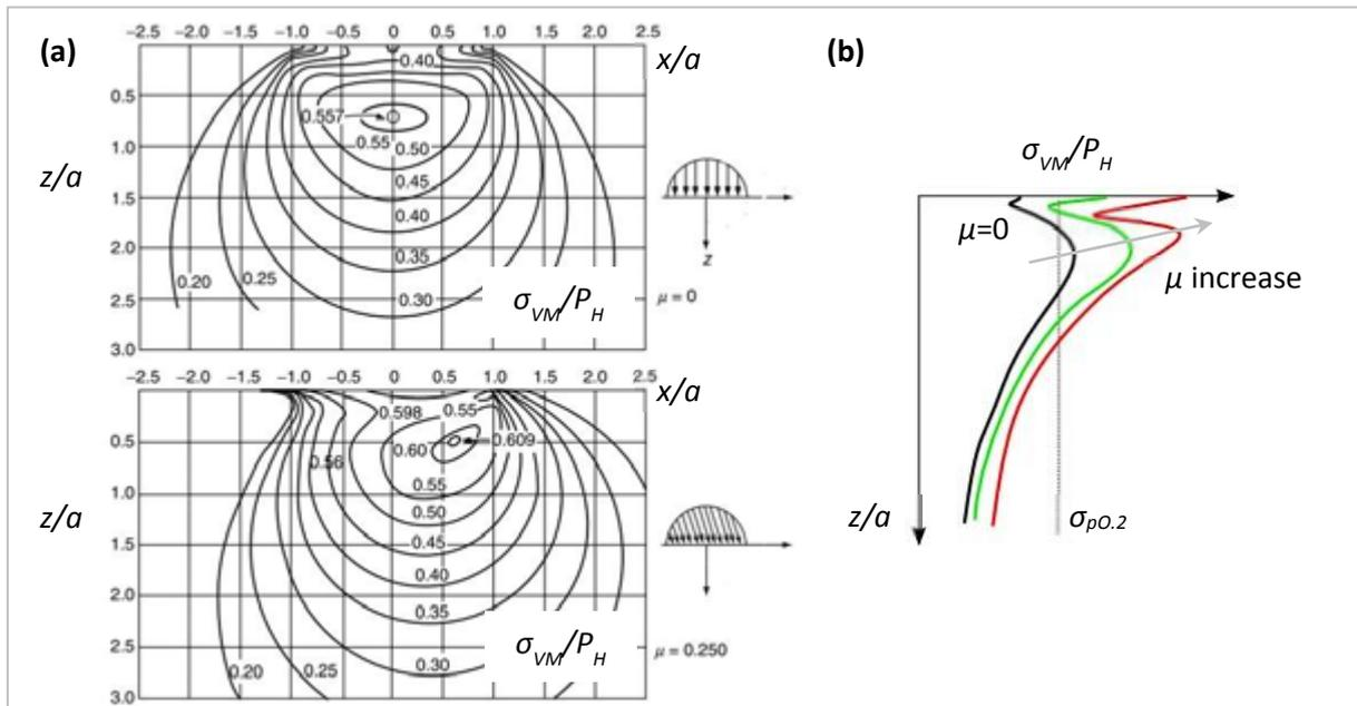
**Fig. 1.15:** (a) Comparison of the contours of Von Mises stress for frictionless hertzian contact and for a friction coefficient  $\mu=0.25$  (adapted from [17]) with the same normal load; (b) Typical Von Mises stress profile modification as the friction coefficient increases.
