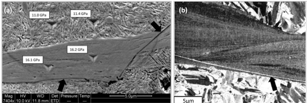
**Fig. 1.41:** (a) WEC close-up using SEM analysis with corresponding nanohardness indentations in the bulk matrix and the WEA (from [6]); (b) WEC close-up using ion channeling contrast to reveal linear feature inside WEAs developed mainly on the upper bound of the cracks (black arrow) but also incipiently on the lower bound, as in (a) (from [14]).
