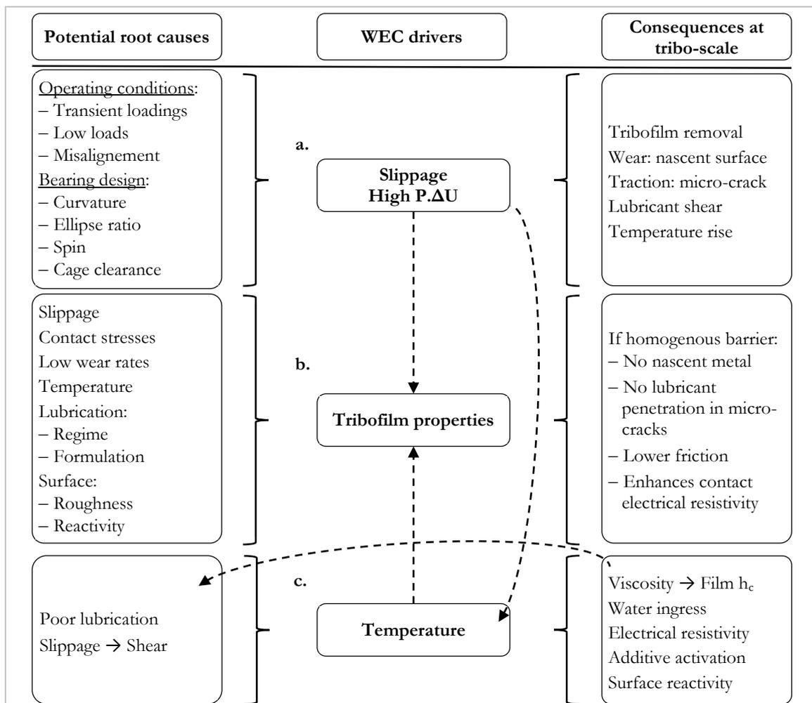
**Fig. 5.3:** Examples of different root causes leading to similar WEC drivers and multiple consequences at tribo-scales all influencing each other: (a) slippage, (b) tribofilm properties, (c) temperature
