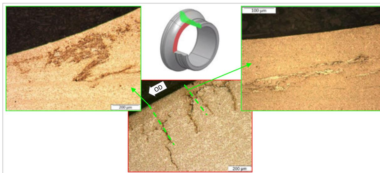
**Fig. 3.6:** Axial and circumferential LOMs of the neutral IR #7 revealing different morphological layouts of WECs and suggesting a possible interpretation of the different WEC aspects on the two axial LOMs.
