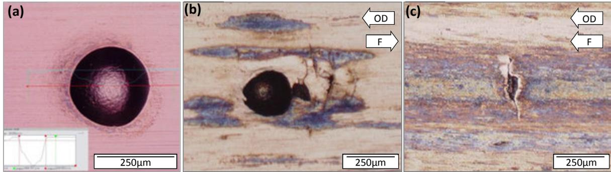
**Fig. 2.9:** LOM topview of disc raceways: (a) Artificial dent (50 Kg Rockwell indenter prior to testing); (b) Dent evolution after RCF testing on the follower surface (Appendix H ref TDM07\_07) (c) Typical surface initiated crack at the raceway border on the counter driver roller (Appendix H ref TDM07\_02\_I\_b).
