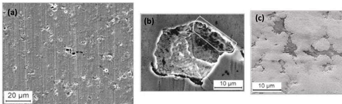
**Fig. 1.25:** Typical SEM analyses of tribochemically induced micropits on a IR raceway ((a-b) from [29]); Tribochemical surface distress of the tribofilm due to water contamination of the lubricant (from [109]).
