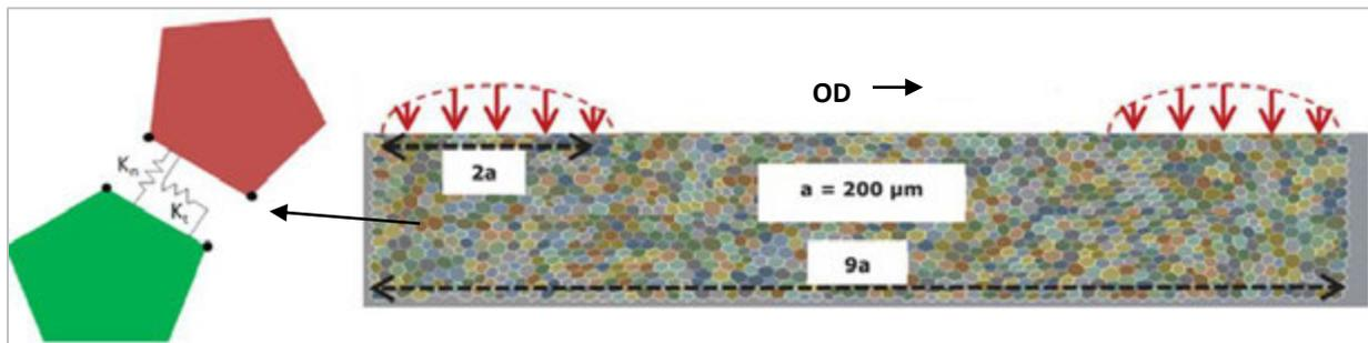
Fig. 1.37: Example of a cohesive finite element model simulating damage accumulation at grain boundaries to predict crack initiation in RCF conditions (from [161]).
