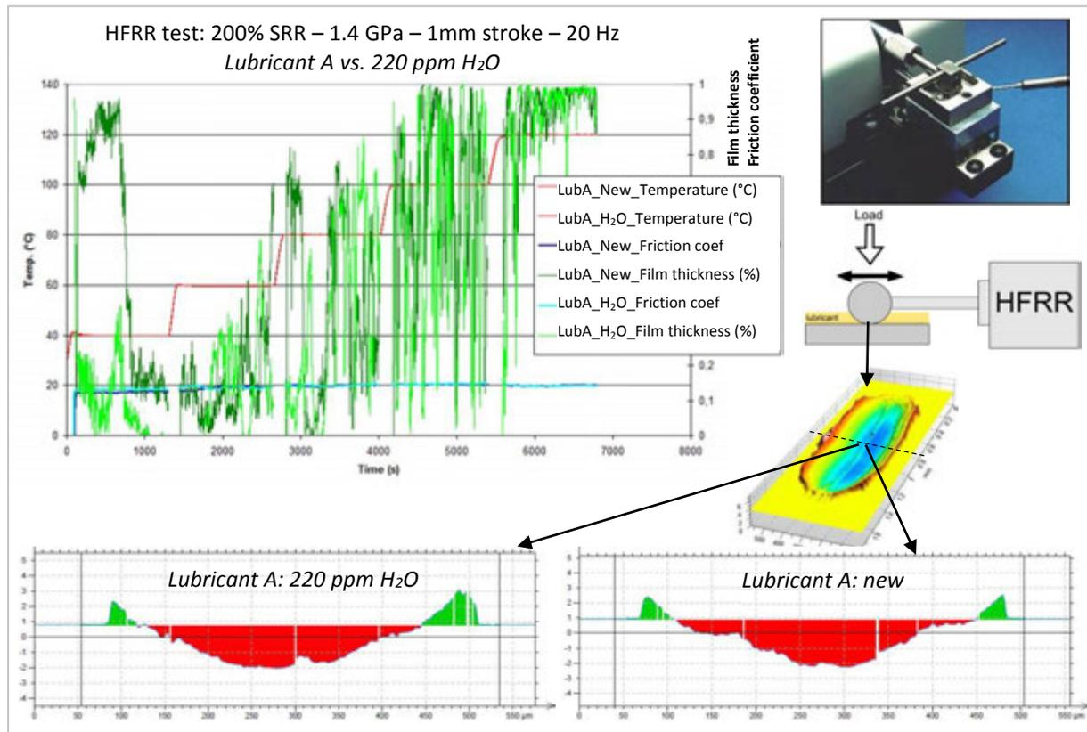
**Fig. 2.14:** Typical HFRR test result and wear scar profile by SENSOFAR PLu neox revealing respectively similar friction coefficient evolutions with the temperature and similar wear scars for lubricant A at neutral state and with 220 wt. ppm of artificially ingressed water.
