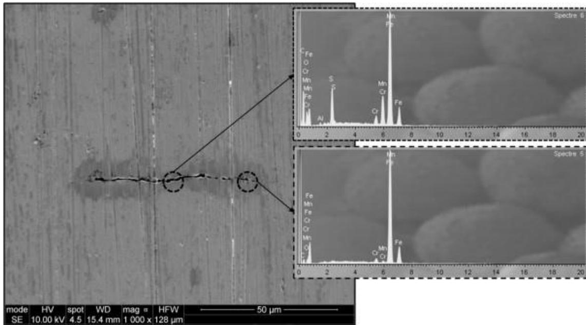
**Fig. 4.17:** SEM-EDX analysis of an axial microcrack observed in the contact edges of WEC-affected ACBB IR #8 revealing high manganese and sulfur contents in the crack vicinity suggesting the crack has been initiated due to the presence and/or dissolution of a type A inclusion near the surface [29].
