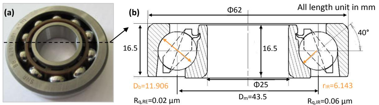
**Fig. 2.3:** (a) NTN-SNR ACBB with 10 balls and a polyamide cage used in this study; (b) Cross section of the ACBB with the mean diameter  $D_m$ , the ball diameter  $D_b$  and the IR curvature  $r_{IR}$
