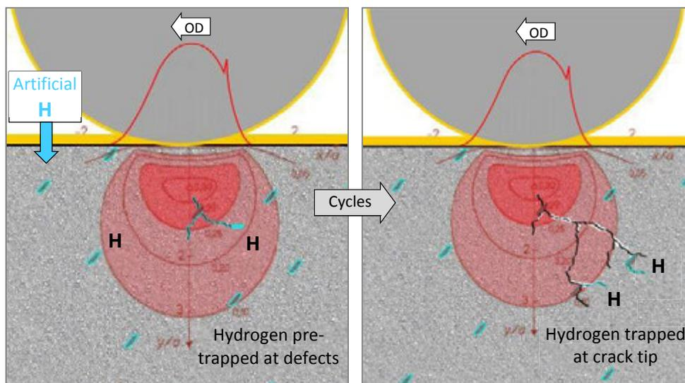
Fig. 3.14: Scheme of WEC formation conjecture in H-precharged specimens where crack initiation occurs in the subsurface maximum shear stress zone due to excessive steel embrittlement
