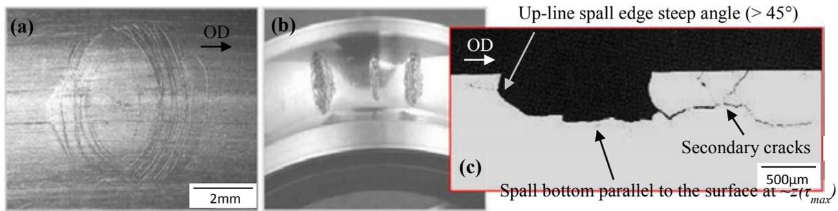
**Fig. 1.34:** (a) Top-view of a developing subsurface initiated spall presenting a typical oval form with more incipient cracks developing on the down-line edge; (b) Propagated subsurface initiated spalls on a DGBB IR; (c) Circumferential cross section revealing the typical morphology of a subsurface initiated spall.
