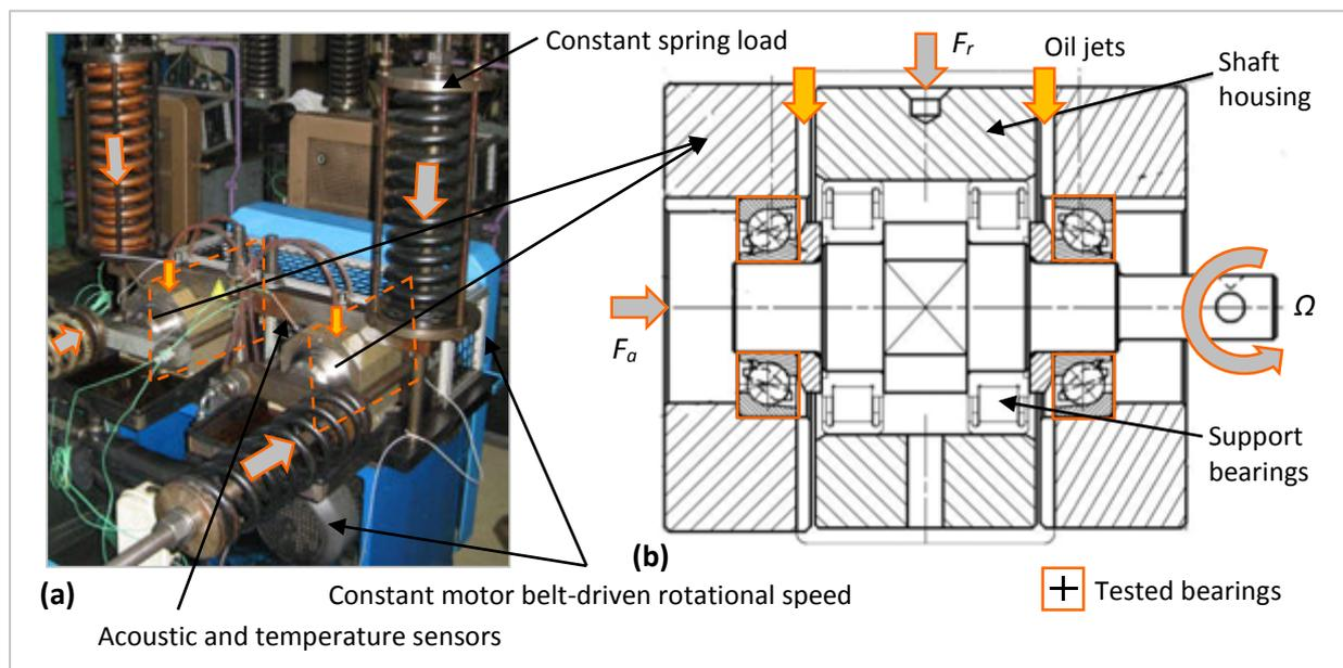
**Fig. 2.2:** (a) NTN-SNR Machine S endurance test rig;
