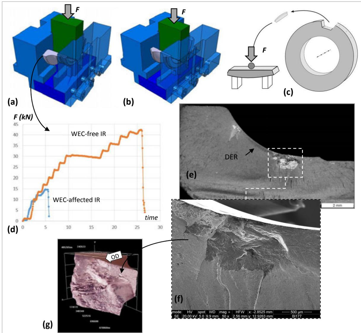
**Fig. 2.21:** Fractography protocol established to force open and reveal WECs: examples of specifically designed tools for ACBB IRs (a) and DGBB IRs (b); pre-sectioning and three-point bending for TDM raceway fractographs; (d) fractography load monitoring; (e) binocular microscopy of an ACBB IR fractograph revealing wide WEC networks; (f) SEM analysis close-up on the WEC network in (e); (g) WEC fractograph 3D assessment on HIROX KH-7700.
