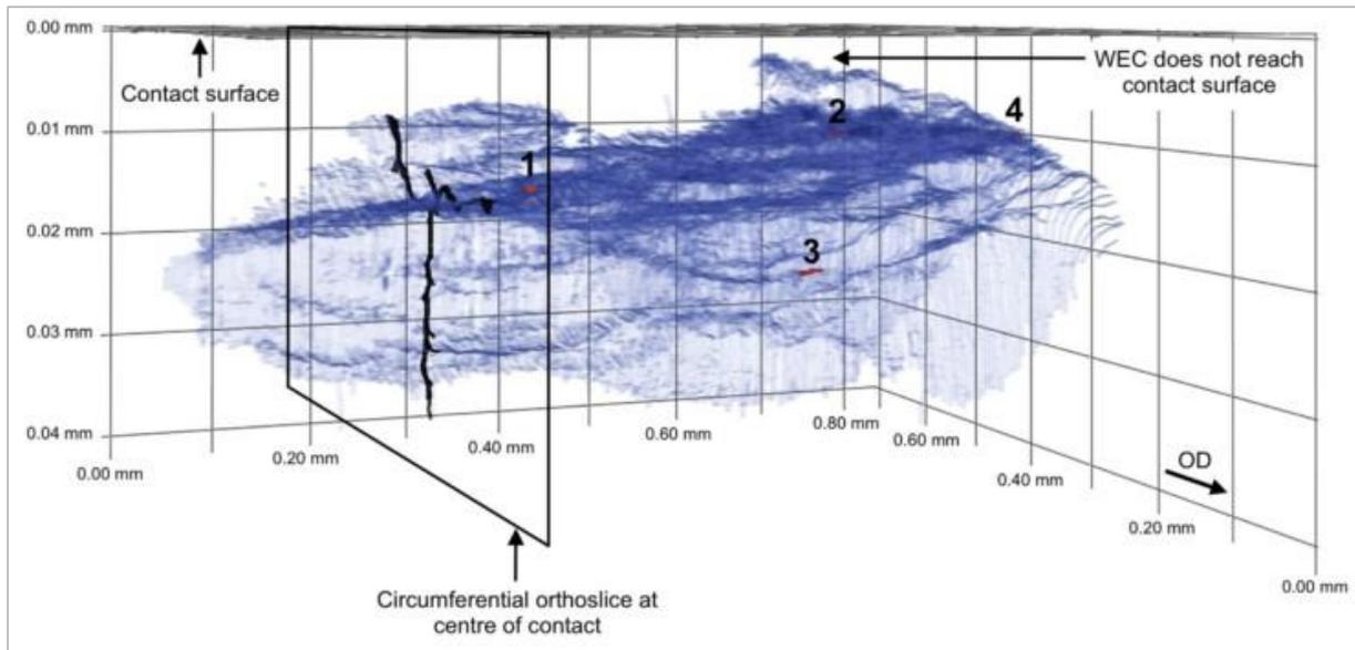
**Fig. 1.43:** 3D mapping of a WEC network reconstructed by manual serial-sectioning and segmentation techniques (in red, inclusion interacting with the cracks) [188].
