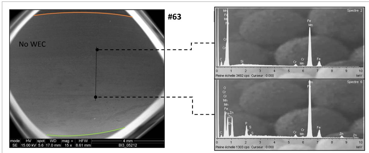
Fig. 4.10: Typical results of SEM EDX linear tribofilm analysis performed on raceway topview of *WEC-free* IR #63 (oblong cage clearance).
