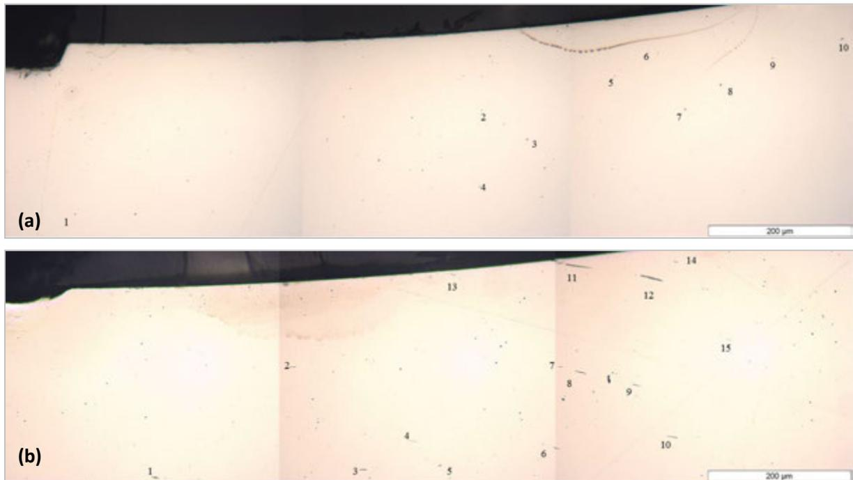
**Fig. 2.5:** Axial LOM prior to Nital etching revealing type A inclusions (MnS) of different morphologies and orientations vs. the raceway in forged (a) and turned (b) IRs coming from two different steel batches.
