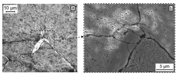
**Fig. 1.40**: Typical WEA bordering cracks of a multi-branching WEC network in (a) a LOM and (b) SEM micrographs of an etched cross section of a gearbox TRB IR (from [29]).
