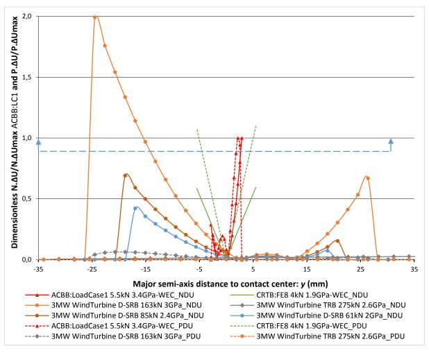
P being the local contact pressure, N the global contact load and  $\Delta U$  the local slip velocity. The dashed blue line represents a possible threshold for WEC formation.
