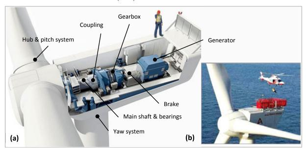
**Figure 4**: Typical horizontal axis MW wind turbine structure at the top of the tower (courtesy of ZF transmission, www.zf.com); (b) AREVA M5000 5 MW wind turbine maintenance [3].
