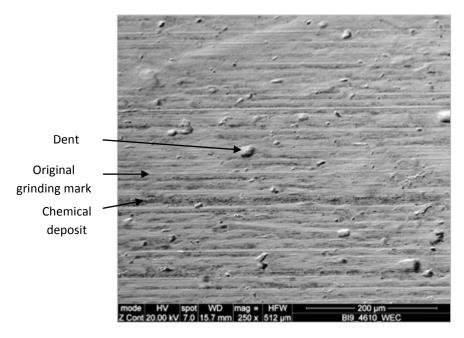
**Fig. 1.13**: Typical SEM analysis of an ACBB IR raceway revealing dents after 1265 h of service (#9 Appendix D).
