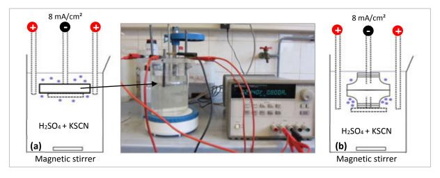
Fig. 3.1: Electrolytic hydrogen charging protocol of TDM specimens (a) and Machine S ACBB IR (b).
