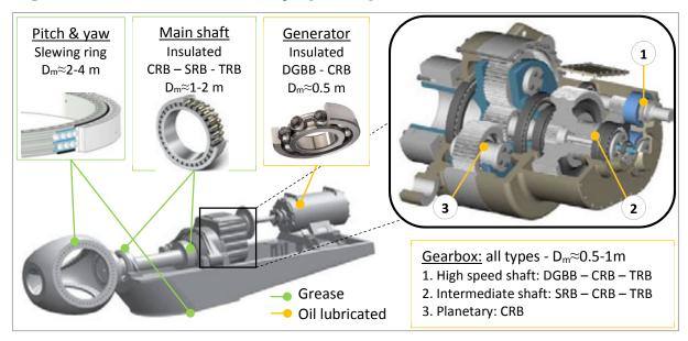
Fig. 1.6: Overview of REB arrangements in a typical MW wind turbine.
