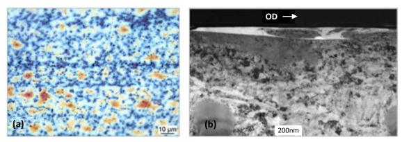
Fig. 1.21: (a) Optical image of a typical spotted ZDDP tribofilm (from [85]); (b) Typical cross section of a wear track revealing the heterogeneous structure of a MoS<sub>2</sub> based tribofilm (from [83]).
