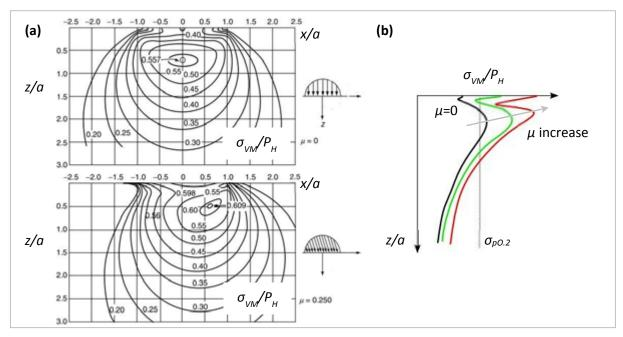
Fig. 1.15: (a) Comparison of the contours of Von Mises stress for frictionless hertzian contact and for a friction coefficient μ=0.25 (adapted from [17]) with the same normal load;
