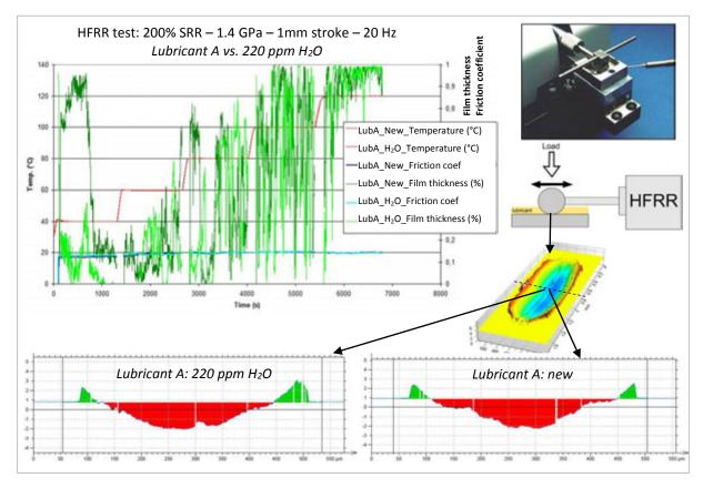
**Fig. 2.14**: Typical HFRR test result and wear scar profile by SENSOFAR PLu neox revealing respectively similar friction coefficient evolutions with the temperature and similar wear scars for lubricant A at neutral state and with 220 wt. ppm of artificially ingressed water.
