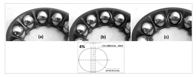
**Fig. 4.3**: (a) standard cage design with spherical pocket (#1-36); (b) enhanced oblong pocket clearance by a 4% circumferential elongation (#37-64); (c) latest design combining oblong pocket and thinner and less-conforming bridges (#65-68).
