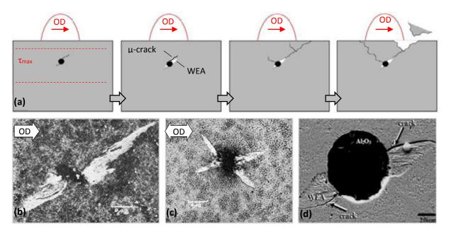
Fig. 1.32: (a) Development of a butterfly in the Hertzian shear stress zone leading to subsurface initiated spalling; (b) Typical development of the butterfly wings at ~45° versus the surface in the direction of OD [125]; (c) Double-winged butterfly in case of alternating OD [125]; (d) Typical SEM analysis of an incipient butterfly composed of lateral micro-cracks and WEA (from [124]).
