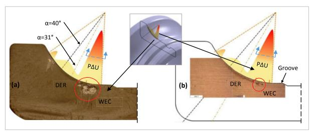
Fig. 4.14: Superposition of the P. $\Delta$ U profile along the major axis of the most loaded ball/IR contact (contact angle  $\alpha$ =30.7°) for the ACBB tests load case 1: (a) fractographs of IR #9 and (b) stitched axial LOM of IR #7. Repositioning is achieved by aligning the respective grooves and flanges.
