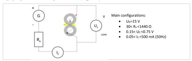
Fig. 2.11: Scheme of the electrical circuit deployed on the TDM.
