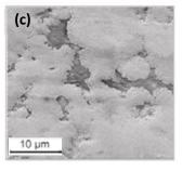
**Fig. 1.25**: Typical SEM analyses of tribochemically induced micropits on a IR raceway ((a-b) from [29]); Tribochemical surface distress of the tribofilm due to water contamination of the lubricant (from [109]).
