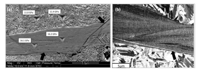
Fig. 1.41: (a) WEC close-up using SEM analysis with corresponding nanohardness indentations in the bulk matrix and the WEA (from [6]); (b) WEC close-up using ion channeling contrast to reveal linear feature inside WEAs developed mainly on the upper bound of the cracks (black arrow) but also incipiently on the lower bound, as in (a) (from [14]).
