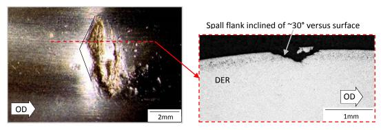
**Fig. 1.33**: Topview and corresponding circumferential metallographic cross section of a surface initiated spall on an ACBB IR during after ~50x106 cycles of in-house testing: the V-shape indicates the position of the initial detrimental dent.
