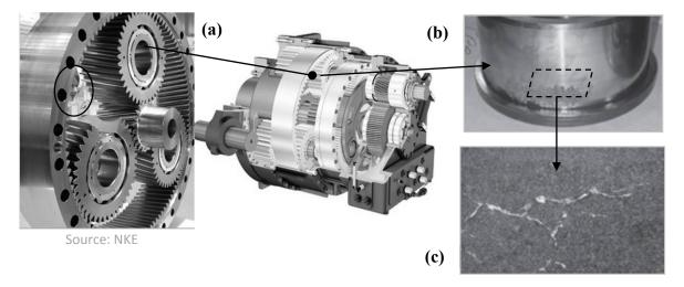
**Figure 8:** (a) Multi-MW wind turbine gearbox layout and size compared to a human head; (b) Example of wind turbine REB fatigue failure [7] associated to (c) the formation of White Etching Cracks (WEC) [7].
