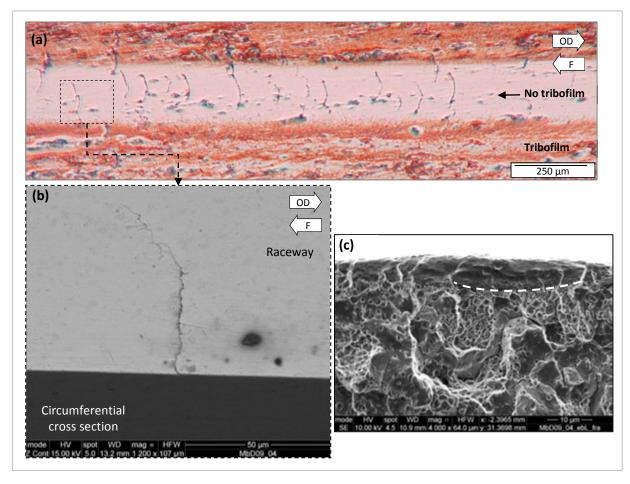
Fig. 5.12: TDM09\_04 crowned roller typical raceway center topview (a), SEM <sup>3</sup>/<sub>4</sub> view of a circumferential cross section (b), and SEM analysis of a raceway fractographs opening a shallow surface microcrack (initiation phase; 1.9x10<sup>7</sup> cycles, 2 GPa, 7% SRR, follower, lubricant A at 50°C).
