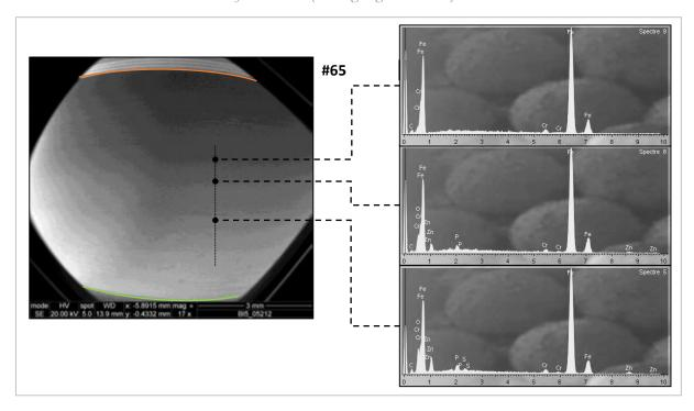
**Fig. 4.11**: Typical results of SEM EDX linear tribofilm analysis performed on raceway topview of WEC-free IR #65 (oblong cage clearance plus less-conforming bridges).
