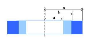
The following equations allow to approximate the stresses induced by fitting a ring on a shaft by the geometry of the above schemes for a given fit value  $\delta = b1-b2$ . The press-fit pressure at the interface  $Pf_{it}$  is given by:
