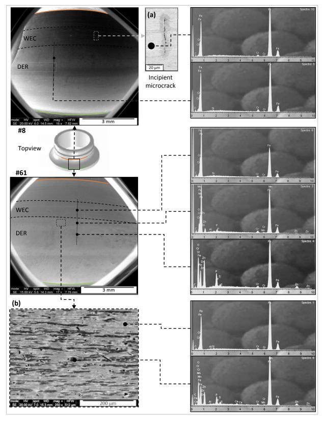
Fig. 4.9: Typical results of SEM EDX linear tribofilm analysis performed on raceway topview of WEC-affected IR #8 (standard cage clearance) and #61 (oblong cage clearance) providing close-ups on (a) an axial incipient microcracks positioned at ~2 mm from the groove in the WEC region, and on (b) heterogeneous and stripped tribofilm at the contact border nearby the WEC region (N.B. the size of the EDX spot represented is not scaled but is here as a reminder).
