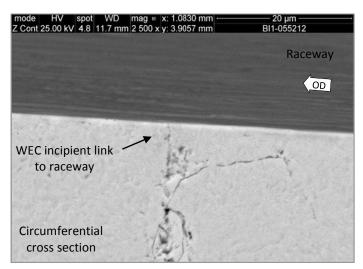
**Fig. 3.13**: SEM close-up on a three-quarter view of an undamaged raceway despite the presence of a WEC network in its vincinity confirmed by a circumferential unetched cross section (IR #61).
