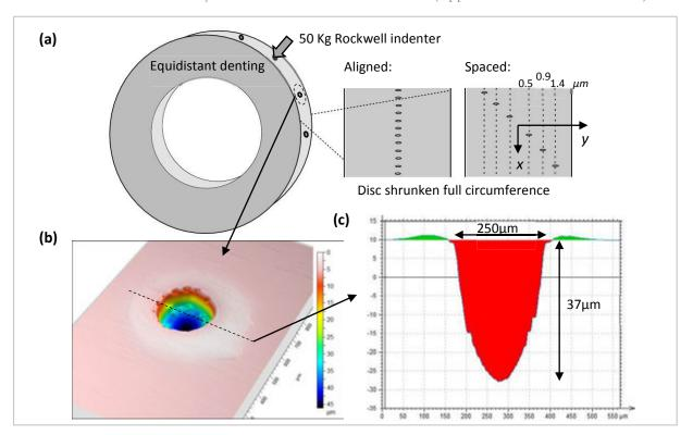
Fig. 2.10: Artificial dent analysis prior to RCF testing: (a) schemes of different dent positionings on the disc circumferences; (b) 3D dent topography and (c) profile measured with SENSOFAR PLu neox.
