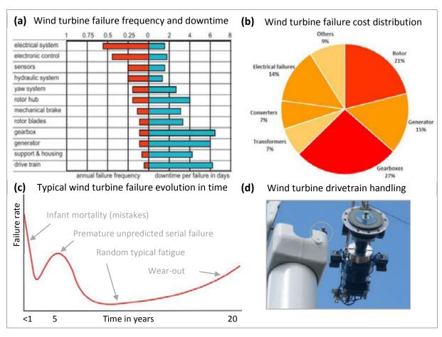
Figure 7: (a) (b) Wind turbine failures distribution in 2009 and the impact on the O&M costs [5]; (c) typical wind turbine failure rate evolution in time with premature failures; (d) wind turbine drivetrain handling.
