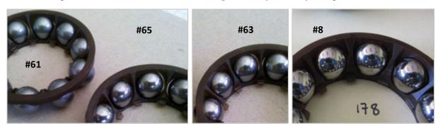
**Fig. 4.5**: WEC-affected ACBB #61 balls with a matt grey coloration; WEC-free ACBB #65 and #63 balls with a shiny aspect; WEC-affected ACBB #8 balls with also a shiny aspect.
