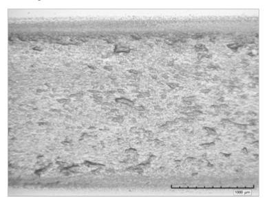
Fig. 1.27: Optical image of advanced smearing on a 100Cr6 driver roller (Appendix H ref TDM03).
