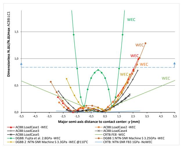
N being the global contact load and  $\triangle U$  the local slip velocity. The dashed blue line represents a possible threshold for WEC formation. c. Dimensionless  $N.\Delta U/\lambda$  along the contact major axis in mm for various WEC-affected and WEC-free tests from NTN-SNR or the literature
