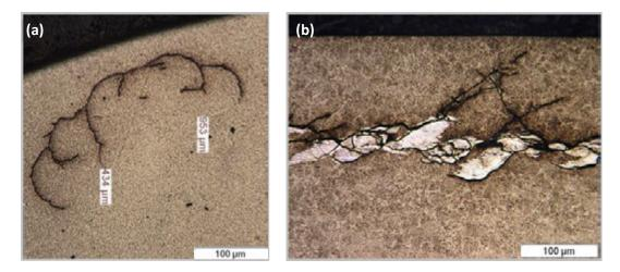
**Fig. 1.44**: (a) LOM of an automotive wheel ACBB through-hardened 100Cr6 ball; (b) LOM of a wind turbine case-hardened TRB IR (courtesy of NTN-SNR)
