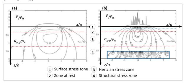
Fig. 1.12: (a) Octahedral stress contours and pressure distribution of a Hertzian line contact with a typical friction coefficient  $\mu$ =0.05; (b) identical as (a) but contacting typical rough surfaces acting as stress raisers (surface zoom) (adapted from [48]).
