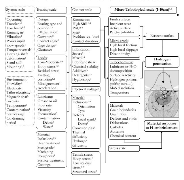
Fig. 5.1: Partial overview of influent drivers on WEC formation from macro to tribo-scales suggested by ¹wind turbine REB, ²ACBB and ³CRTB WEC occurrences. Examples of interactions suggested by arrows.
