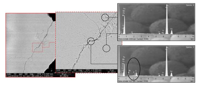
**Fig. 3.16**: SEM-EDX analysis of a circumferential cross section of neutral IR #61 revealing a WEC network connected to the surface with the presence of lubricant compounds deep into the primary crack but not in the adjacent WEA.
