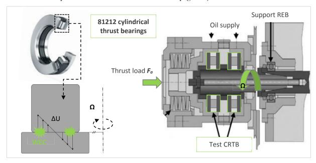
**Fig. 4.1**: Scheme of the 81212 CRTBs tested on a FAG FE-8 test rig with a focus on the induced slip velocities and WEC locations versus the contact area.
