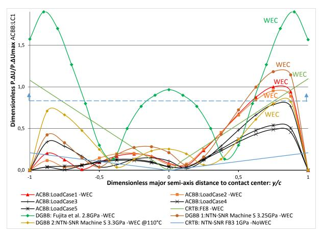
Fig. 5.5: Dimensionless sliding energetic criteria P.ΔU along the contact major axis for various REBs.
