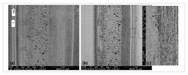
**Fig. 2.17**: SEM-EDX analysis led on a TDM specimen subjected to high surface distress and tribofilm deposit (Appendix H ref TDM07\_01\_II): (a) SE imaging; (b) BSE imaging revealing chemical deposits; (c) magnification of tribofilm deposit further confirmed by EDX analysis.
