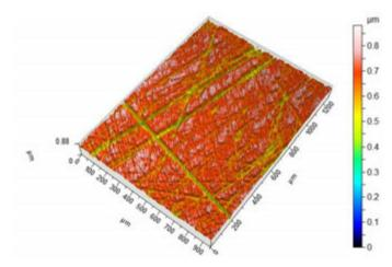
Fig. 4.2: Typical grinding marks on similar NTN-SNR CRTB washers ( $R_a$ =0.10 µm)
