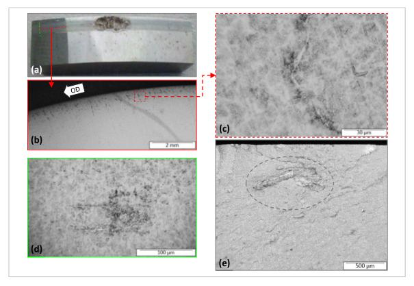
Fig. 3.5: WEC reproduction on the artificial H-precharged TDM roller of TDM08\_01: (a) premature spall, (b) circumferential LOM revealing WEC, (c) close-up on a WEC in the depth of maximum shear stress, (d) axial LOM revealing WEC; (e) axial fractograph revealing a brighter WEC network.
