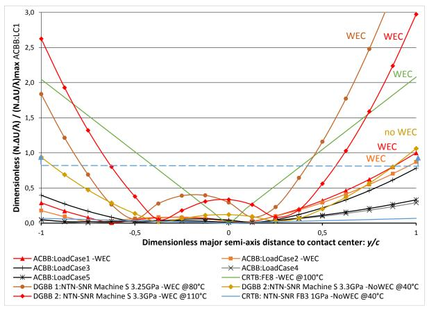
Fig. 5.8: Dimensionless sliding energetic criteria vs. the lubrication parameter  $N.\Delta U/\lambda$  for various REBs.
