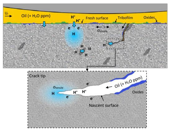
**Fig. 4.18**: Scheme of hydrogen permeation into the steel: lubricant or water molecules are chemisorpted at tensely stressed nascent metal surfaces at the raceway or at microcrack tips liberating highly diffusible hydrogen that is eventually trapped in the vicinity of defects such as inclusions.
