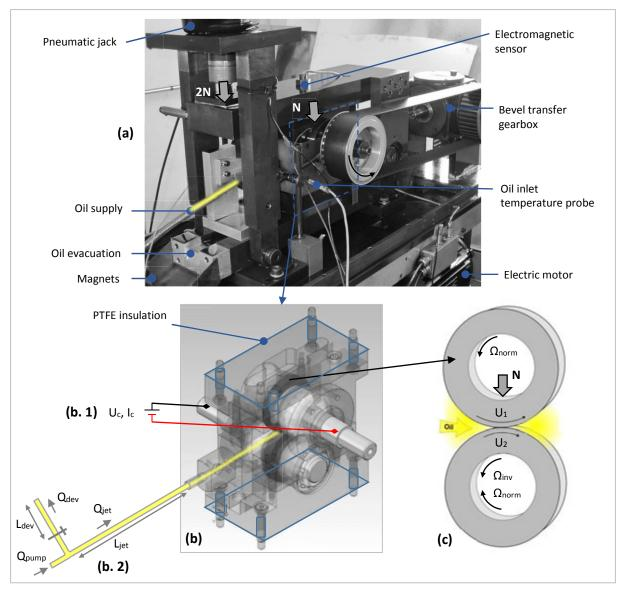
**Fig. 2.6**: LaMCoS TDM RCF test rig: (a) Main operational components and sensors; (b) Scheme of the roller mounting and optional specific installations to (1) impose an electric potential or current through the contact and to (2) regulate the jet oil flow Q<sub>jet</sub> by varying the relative pipe losses of an opened deviation; (c) Scheme of the twin-disc tribological contact parameters.
