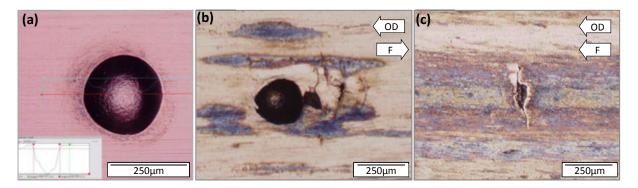
**Fig. 2.9**: LOM topview of disc raceways: (a) Artificial dent (50 Kg Rockwell indenter prior to testing); (b) Dent evolution after RCF testing on the follower surface (Appendix H ref TDM07\_07) (c) Typical surface initiated crack at the raceway border on the counter driver roller (Appendix H ref TDM07\_02\_I\_b).
