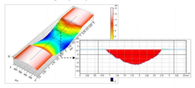
**Fig. 1.26**: Significant mild wear profile of a 100Cr6 driver roller after 106 cycles with important material removal measured by SENSOFAR PLu neox optical profilometer (Appendix H ref TDM09\_04).
