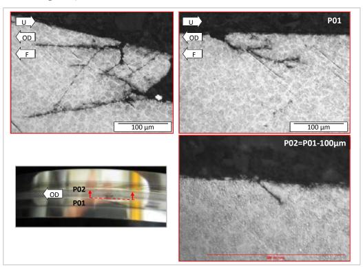
**Fig. 5.10**: TDM07\_01\_II cylindrical roller circumferential LOM (propagation phase, 3.0x10<sup>7</sup> cycles, 3.4 GPa, 30% SRR, driver, subsequent to microcrack pre-initiation with a dented counter-roller).
