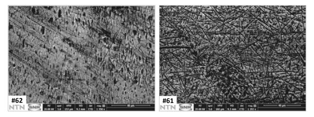
Fig. 4.6: SEM analyses of shiny ball from ACBB #62 and grey and matt ball from ACBB #61.
