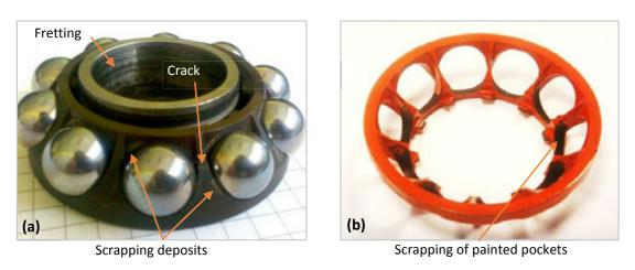
Fig. 4.4: (a) ACBB #40 standard cage after dismounting; (b) Specific ACBB short test under load case 4 with an orange painted oblong cage to locate the friction spots between the ball and the cage pockets.
