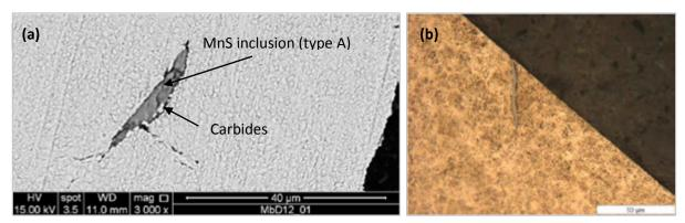
**Fig. 1.4**: (a) SEM image of a manganese sulfide (MnS) inclusion and (b) optical micrograph of another MnS emerging inclusions both found in a 100Cr6 D2 specimen.
