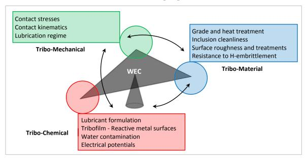
**Fig. 5.17**: WEC formation seems to require a subtle instable equilibrium between mechanical, material and chemical tribological phenomena all interacting.
