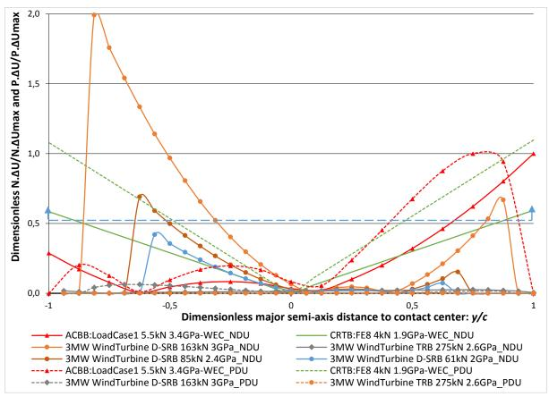
Fig. 5.6: Dimensionless sliding energetic criteria P.ΔU and N.ΔU for wind turbine D-SRB and TRB.
