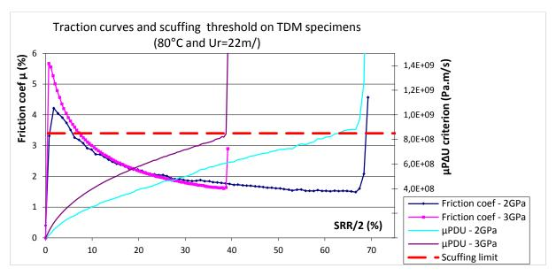
Fig. 2.7: Traction curves performed on the LaMCoS two-disc machine suggesting a  $\mu$ P $\Delta$ U threshold to establish a scuffing limit for future TDM RCF tests.
