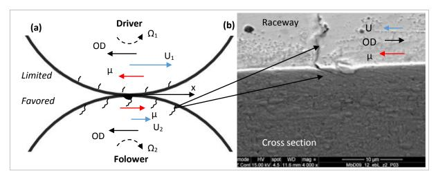
**Fig. 1.28**: (a) Scheme of microcrack development function of the contact kinematics and friction forces illustrating that surface microcrack propagation is favored on the follower surface; (b) SEM analysis of a 100Cr6 follower roller revealing a typical incipient surface microcrack (Appendix H ref TDM09\_12).
