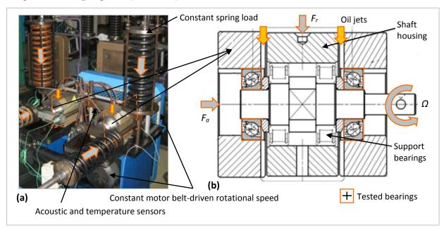
**Fig. 2.2**: (a) NTN-SNR Machine S endurance test rig; (b) Cross section of the ACBB mounting used in this study for WEC reproduction.
