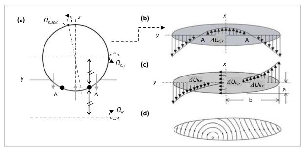
**Fig. 1.17**: (a) Heathcote conforming osculation with two lines of pure rolling in A; (b) ball contact sliding velocities in a radial loaded DGBB representing Heathcote slip; (c) ball contact sliding velocities in an ACBB accounting for transverse spinning motions; (d) overall sliding velocity lines in an ACBB without considering skidding (b, c, and d adapted from [17]).
