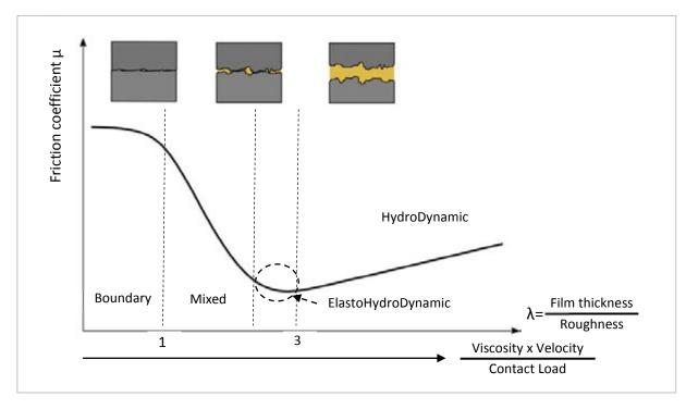
Fig. 1.19: Typical Stribeck curve representing the evolution the friction coefficient depending on the Hersey number or the  $\lambda$  film thickness ratio for the different lubrication regimes.
