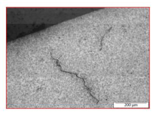
Fig. 3.8: LOM of an H-precharged TDM roller that failed prematurely after 2.5x106 cycles (TDM08\_03)
