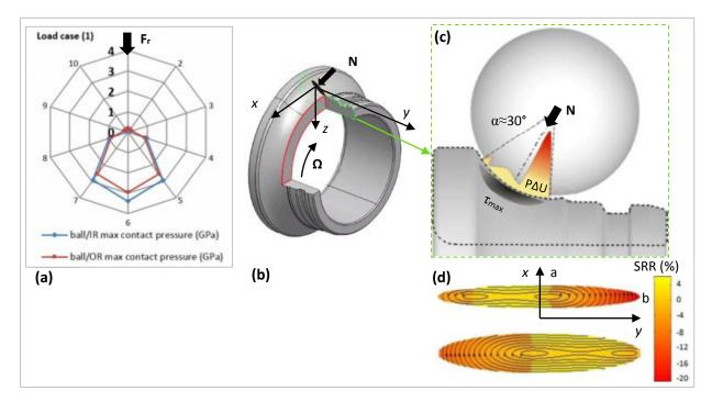
Fig. 2.4: (a) Contact pressure distribution in the ACBB; (b) Scheme of a cross sectioned IR of the tested ACBB; Schemes of the tribological parameters for the most loaded ball/IR contact in load case (1) with (b) illustrating the effective contact angle, subsurface shear stress and  $P\Delta U$  sliding energy criterion, and (c) the SRR lines in the IR and OR respective contact ellipsoid.
