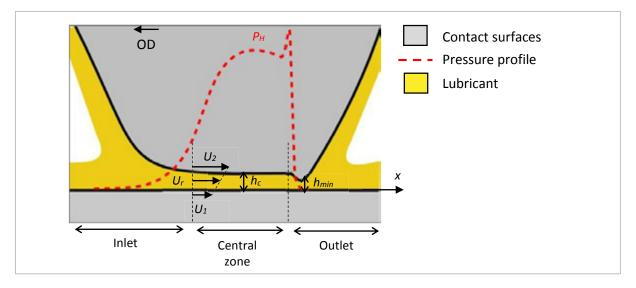
Fig. 1.20: Cross section of a typical EHL contact along the OD direction illustrating the contact pressure distribution and the film thickness profile (adapted from [66]).
