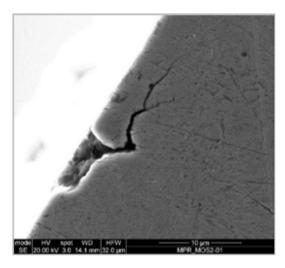
Fig. 1.29: SEM analysis of a typical incipient micropit obtained on a 100Cr6 roller.
