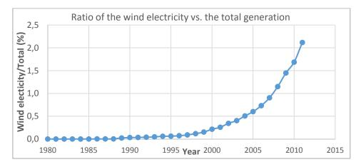
**Figure 3**: Zoom on the worldwide ratio of wind turbine electricity generation versus total generation from **Figure 1** (numerical data from [1]).
