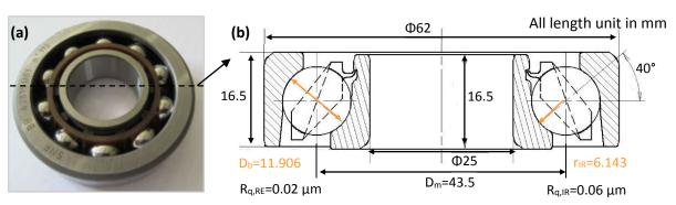
Fig. 2.3: (a) NTN-SNR ACBB with 10 balls and a polyamide cage used in this study; (b) Cross section of the ACBB with the mean diameter  $D_m$ , the ball diameter  $D_b$  and the IR curvature  $r_{IR}$
