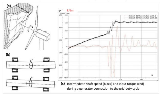
**Fig. 1.23**: Examples of wind turbine loadings affecting the REB tribological contacts: (a) wind fluctuations; (b) REB misalignments due shaft displacement (bottom) or bending (top); typical transient events in wind turbine gearboxes (from [9]).
