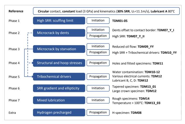
Fig. 5.9: General approach of WEC initiation and propagation on the TDM (details in Appendix H).
