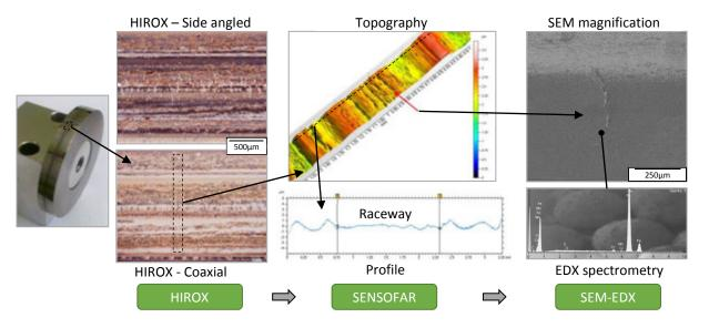
Fig. 2.15: Typical surface analyses of a TDM specimen: (1) HIROX LOM, (2) SENSOFAR raceway 3D topography and axial profile and (3) SEM-EDX and chemical spectroscopy in the vicinity of a microcrack.
