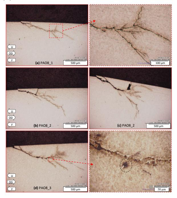
**Fig. 5.15**: Typical circumferential LOMs of TDM cylindrical follower raceway after RCF testing with various additive blends (**Table 5-2**) targeted to intersect with visible surface cracks.
