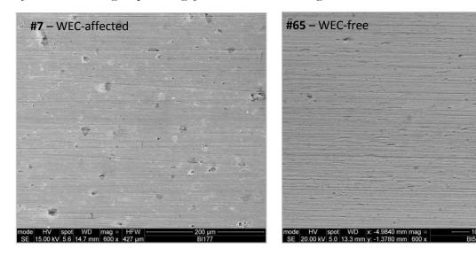
**Fig. 4.15**: Raceway topview of the contact edges of ACBB IR #7 and #65 where grinding marks remain (dents on IR#7 most probably due to debris from subsequent spalling).
