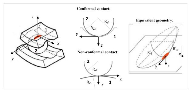
Fig. 1.8: Typical equivalent contact geometry of a raceway (1) – ball (2) elliptical contact.
