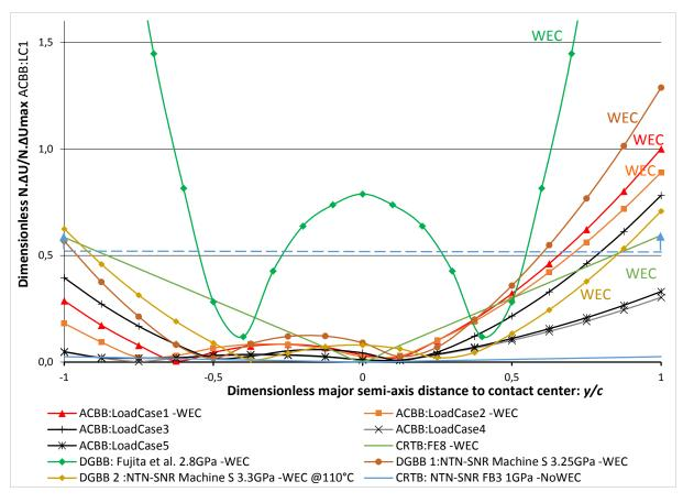
Fig. 5.7: Dimensionless sliding energetic criteria N.ΔU along the contact major axis for various REBs.
