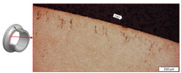
Fig. 5.4: Circumferential LOM of IR#61 with a high WEC density despite at high inclusion cleanliness.
