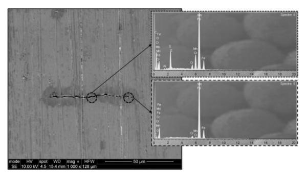
**Fig. 4.17**: SEM-EDX analysis of an axial microcrack observed in the contact edges of WEC-affected ACBB IR #8 revealing high manganese and sulfur contents in the crack vicinity suggesting the crack has been initiated due to the presence and/or dissolution of a type A inclusion near the surface [29].
