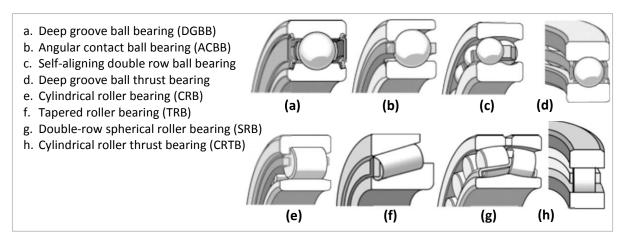
Fig. 1.2: Typical examples of REB types (courtesy of SKF).
