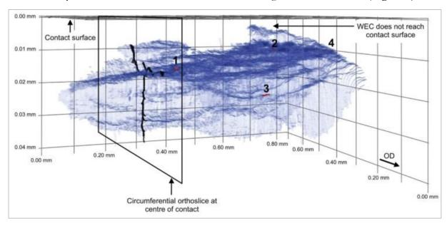
**Fig. 1.43**: 3D mapping of a WEC network reconstructed by manual serial-sectioning and segmentation techniques (in red, inclusion interacting with the cracks) [188].
