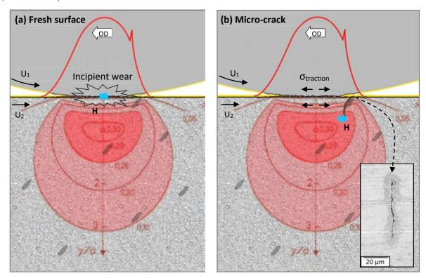
**Fig. 4.16**: Scheme of WEC initiation mechanisms by formation of nascent steel surfaces either (a) directly at the surface by incipient wear and/or heterogenous and patchy tribofilms, either (b) indirectly by the opening of incipient surface microcracks allowing lubricant contact with nascent flanks.
