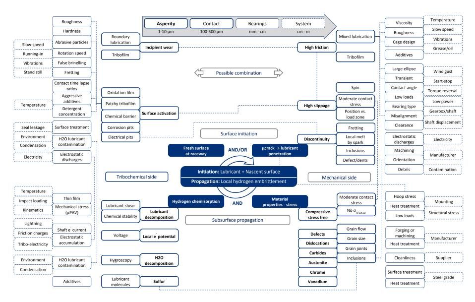
Fig. 5.2: WEC initiation and propagation root cause analysis with some various influences of multiple drivers from tribo to macro-scales (Appendix I, J, K, L).
