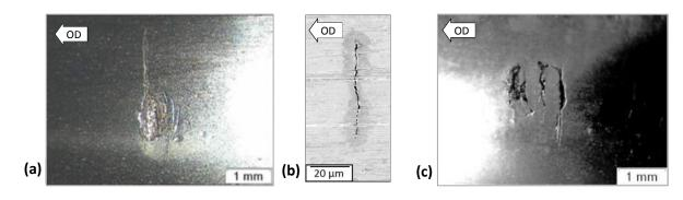
Fig. 3.3: Examples of axial spalls on ACBB IR: (a) neutral #7, (b) neutral unspalled #8, (c) H-precharged #28.
