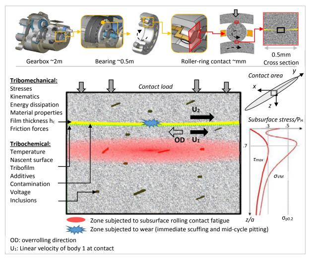
**Fig. 1.7**: Schematic overview of a tribological contact in a REB considering both tribomechanical and tribochemical parameters affecting the life time before surface or subsurface failure.
