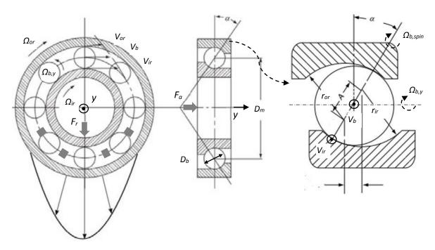
Fig. 1.16: Basic rolling kinematics of an angular contact ball bearing under a typical load illustrating the different velocities, contact angle, osculation and dynamic effects of the cage (adapted from [17]).
