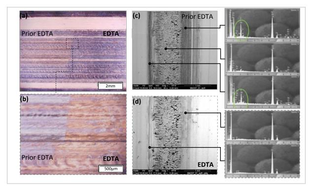
Fig. 2.18: Efficiency of EDTA to remove tribofilm deposits (1) illustrated by the clear frontier between the untouched left side and the EDTA tissue-cleaned right side of a TDM raceway observed on (a) side-angled LOM and (b) co-axial LOM close-up (Appendix H ref TDM12\_07) and (2) confirmed by SEM-EDX analysis on a different TDM raceway (Appendix H ref TDM07\_01\_II) (c) prior and (d) after EDTA ultrasound bath rising where no more traces of sulfur and phosphorus remain.
