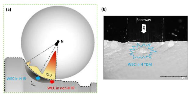
**Fig. 3.11**: (a) Scheme illustrating the WEC location versus the contact area in non-H-precharged and H-precharged ACBB IR; (b) Three-quarter view of the H-precharged (H) TDM roller fractograph revealing a WEC at the center of contact below the raceway (cf. **Fig. 3.5**).
