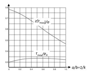
Fig. 1.10: Tresca shear stress  $\tau_{max}$  and respective depth  $z(\tau_{max})$  at x=0 function ratio of the degree of ellipticity: case of a line contact for a/b=0 with  $\tau_{max}=0.3P_H$  at z=0.78a; case of a circular contact for a/b=1 with  $\tau_{max}=0.31P_H$  at z=0.48a (plot adapted from [17]).
