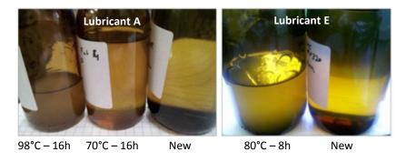
Fig. 2.13: Visual aspect of lubricant samples after environmental artificial water ingress.
