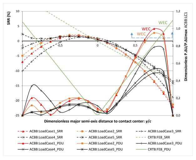
Fig. 4.13: Slide to roll ratio (SRR) and dimensionless sliding energetic criteria P.ΔU along the contact major axis transverse to rolling motion for (1) the CRTB FE8 configuration (green) and for (2) WEC-free (black) and WEC-affected (orange-red) ACBB load cases (Fig. 2.4 and Table 2-2). A suggested P.ΔU threshold for WEC development is represented by the blue dashed lined and arrows. Similar P.ΔU plot accounting for scaled contact major axis available in Appendix G (a).
