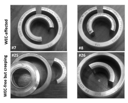
Fig. 4.7: ACBB ring flanges aspect after RCF tests.
