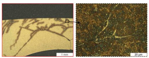
**Fig. 5.14**: Circumferential LOM of TDM11\_00 cylindrical roller with holes inducing additional structural stresses (3.5 GPa, 7% SRR, driver, lubricant PAO8 at 80°C) (cracks are emphasized due to etchant trap in their vicinity).
