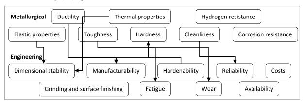
**Fig. 1.3**: Typical metallurgical and engineering properties required for bearing steels and examples of interdependencies
