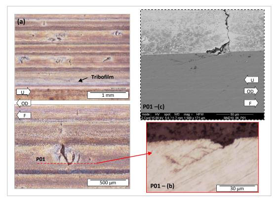
**Fig. 5.11:** TDM10\_06 crowned roller typical raceway topview (a), circumferential LOM (b) and SEM <sup>3</sup>/<sub>4</sub> view of the circumferential cross section and raceway microcrack revealing some crack ramifications opposite to OD without adjacent WEA (propagation phase, 2.9x10<sup>7</sup> cycles, 3 GPa, 30% SRR, driver, 85°C water contamination, and regular EDTA cleaning of the tribofilm, subsequent to microcrack pre-initiation with a dented counter-roller).
