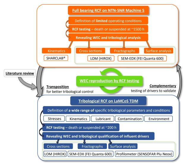
Fig. 2.1: Overall methodology and experimental procedures led for a tribological analysis of WECs.
