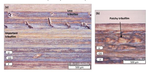
Fig. 5.13: Typical TDM13\_02 raceway topview of (a) cylindrical follower roller and (b) crowned driver roller (2.5x 10<sup>7</sup> cycles, 3 GPa, 30% SRR, lubricant B at 85°C, water contamination and 50mA).
