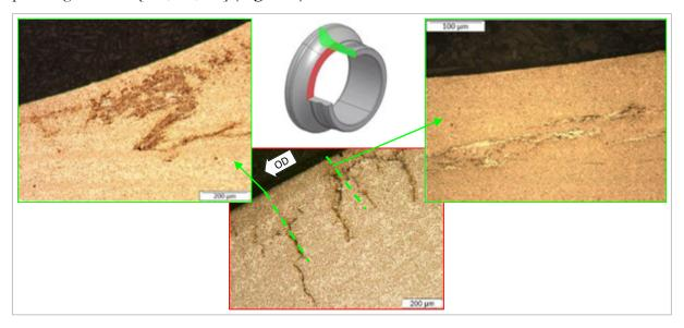
**Fig. 3.6**: Axial and circumferential LOMs of the neutral IR #7 revealing different morphological layouts of WECs and suggesting a possible interpretation of the different WEC aspects on the two axial LOMs.
