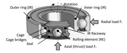
Fig. 1.1: Rolling Element Bearing (REB) typical structure, components and speeds (courtesy of SKF).
