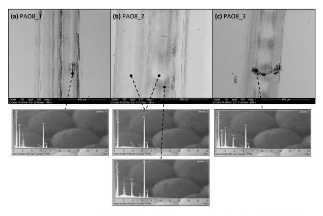
**Fig. 5.16**: SEM-EDX analysis on TDM raceways after RCF testing with various additive blends (**Table 5-2**) revealing different tribofilm composition.
