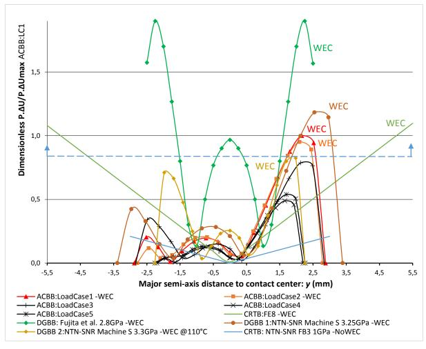
P being the local contact pressure and  $\triangle U$  the local slip velocity. The dashed blue line represents a possible threshold for WEC formation.
