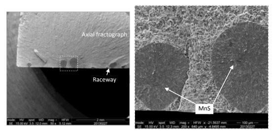
**Fig. 3.2**: Example of transgranular fracture halos around MnS inclusion on a TDM roller fractograph 96 hours after artificial hydrogen charging.
