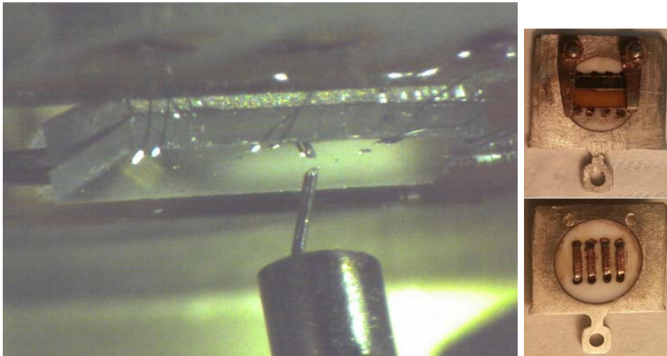
Figure 3.12: Left: Picture of the NbN sample where one can see the Al-bonding used for transport measurements. Right: Top and bottom views of the modified "OMICRON" sample holder. Contacts are made through copper ribbons and a fixation system for the sample has been created.
