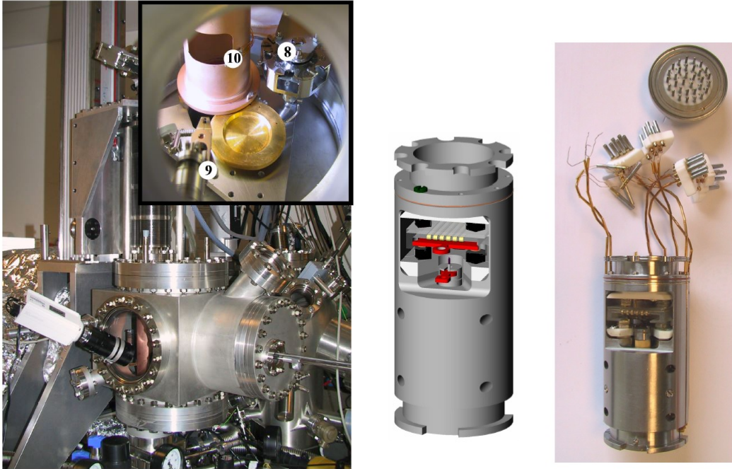
Figure 3.10: Left: External and internal views of the STM chamber: (8) Tips and samples carousel storage, (9) Wobble-stick, (10) Copper screen shielding the STM head. Right: Sketch and picture of the M3 STM head. In red are the tip holder (below) and the sample holder (above). The contact springs for in-situ transport measurements are seen in yellow, above the sample holder.
