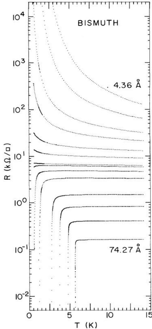
Figure 1.2: Resistance evolution as a function of temperature for different thin film thicknesses of Bi on Ge extracted from [HLG89]. This is the characteristic behavior of superconductor-insulator transition in homogeneous systems.
