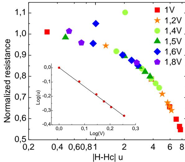
Figure 4.6: Resistance as a function of the scaling variable  $|H-H_c|u$  for different voltage drops across the sample at a temperature of 1.9K. We adjust  $u = E^{1/\nu(z+1)}$  in order to obtain the best collapse of the data. Inset: log-log plot of the parameter  $u$  versus voltage used to determine the value of  $\nu(z+1)$ .
