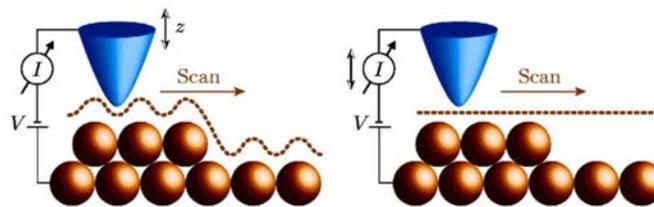
Figure 3.2: *Topographic STM modes. On the left: constant current imaging, distance  $z$  is adjusted to maintain the current constant. On the right: constant height imaging, the current  $I$  is changing.*
