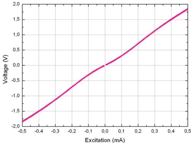
Figure 3.13:  $I(V)$  curve measured at 1.8K with PPMS by passing an AC current from -0.5mA to 0.5mA through a NbN 2.16nm thick sample. It is not possible to distinguish between the increasing or decreasing current. No hysteresis is observed. A non linearity can be seen because the measurement has been performed on a superconducting sample.
