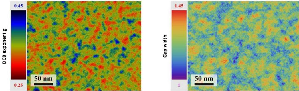
Figure 6.13: *Comparison between the dynamical Coulomb blockade exponent map (on the left) and the superconducting gap map (on the right) measured in the same area. The red and blue patches of the dynamical Coulomb blockade  $g$  map correlate directly with the red (larger gap) and blue regions (lower gap) of the studied area. This shows a direct link between the local disorder potential combined to electron-electron interactions and the local gap values.*
