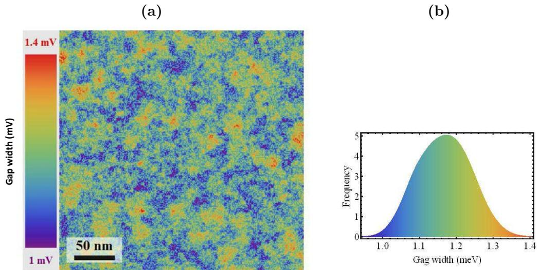
Figure 6.5: (a) Superconducting gap map corresponding to the conductance map in figure 6.4 and showing the spatial variations of the gap width. The gap  $\Delta$  is defined as the peak-to-peak value. (b) Histogramm of the frequency of the gap width, the mean value is  $1.2\text{meV}$ .
