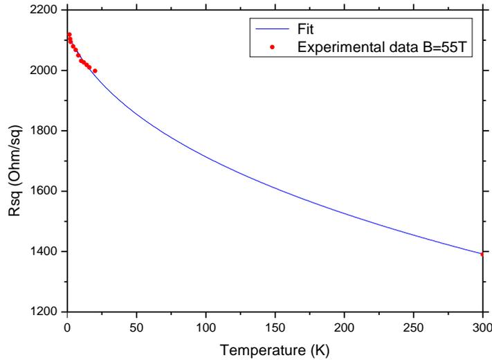
Figure 4.7: Fit of the experimental data measured under a magnetic field of 55T. The law used to fit the normal state resistance is  $R_N(T) = 3,52L_T^3 + 12,1L_T + 2112,62$ . It has been determined from the experimental data without magnetic field but one can see that it is fully consistent with the normal state data measured at 55T.
