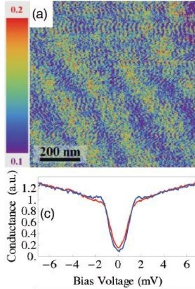
Figure 1.19: *Spatial inhomogeneities of the superconducting gap measured at 2K on a 2.16nm thick NbN sample by tunneling spectroscopy. The red spectra are representative of the red area of the conductance map and the blue one of the blue area of the conductance map. We observed that very small coherence peaks are present only in the blue regions.*
