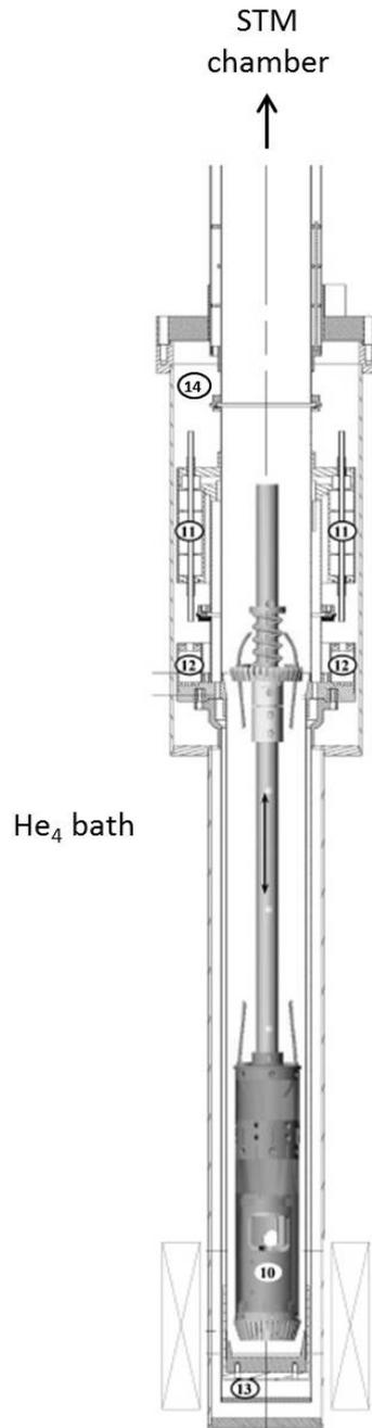
Figure 3.11: *M3 cryogenic system sketch. The STM Head (10) is located at the end of the rod used to move it in the UHV insert. The cone at its extremity is pressed on the  $^3\text{He}$  socket (13) which is in direct thermal contact with the volume where  $^3\text{He}$  is condensed. The  $^3\text{He}$  sorption pump is located on (11), under the 1K pot (12). In (14) is located the Internal Vacuum Can (IVC) used to isolate the helium 4 bath from the  $^3\text{He}$  cooling system.*
