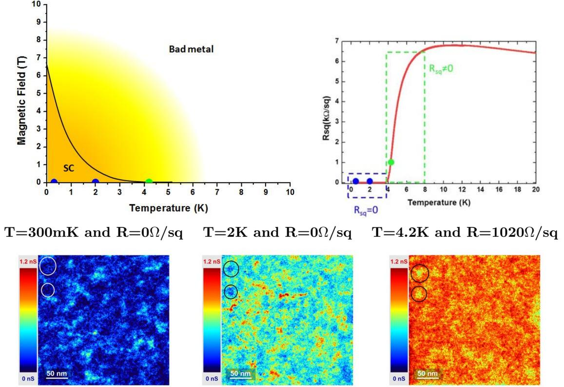
Figure 1.21: On the first line is represented the phase diagram with the studied points as a function of temperature. In blue are the points where we measured zero resistance, the sample is in the superconducting state. In green are the point where the resistance reach a finite value. They are plotted on the resistance curve. On the second line are the conductance map measured over the same sample area with increasing the temperature.
