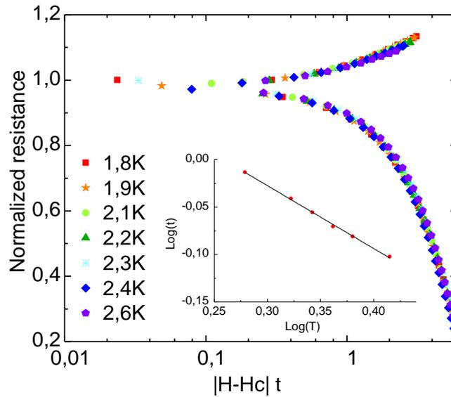
Figure 4.4: Resistance per square as a function of the scaling variable  $|H-H_c|t$  for different temperatures and a critical magnetic field of 10.7T. We adjust  $t = T^{1/\nu z}$  in order to obtain the best collapse of the data. Inset: log-log plot of the parameter  $t$  versus temperature used to determine value of  $\nu z$ .
