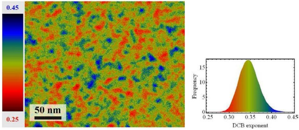
Figure 6.12: *Left: Map of the dynamical Coulomb blockade exponent extracted from the fit of all spectra measured on the area of figure 6.1 using the formula:  $dI/dV \sim V^2/g$ . Right: Histogram of the frequency of the value of the dynamical Coulomb blockade (DCB) exponent. The mean value is 0.35.*
