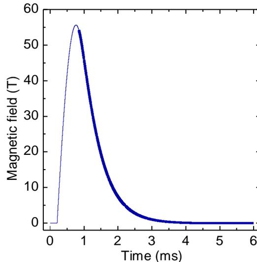
Figure 4.11: *Evolution of the magnetic field amplitude as a function of time for a ramp from  $0\text{T}$  to  $55\text{T}$ . The acquisition time is  $6\text{ms}$  but increasing the magnetic field lasts only  $1\text{ms}$ .*
