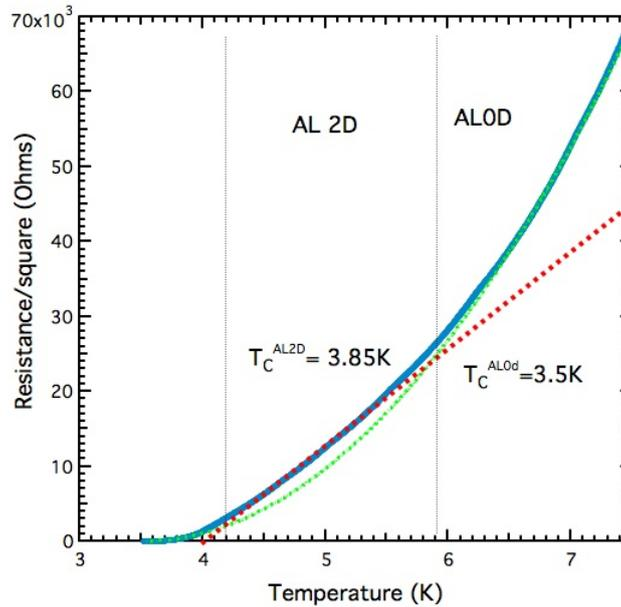
Figure 4.10: *Extracted paraconductivity for sample  $A_2$ . In blue are the experimental data, in green is the AL0D fit and in red is the AL2D fit. A cross-over between the two regime is observed very close to  $T_c$ .*
