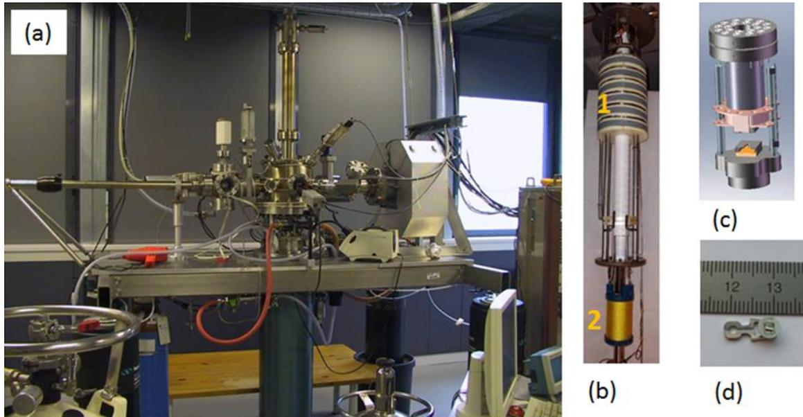
Figure 3.4: (a) General view of the M2 experimental setup. (b) Cryogenic insert of the  $^4\text{He}$  cryostat. In (1) are the new cryogenic screens and in (2) is the new superconducting magnet. (c) Modified STM head. (d) New sample holder with a  $\text{NbSe}_2$  sample.
