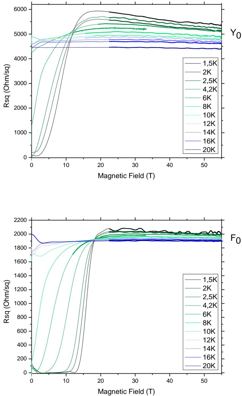
Figure 4.12: *Magnetoresistance of two samples. On the top:  $Y_0$  and on the bottom:  $F_0$ . The magnetic field is increased from 0T to 55T and the temperature varied from 1.5K to 20K. For sample  $Y_0$ , a small peak appears and the magnetoresistance is then negative. The thicker sample  $F_0$  is less sensible to the applied magnetic field. In both cases, a crossing point is clearly visible.*
