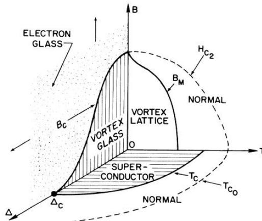
Figure 1.5: Schematic phase diagram drawn by M. Fisher and extracted from [Fis90].  $\Delta$  is the disorder,  $T$  the temperature and  $B$  the magnetic field. These three axis represent the three different ways to induce the superconductor-insulator transition.
