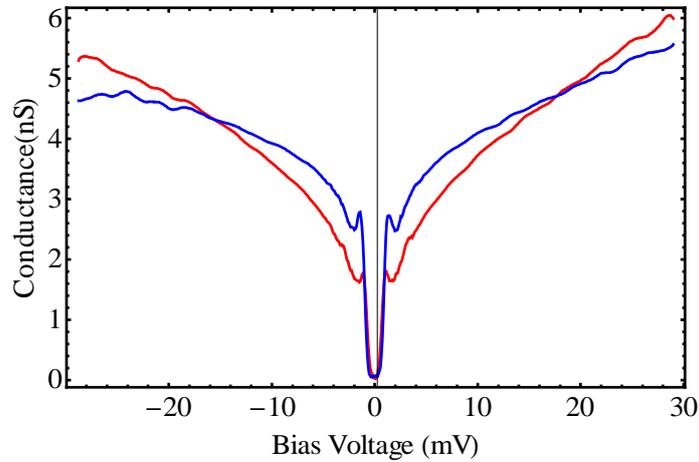
Figure 6.11:  $dI/dV$  tunneling spectroscopy measurements of the local density of states over an energy scale about 10-15 times  $\Delta$  :  $[-30\text{mV}; +30\text{mV}]$  and at  $T=300\text{mK}$  and  $B=0T$ . The observed V-shape background is characteristic of the Altshuler-Aronov effect that describes bad metal films.
