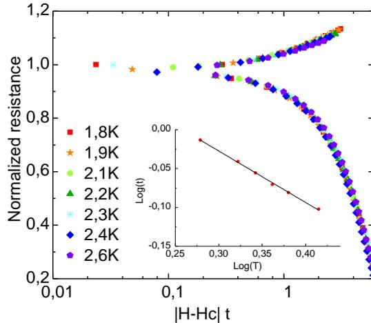
Figure 1.20: Resistance per square as a function of the scaling variable  $|H-H_c|t$  for different temperatures at a magnetic field of  $10.7T$ . We adjusted  $t = T^{1/\nu z}$  in order to obtain the best collapse of the data. Inset: log-log plot of the parameter  $t$  versus temperature used to determine value of  $\nu z$ .
