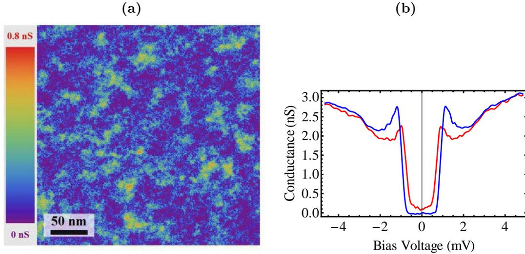
Figure 6.4: (a) Tunneling spectroscopy  $dI/dV(V=0)$  conductance map measured at  $300\text{mK}$  and in zero magnetic field. The color code represents the spatial variations of the  $dI/dV$  signal. Spectral inhomogeneities are visible, attesting for an emergent granularity. (b) Individual tunneling  $dI/dV$  spectra representative of the inhomogeneities observed in the conductance map. Blue spectra is measured in a blue zone and red spectra in a red/yellow one.
