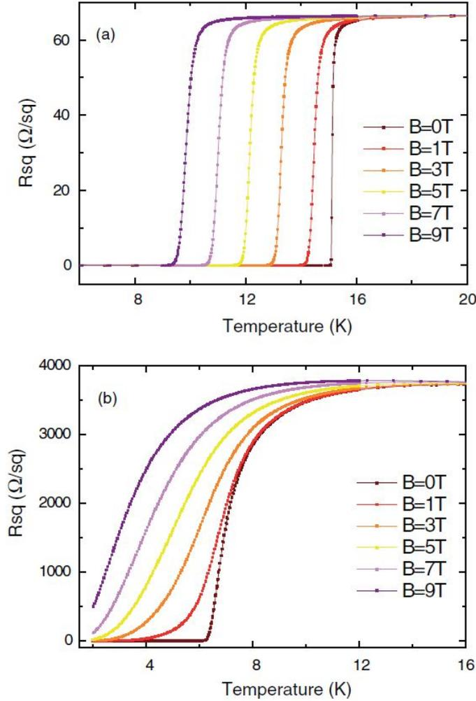
Figure 5.6: *Square resistance versus temperature for different magnetic fields in the range 0-9T for (a) 17.5nm thick NbN film with a  $T_c$  of 15K and (b) 2.16nm thick NbN film with a  $T_c$  of 6.5K*
