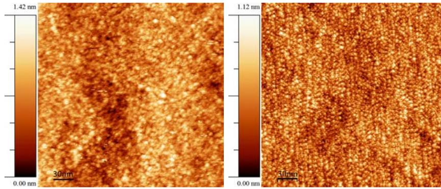
Figure 3.8: *STM images 300nm\*300nm before (left) and after (right) ionic bombardment on a NbN sample. In both cases, grains are observed. On the image after ionic sputtering, grains appear smaller. It is a multiple tip effect.*
