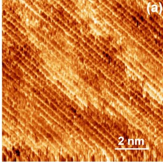
Figure 1.10: Topographic image of the TiN film extracted from [KSR<sup>+</sup>14b] and showing the atomic resolution on a  $10\text{nm} \times 10\text{nm}$  area.
