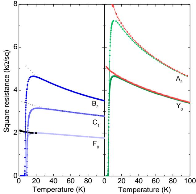
Figure 4.8: *Blue and green dots: Square resistance under 0T as a function of temperature for samples A<sub>2</sub>, B<sub>2</sub>, C<sub>1</sub>, F<sub>0</sub> and Y<sub>0</sub>. Red triangles: resistance under 14T perpendicular magnetic field for sample A<sub>2</sub> and Y<sub>0</sub>. Dotted line: extrapolated normal state resistance for samples B<sub>2</sub>, C<sub>1</sub> and the normal state measured under 55T for F<sub>0</sub>.*
