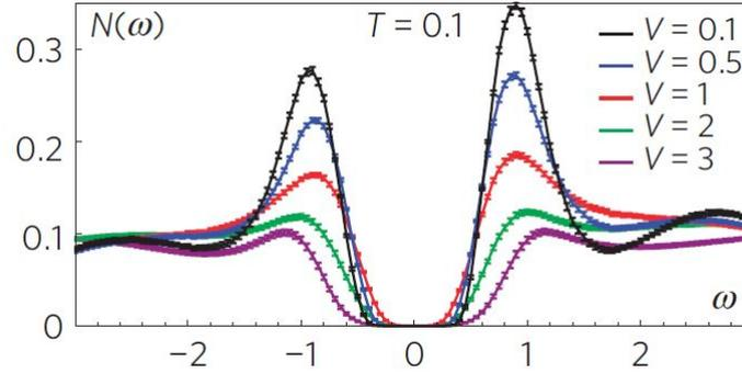
Figure 1.8: *Evolution of the local density of state  $N(\omega)$  as a function of the disorder and at a fixed temperature extracted from [BLRT11]. A hard gap persists in the insulating while the coherence peaks exists only in the superconducting state.*
