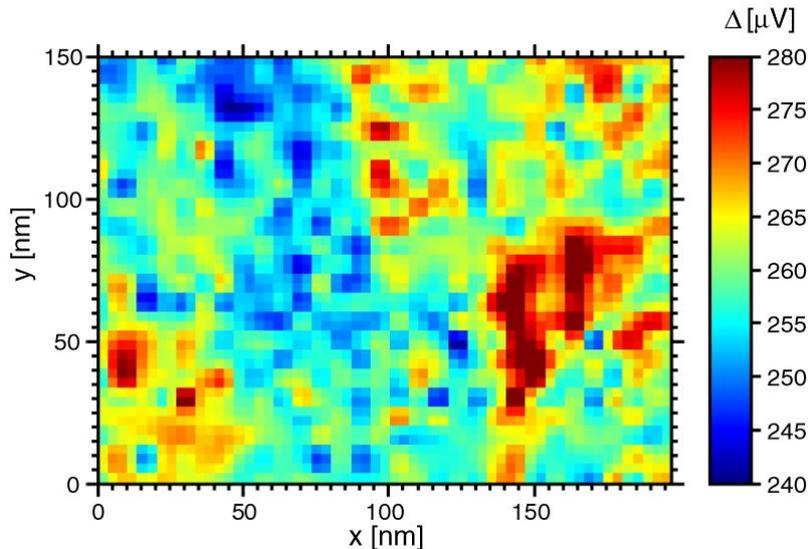
Figure 1.9: *Color map of the spatial inhomogeneities of the gap measured by STS in TiN and extracted from [SCB<sup>+</sup>08].*
