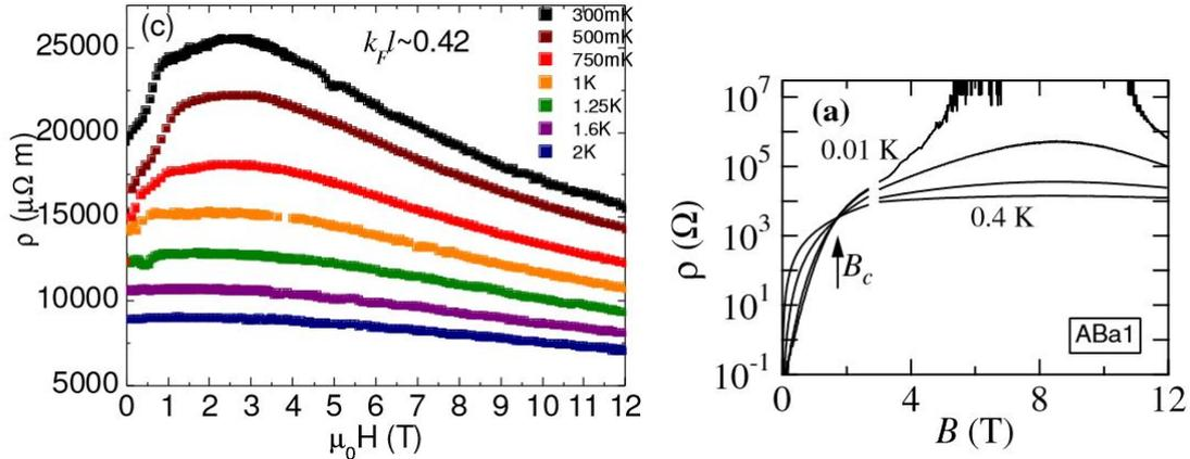
Figure 1.16: *Left: Magnetoresistance peak measured on epitaxial NbN film extracted from [CMK<sup>+</sup>12]. Right: Magnetoresistance peak measured on InO film extracted from [SEJ<sup>+</sup>05]. In NbN, the maximum resistance reaches is about 25000 $\mu\Omega\cdot m$  while in Ino it is more than  $10^7\Omega$ . This point highlights that the two materials have a completely different behavior under magnetic field.*
