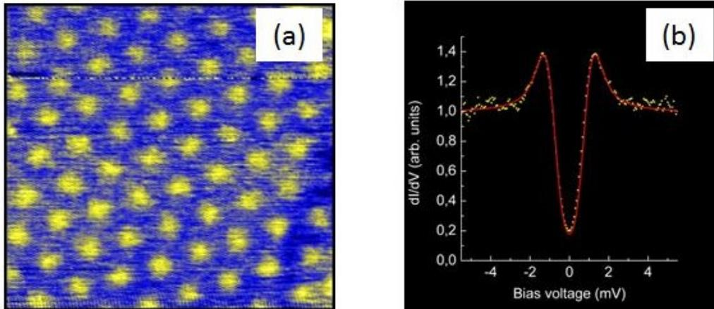
Figure 3.6: Operating test of the experimental setup M2. (a) Vortex lattice in NbSe<sub>2</sub> (200nm x 200nm,  $B=4T$ ,  $T=2K$ ). Vortices correspond to the yellow circles and the blue area is superconducting. (b)  $dI/dV$  spectra in NbSe<sub>2</sub> without magnetic field and at  $T=2K$ . In yellow are the experimental data that can be well fitted by the BCS theory in red.
