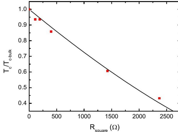
Figure 5.7: Dependence of  $T_c/T_{c\text{-bulk}}$ , the superconducting critical temperature normalized by the bulk one, as a function of their square resistance  $R_{\text{sq}}$  in the normal state at 40K. Red squares are experimental data extracted from resistivity measurements. The black line is the fit by the Finkelstein law.
