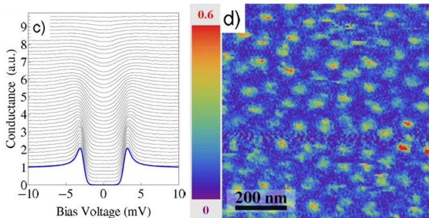
Figure 5.2: *c) Evolution of the tunneling conductance spectra with the temperature from  $2.3\text{K}$  to  $15\text{K}$  (vertically shifted for clarity). The bottom blue line is the BCS fit at  $T=2.3\text{K}$ ; d)  $dI/dV$  conductance map at zero bias under magnetic field  $B=1\text{T}$ . It reveals a disordered vortex lattice.*
