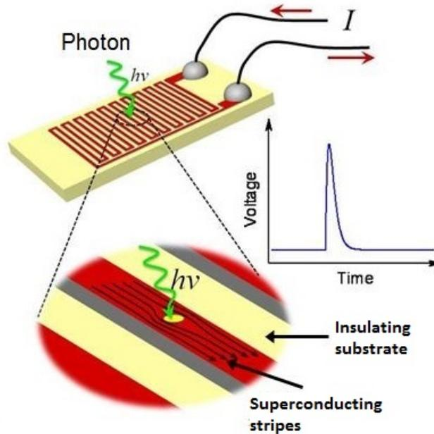
Figure 7.1: *Schematic view of the Superconducting Nano-Stripe Photon Detector operating mode. When a photon is absorbed on the wire, a resistive hotspot is formed and a voltage pulse can be detected at both ends of the meander.*
