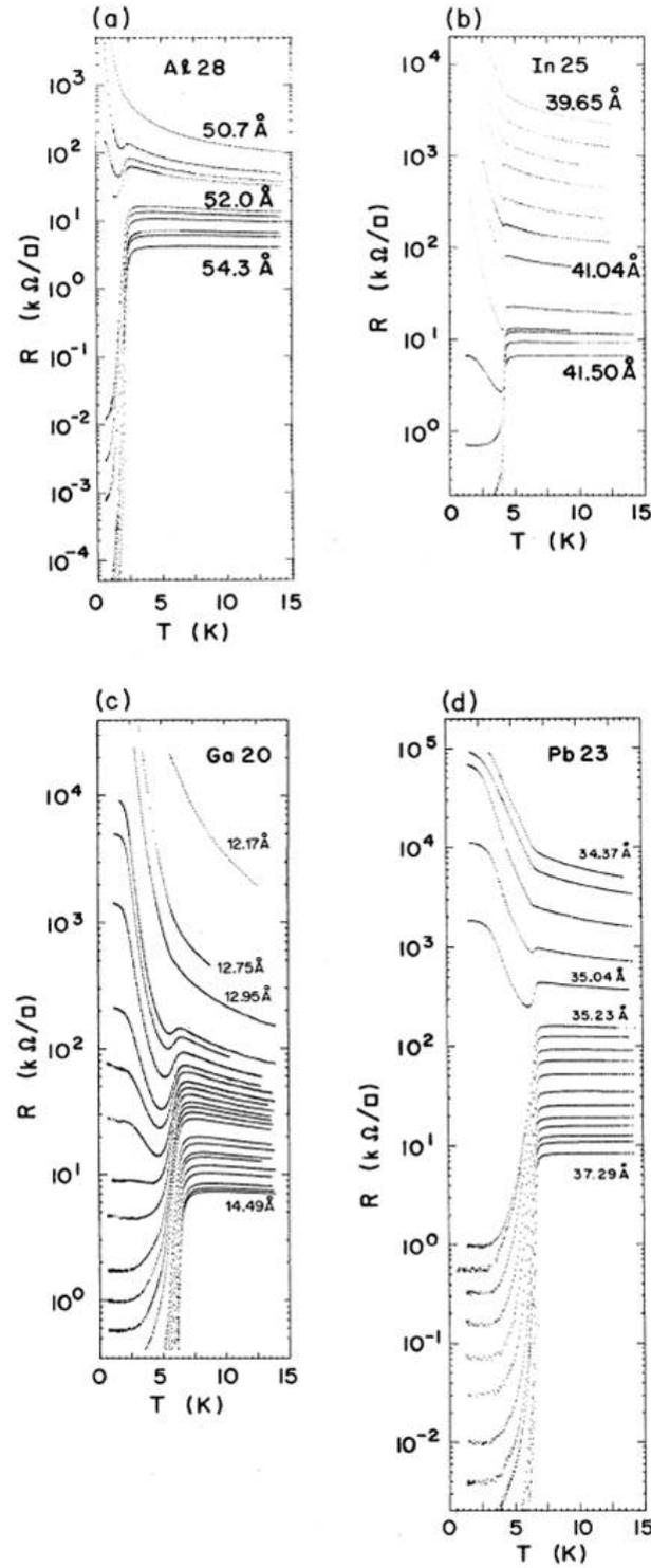
Figure 1.1: Evolution of  $R(T)$  curves for so-called granular superconductors a) Al, b) In, c) Ga and d) Pb as a function of film thickness. In both cases, a superconductor-insulator transition is observed. (Extracted from [JHOG89].)
