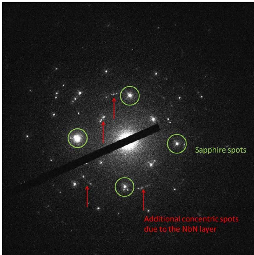
Figure 2.3: *Electronic diffraction pattern obtained by TEM on a 2.33nm thick NbN sample. Concentric circles (red arrows) are visible in addition to the spots due to the sapphire substrate (green circles). These features are characteristic of polycrystalline samples.*
