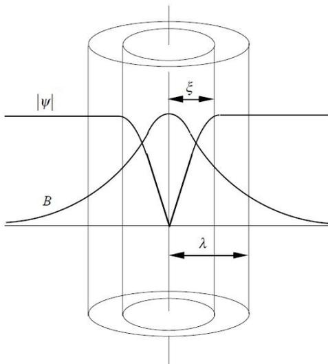
Figure 1.4: Shape of the magnetic field  $B$  and the density of Cooper pairs  $|\psi|$  close to a vortex.  $\xi$  is the coherence length that represent the size of the vortex core.  $\lambda$  is the penetration length which correspond to the size over which the magnetic field is screened by the super-current rotating around the vortex.
