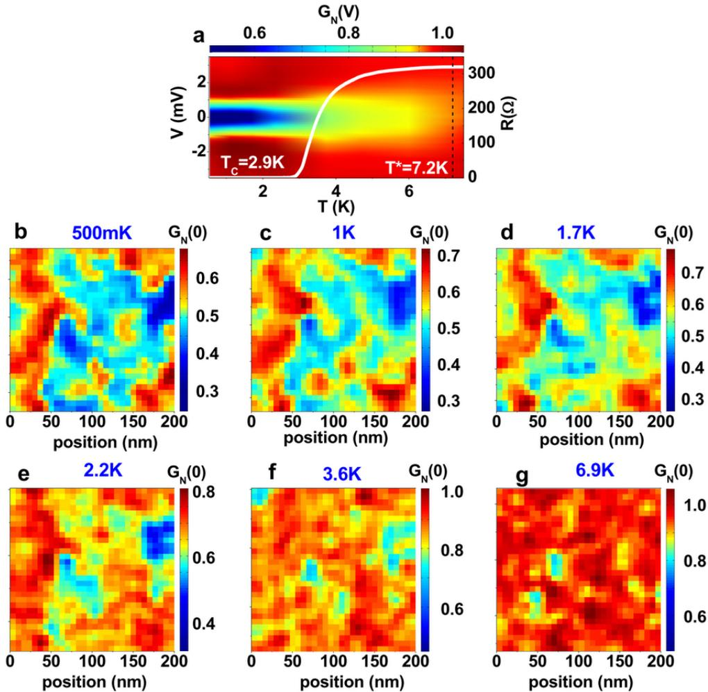
Figure 1.11: *Evolution of the superconducting inhomogeneities over the sample area as a function of temperature in epitaxial NbN film with a  $T_c$  of 2.9K extracted from [KDG<sup>+</sup>13].*
