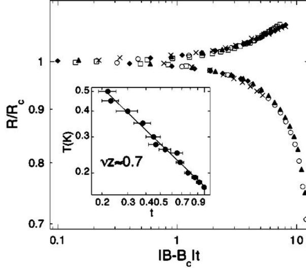
Figure 1.15: Temperature scaling law analysis of the magnetic field tuned superconductor-insulator transition in Bi thin film extracted from [MCM<sup>+</sup>99]. The critical exponents are found to be equal to  $\nu z = 0.7$ .
