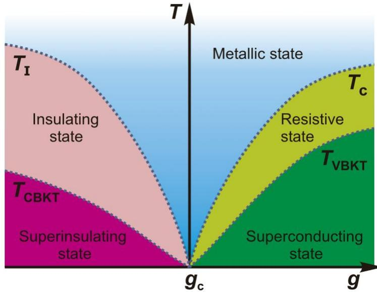
Figure 1.14: *Phase diagram  $T$ - $g$  of the superinsulator-superconductor transition extracted from [BV13].  $T$  is the temperature and  $g$  is the critical parameter. In the Josephson junction arrays,  $g$  represent the ratio of Josephson coupling and charging energy  $g = E_J/E_C$  where  $E_J$  is the Josephson coupling energy of the two adjacent superconducting islands and  $E_C$  is the energy cost to transfer a Cooper pair between the neighbouring islands.*
