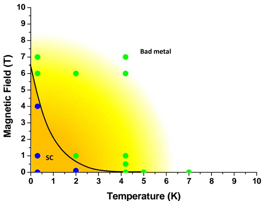
Figure 6.3:  $B$ - $T$  phase diagram representing point corresponding to all situation studied by STS. The transition between the superconducting state (SC) and the bad metal state is induced by varying the temperature or the magnetic field. In blue are the points corresponding to the superconducting state, when the measured resistance is truly zero, and in green are the points for which the resistance of the film is different from zero.
