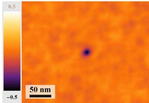
Figure 6.14: *Cross-correlation map between the dynamical Coulomb blockade exponent map and the superconducting gap map shown in figure 6.13. The black disk at the center of the image indicates that there is a strong correlation between the two map. The value obtained is -0.56 meaning that there is a strong ant-correlation between the dynamical Coulomb blockade exponent and the gap width : the smaller is the exponent, the larger is the local gap value.*
