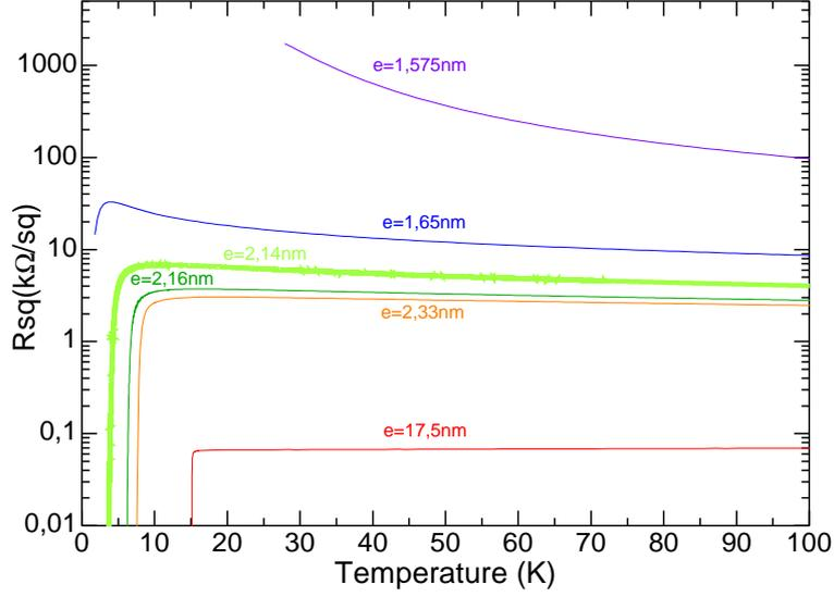
Figure 1.18: *Square resistance evolution as a function of temperature. The superconductor-insulator transition is induced by decreasing the film thickness. It has a behavior similar to what is typically observed in homogeneous thin films.*
