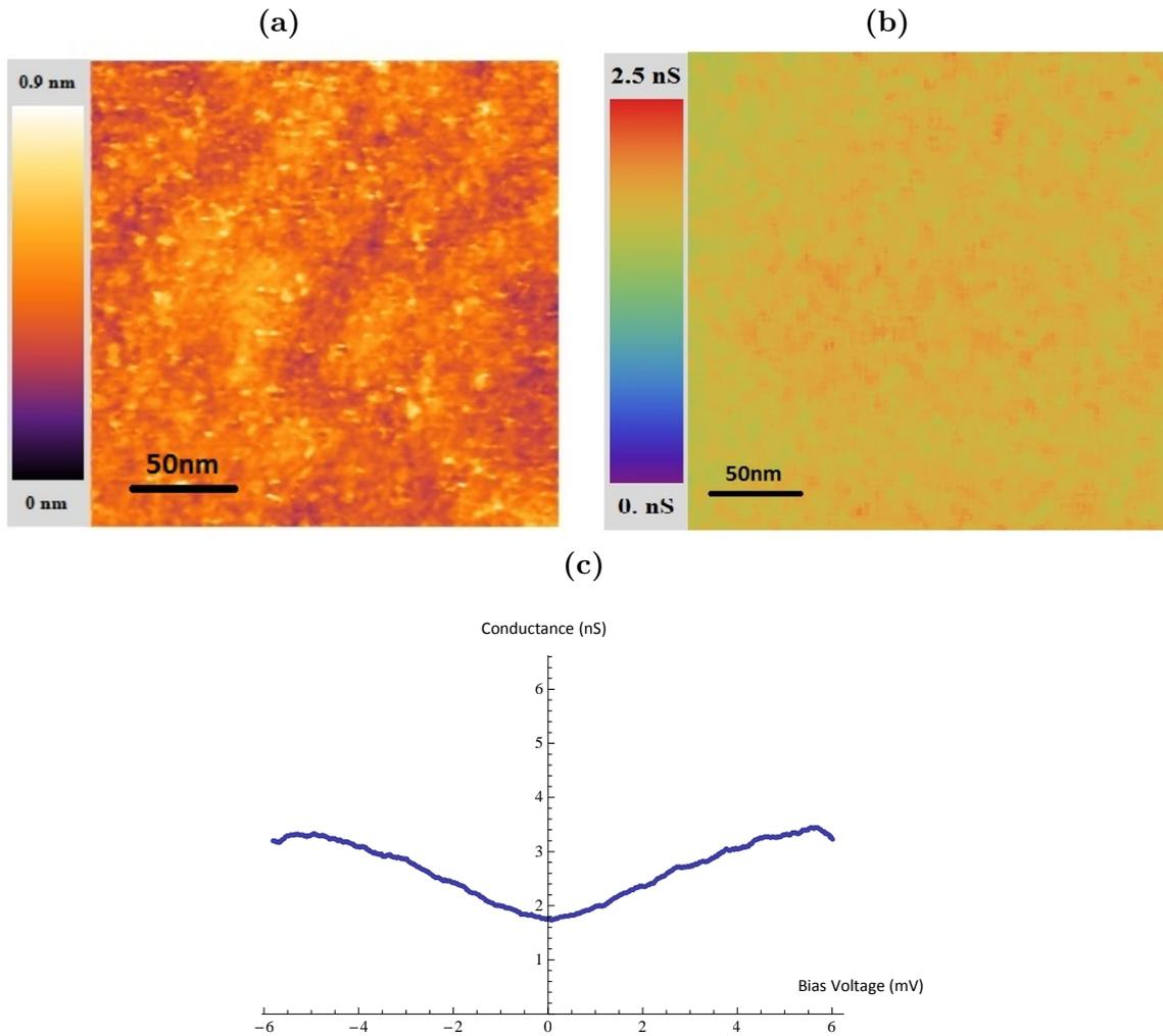
Figure 6.7: a) *STM topography image measured at 7K. The typical nanocrystallites composing the samples are visible.* b) *Corresponding zero bias conductance map measured at 7K. It becomes completely homogeneous when increasing the temperature well above  $T_c$ .* c) *Characteristic spectrum measured on this conductance map.*
