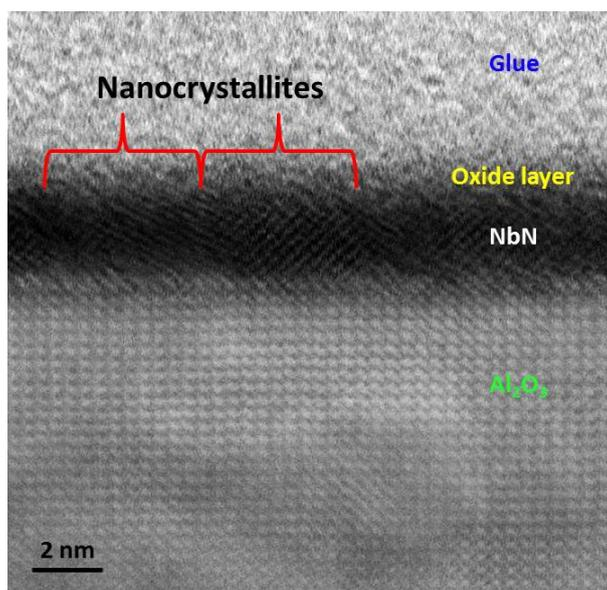
Figure 2.4: TEM image done on a 2.33nm thick NbN sample in cross section view. Nanocrystallites of few nanometers are visible. The oxide layer has been detected by a chemical analysis but is too thin to be observed.
