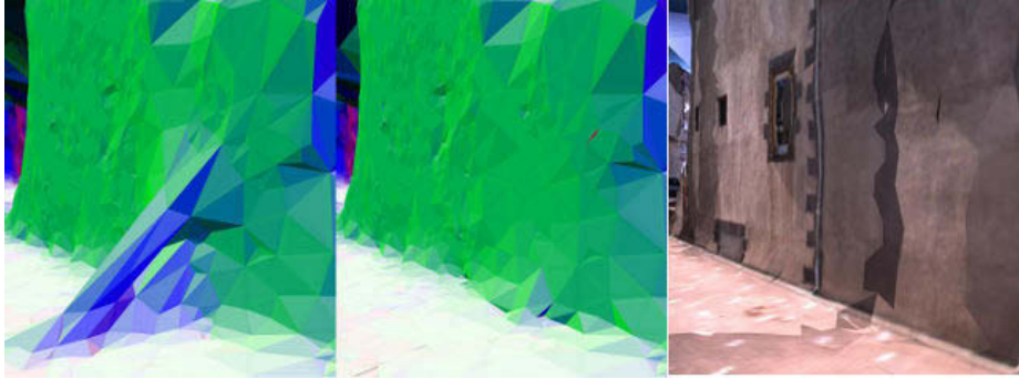
Figure VI.1: A visual artifact example. On the left image the surface contains an easily visible visual artifact. On the central image the visual artifacts was removed from the surface. Colors encode the triangles normals. On the right image the visual artifact is removed and the surface is textured.
