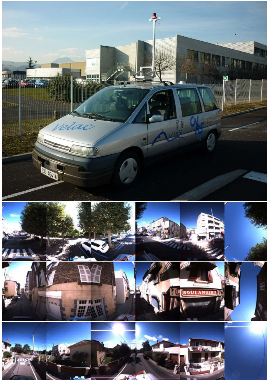
Figure V.2: The top image shows the experimental vehicle equipped with the Ladybug omnidirectional camera used to acquire the aubiere real world sequence. The three following images shows some representative pictures.
