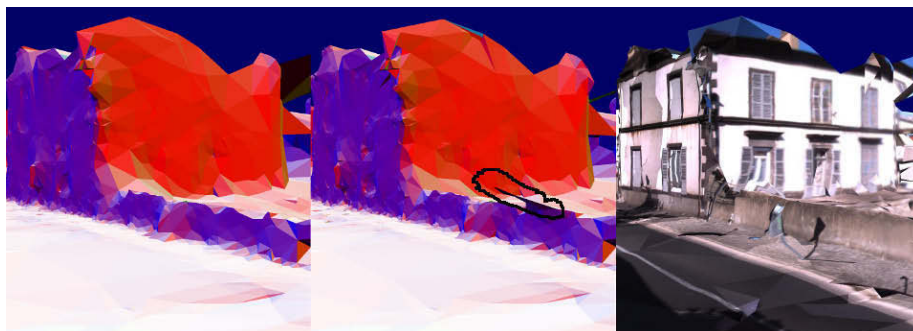
(c) Example of a inside peak. Left image shows the surface computed with the peak removal enabled. The central image shows the surface without peak removal, the artifact is encircled by a black trait. The right image shows the textured surface for reference. The illustrations shows the final surface computed by processing the aubiere sequence (see chapter V). The colors encode the triangles normals.
