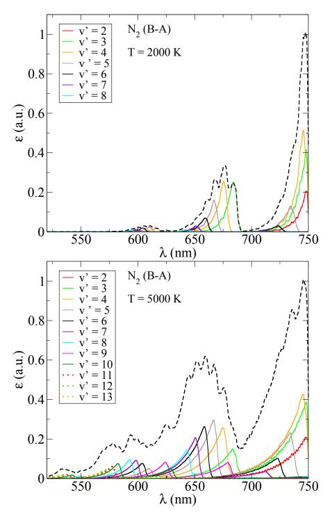
Figure 7.20.: Equilibrium synthetic spectrum (black) and corresponding vibrational bands contribution at  $2000~{\rm K}$  (top) and  $5000~{\rm K}$  (bottom).
