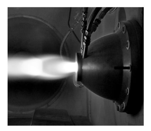
Figure 2.28.: Plasmatron subsonic (top) and supersonic (bottom) plasma jet.
