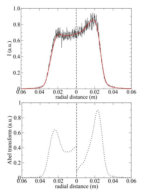
Figure 3.3.: Top: Asymmetric intensity profiles: experimental (black) and filtered (red). Bottom: Corresponding Abel transform.
