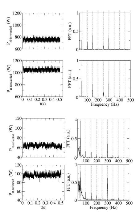
Figure 2.15.: Forwarded (top) and reflected (bottom) RF microwave power at 0.1  $\rm g.s^{-1}$  with associated Fourier fluctuation analysis.
