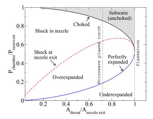
Figure 2.25.: Nozzle operating map ( $\gamma=1.3$ ) and hydrodynamic regimes associated to experimental configurations of Plasmatron and microwave plasma sources.
