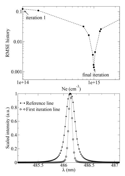
Figure 4.7.: Top: RMSE distribution. Bottom: Reference and computed  $\mathbf{H}_{\beta}$  line at the first iteration
