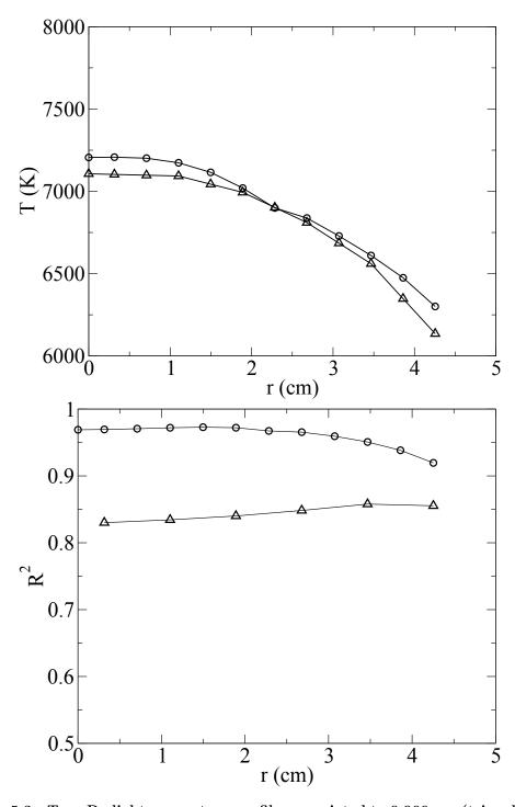
Figure 5.3.: Top: Radial temperature profiles associated to  $0.066~\mathrm{nm}$  (triangle) and  $0.3~\mathrm{nm}$  (circle) spectral resolution fitting. Bottom: Squared correlation coefficient associated to  $0.066~\mathrm{nm}$  (triangle) and  $0.3~\mathrm{nm}$  (circle) spectral resolution fitting.
