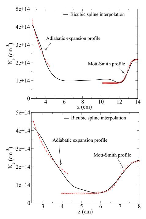
Figure 7.16.: Electron density interpolated profile on the symmetry axis (black). Analytical expansion and shock profiles (red). Case 1  $p_b = 6$  mbar (top), Case 2  $p_b = 12$  mbar (bottom).
