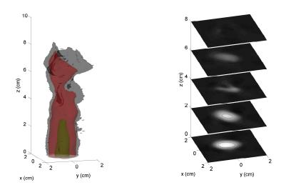
Figure 2.11.: Instantaneous emission distribution - low mass flow rate case (0.9 g.s^{-1}, 0.8 kW).
