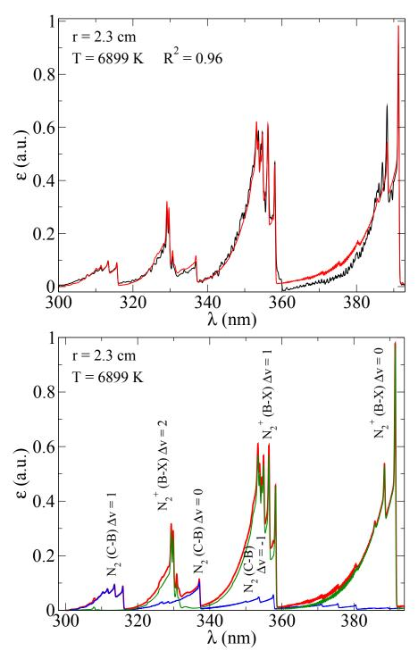
Figure 5.5.: Top: Best fit accounting for  $N_2^+$ ,  $N_2$  and CN molecular systems. Bottom: Synthetic representation of the relative contribution of each system.
