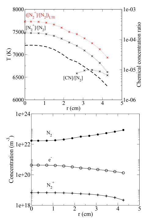
Figure 5.7.: Top: Temperature (dashed line) and species concentration ratio  $N_2^+/N_2$  (cross) radial profiles. Bottom: Radial LTE concentration computed using CEA equilibrium tool [66].
