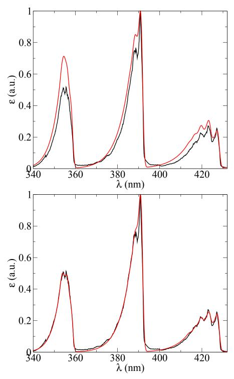
Figure 7.19.: Top: Initial fitting condition at  $T_{rot.}=T_{vib.}=6000~{\rm K}$  (right). Bottom: Best fit obtained for  $T_{rot.}=5354~{\rm K}$  and  $T_{vib.}=5681~{\rm K}$
