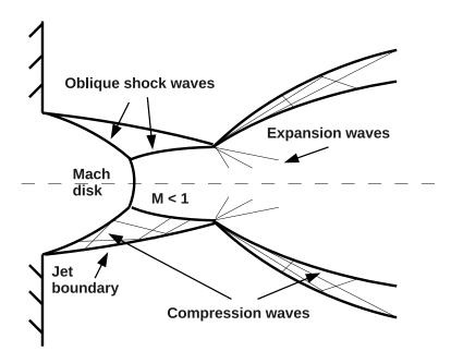
Figure 6.2.: Oblique shocks that create the first compression cell in over-expanded flow.
