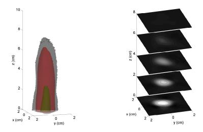
Figure 2.12.: Mean emission distribution - low mass flow rate case (0.9 g.s $^{-1}$ , 0.8 kW).
