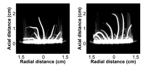
Figure 2.6.: Argon streamer regime at 0.6 kW (left) and 1.0 kW (right) microwave power.
