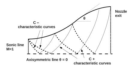
Figure 2.26.: Geometry of contoured nozzle defined by Anderson [63].
