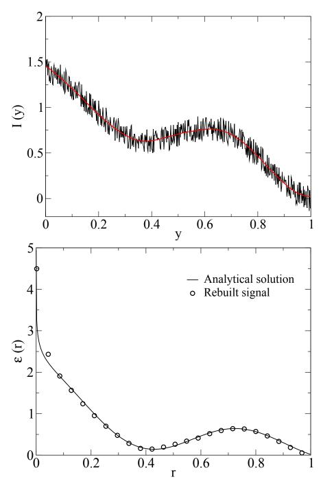
Figure 3.6.: Top: noisy profile and associated filtering. Bottom: Abel inversion results  ${\bf r}$
