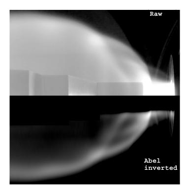
Figure 3.7.: Abel transform of plasma flow emission around heat flux probe.
