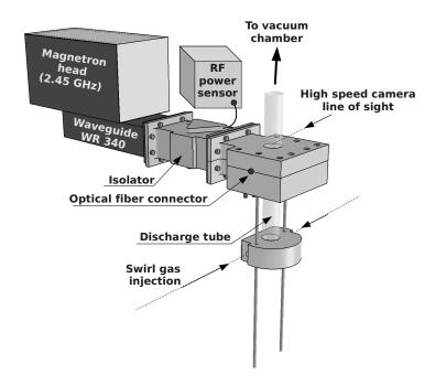
Figure 2.1.: Representation of VKI microwave plasma source.
