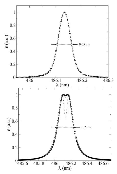
Figure 4.3.: Computations of  $H_{\beta}$  line shape with Stark and Doppler broadening at 10000 K and  $10^{14}$  (top) and  $10^{15}$  (bottom) cm<sup>-3</sup> electron density. VCS (dotted), MMM (dashed) and CS (circle)
