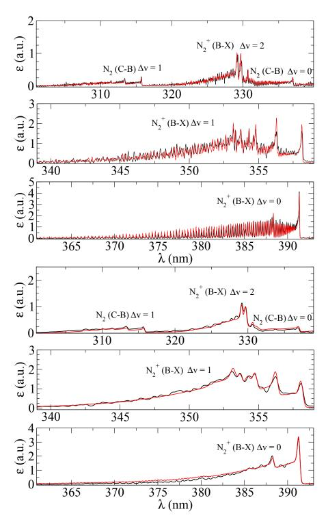
Figure 5.2.: Best fits executed at 0.066 nm (first three figures) and 0.3 nm (last three figures) spectral resolution. Experimental (black) and computed equilibrium (red) spectra on the jet centerline.
