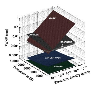
Figure 4.2.:  $H_{\beta}$  line shape broadening contributions as a function of the electron number density and temperature in LTE air plasma at atmospheric pressure.
