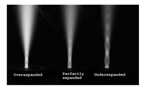
Figure 2.27.: Supersonic microwave discharge system (top) and plasma flow regimes (bottom).
