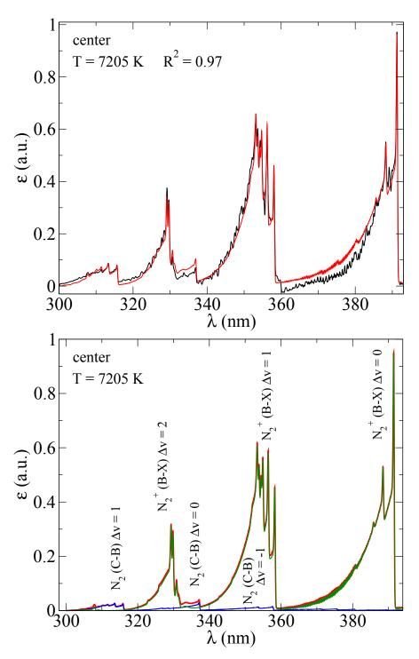
Figure 5.4.: Top: Best fit accounting for  $N_2^+$ ,  $N_2$  and CN molecular systems. Bottom: Synthetic representation of the relative contribution of each system.
