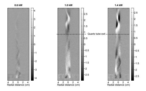
Figure 2.8.: Intensity fluctuation for  $0.3 \text{ g.s}^{-1}$  air plasma jet.
