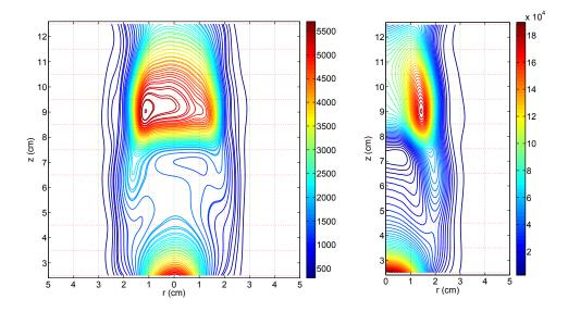
Figure 7.6.: Case 2 (p<sub>b</sub> = 12 mbar): Spectrally integrated radiance [W.m<sup>-2</sup>.sr<sup>-1</sup>] over [400-900] nm spectral range (left) and associated local emission [W.m<sup>-3</sup>.sr<sup>-1</sup>] (right).
