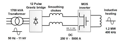
Figure 2.22.: Electrical scheme of VKI Plasmatron facility.
