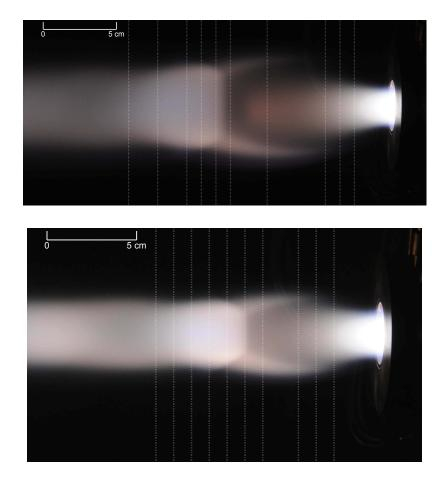
Figure 7.1.: Locations of line of sight measurements in supersonic air plasma jets at 6 mbar (top) and 12 mbar (bottom) back pressure conditions.
