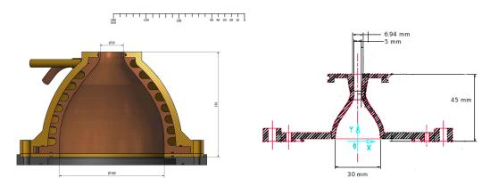
Figure 2.24.: Plasmatron converging throat (right) and MPT converging diverging nozzle (left) technical drawings.
