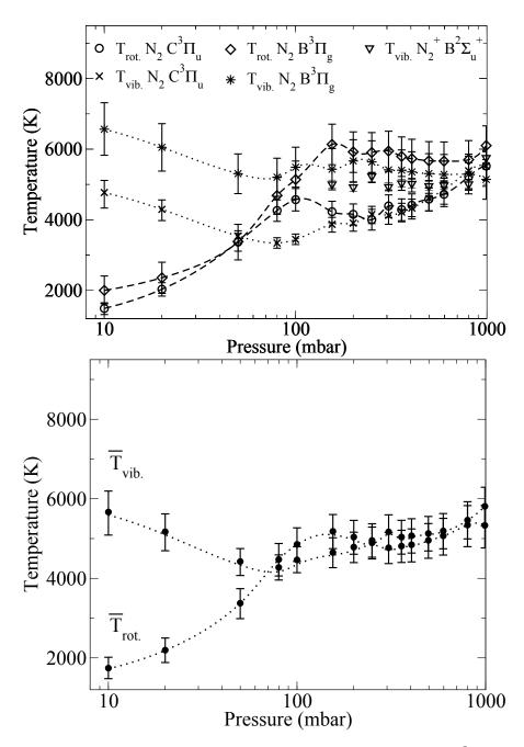
Figure 5.25.: Top: Rotational and vibrational temperatures of  $C^3\Pi_u$  and  $B^3\Pi_g$  states of  $\mathbf{N}_2$  and vibrational temperature associated to  $B^2\Sigma_u^+$  state of  $\mathbf{N}_2^+$ . Bottom: Corresponding geometric average temperatures.
