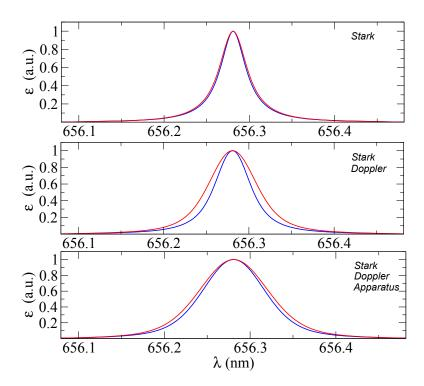
Figure 4.5.: Computed hydrogen  $H_{\alpha}$  spectral line shape broadening at  $N_e = 5.0 \times 10^{14}$  cm<sup>-3</sup>, T = 5000 K (blue), 15000 K (red).
