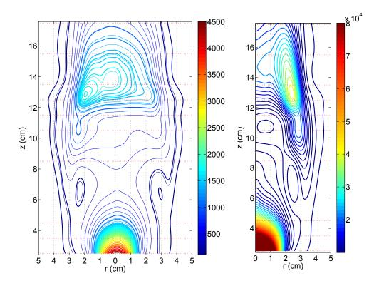
Figure 7.5.: Case 1 (p<sub>b</sub> = 6 mbar): Spectrally integrated radiance [W.m<sup>-2</sup>.sr<sup>-1</sup>] over [400-900] nm spectral range (left) and associated local emission [W.m<sup>-3</sup>.sr<sup>-1</sup>] (right).
