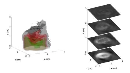
Figure 2.13.: Instantaneous emission distribution - high mass flow rate case (1.3 g.s $^{-1}$ , 0.8 kW).
