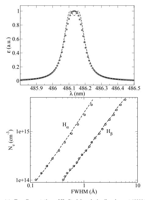
Figure 4.4.: Top: Computations of  $H_{\beta}$  Stark broadening line shape at 10000 K, 5.0  $\times$  10<sup>14</sup> cm<sup>-3</sup> electron density for various relative reduced mass  $\mu_r$  =5.0 (dashed), 1.0 (dotted), 0.5 (circle). Bottom: Stark broadening FWHM at  $T_e$  = 5000 K (dashed) and  $T_e$  = 10 000 K (circle) using CS simulation.
