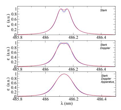
Figure 4.6.: Computed hydrogen  $H_{\beta}$  spectral line shape broadening at  $N_e = 5.0 \times 10^{14}$  cm<sup>-3</sup>, T = 5000 K (blue), 15000 K (red).
