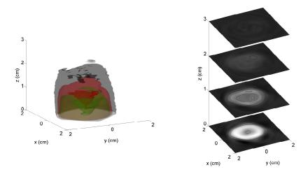
Figure 2.14.: Mean emission distribution - high mass flow rate case (1.3 g.s<sup>-1</sup>, 0.8 kW).
