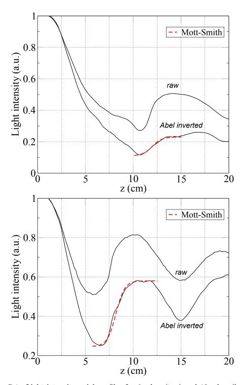
Figure 7.4.: Light intensity axial profiles for 6 mbar (top) and 12 mbar (bottom) back pressure conditions.
