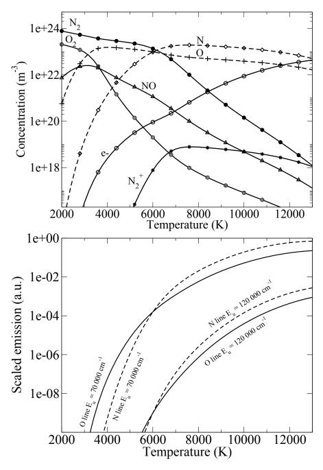
Figure 4.1.: Top: 273 mbar air plasma species concentration. Bottom: Scaled atomic emission.
