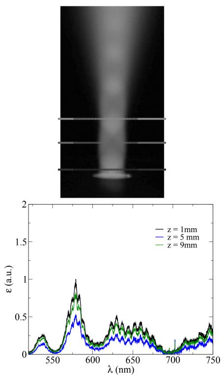
Figure 7.17.: Top: Over-expanded jet. Bottom:  $N_2$  First Positive spectra along the axis of the over-expanded jet.
