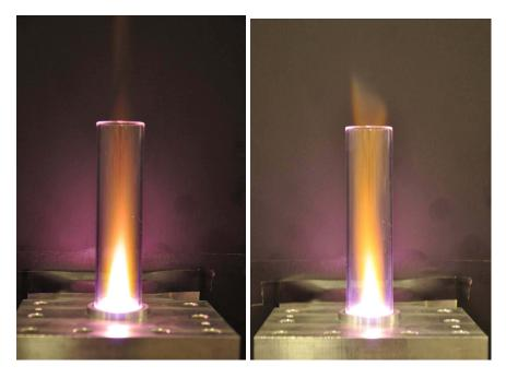
Figure 2.5.: 0.8 kW  $N_2$  plasma flow at 0.1 g.s<sup>-1</sup> (left) and 1.5 g.s<sup>-1</sup> (right).
