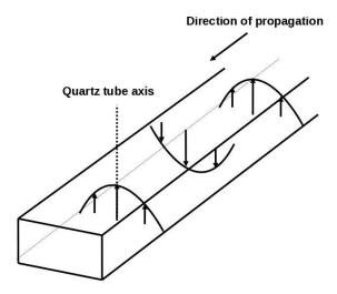
Figure 2.2.: Electric field distribution for  $TE_{10}$  mode.
