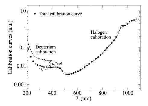
Figure 2.18.: Relative calibration curve using halogen/deuterium source.
