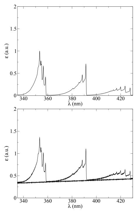
Figure 4.10.: Synthetic spectrum -  $T_{rot} = 7000 \text{ K}$ ,  $T_{vib} = 12000 \text{ K}$  - (top). Synthetic noisy spectrum and additional noisy background (bottom).
