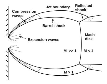
Figure 6.1.: Wave structures that create the first expansion cell in under-expanded flow.
