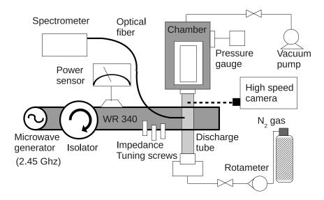
Figure 5.20.: Schematic of the setup.
