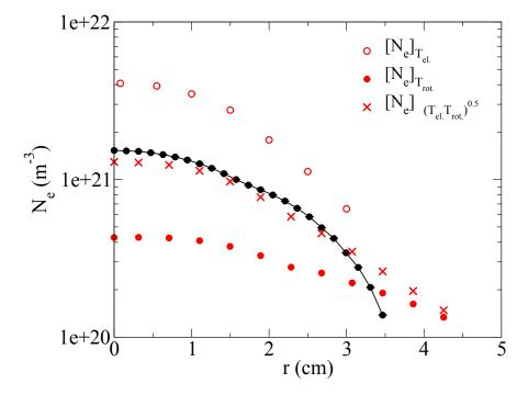
Figure 5.19.: Measured electronic density profile (black) and density computed at equilibrium (red).
