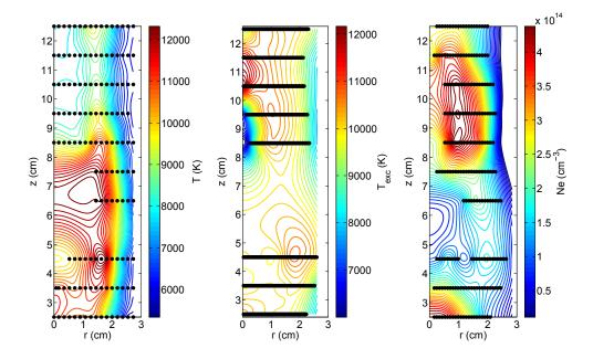
Figure 7.15.: Case 2 (p<sub>b</sub> = 12 mbar): Interpolated temperatures and electron density isocontours.
