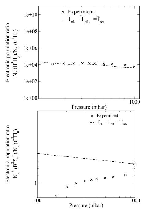
Figure 5.26.: Top: Electronic population density ratio  $N_{B^3\Pi_g}/N_{C^3\Pi_u}$ . Bottom: Electronic population density ratio  $N_{B^2\Sigma_u^+}/N_{C^3\Pi_u}$ . Experiment (cross) and theoretical calculation (red).
