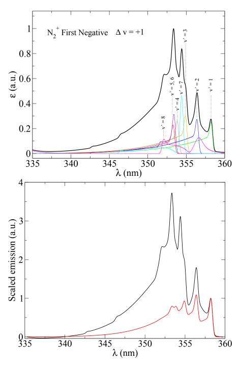
Figure 4.14.: Vibrational non-equilibrium synthetic spectrum and vibrational bands contribution (top) and first fitting iteration (bottom).
