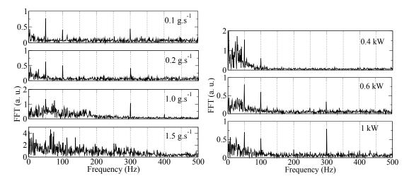
Figure 2.9.: Component frequencies of the emission fluctuation for 0.8 kW (left) and 0.3 g.s<sup>-1</sup> (right) air plasma jet (1 cm above the waveguide).
