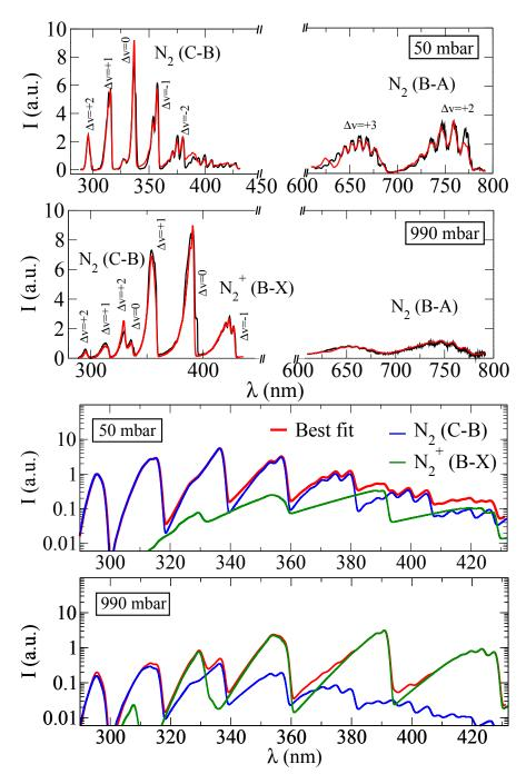
Figure 5.22.: Top: Experimental spectra (black) and their associated best fits (red). Bottom: Best fits (red) and resolved contribution of  $N_2$  2nd Positive (C-B) (blue) and  $N_2^+$  First Negative (B-X) (green) systems.
