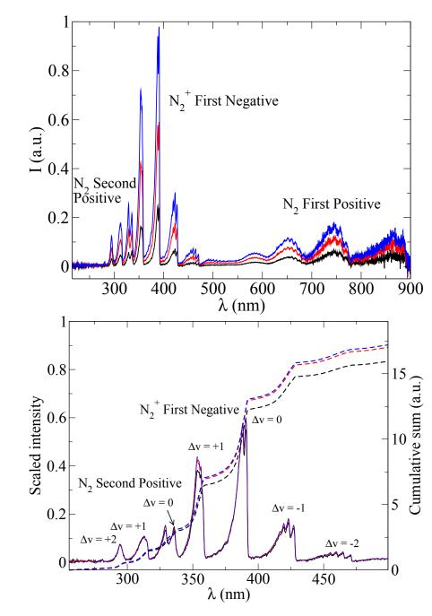
Figure 2.20.: Typical radiative signature of nitrogen discharge (top) operated at 0.6 (black), 0.8 (red) and 0.9 kW (blue) and associated scaled spectra (bottom).
