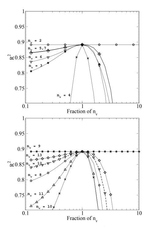
Figure 7.25.: Sensitivity of the correlation coefficient  ${\bf R}^2$  relative to the fraction of the vibrational population at  ${\bf T}_{rot.}={\bf 2708}$  K.
