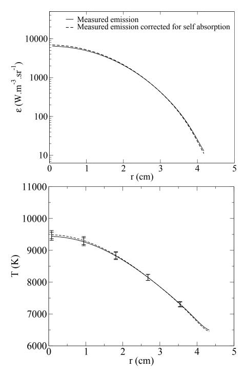
Figure 5.12.: Top: Measured (black) and theoretical (red) emission for nitrogen line at 742 nm. Bottom: LTE temperature profile (solid line) and temperature profile corrected for self absorption (dashed line).
