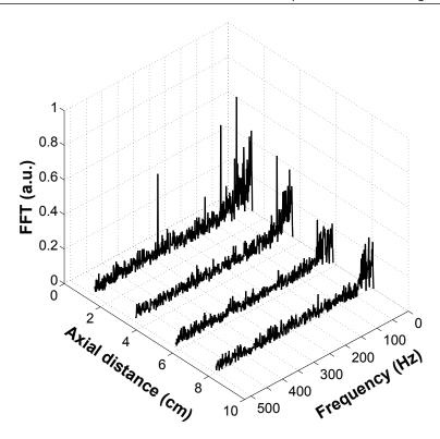
Figure 2.10.: Component frequencies of the emission fluctuation (air, 0.3 g.s $^{-1}$ , 0.8 kW).
