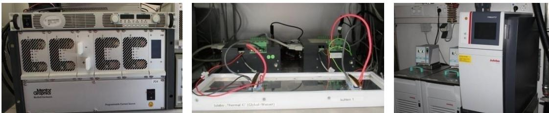
Figure 4.1: From the left to the right: a current source (200A), 2 devices under test mounted on the heat sink and connected to switching boxes, and both glycol and silicon oil thermostats.
