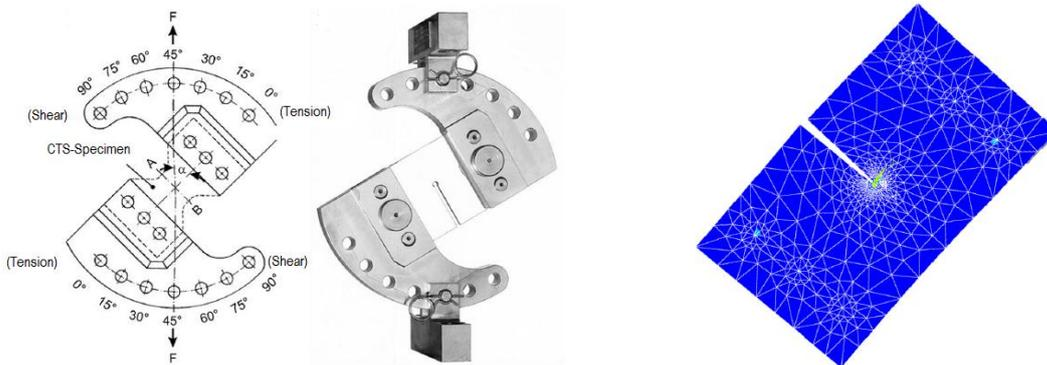
Figure 6.5: Schematic and picture of a CTS specimen [Ric85] and its corresponding FE model
