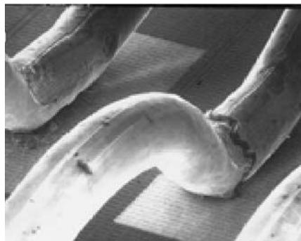
Figure 1.8: Heel cracking [Cia02]
