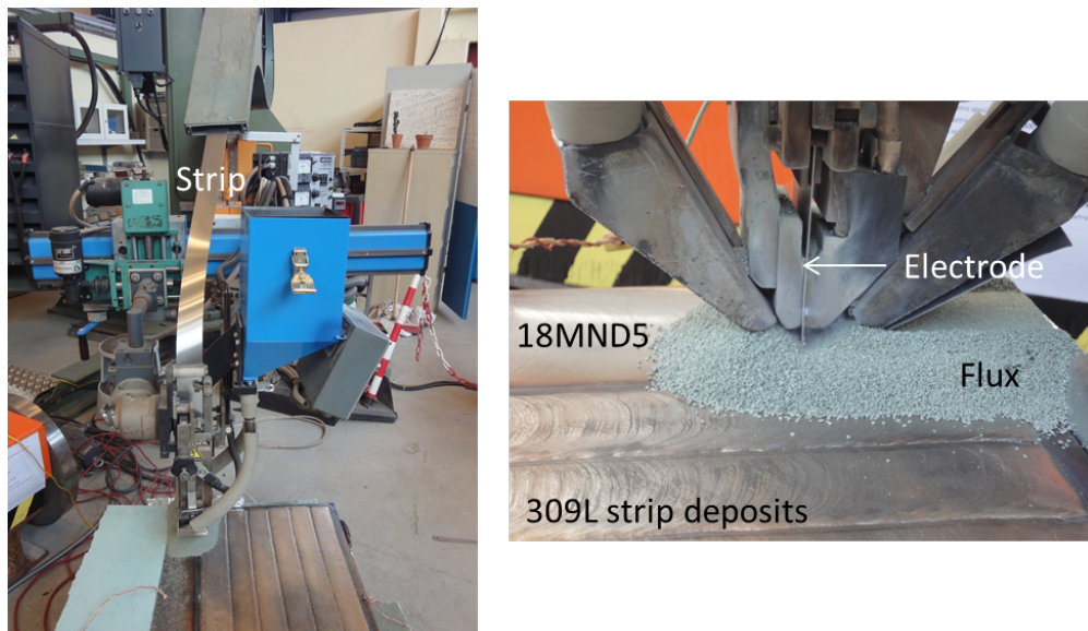
Figure 1.5: Strip electrode welding process
