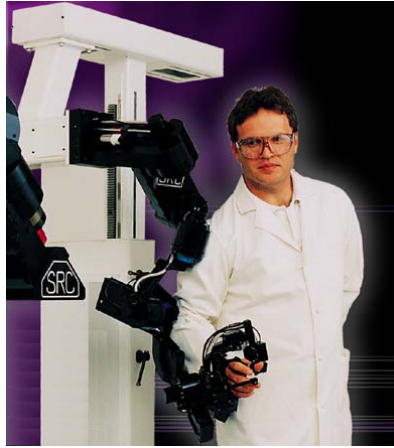
FIGURE 2.5: Bras exosquelette SARCOS (MAEKAWA et HOLLERBACH 1998).
