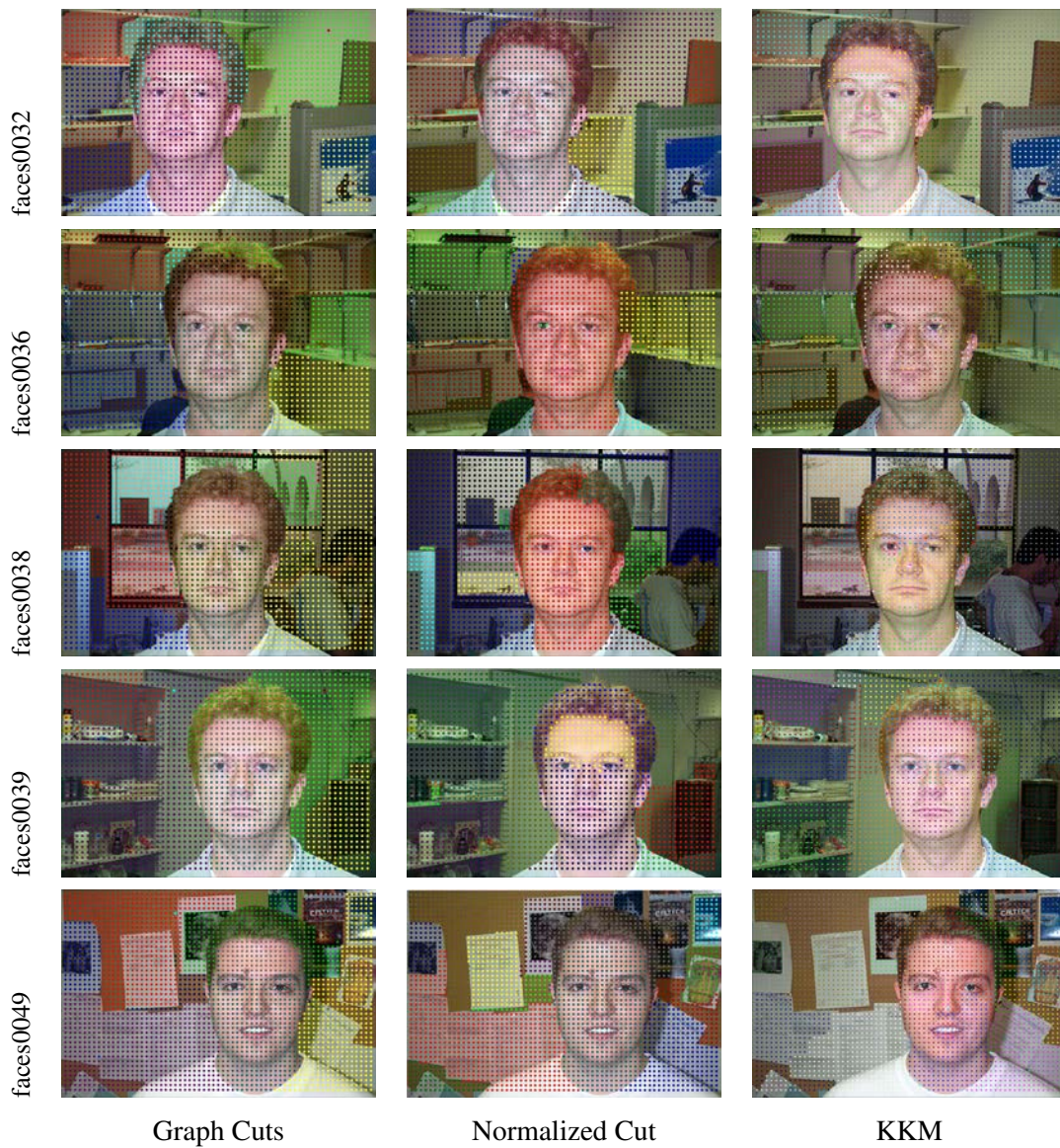
Figure 3.19: Examples of graph partitioning in 16 irregular subgraphs on five examples in category “faces” from Caltech-101 dataset by three methods: Graph Cuts (GC), Normalized Cut (NC), kernel k -means (KKM). This figure is better viewed in color .
