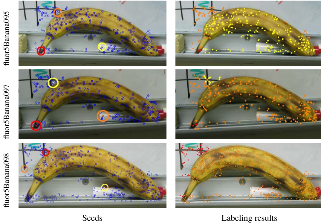
Figure 3.10: Examples of seeds selection in prominent keypoints approach. The stability of seeds is hardly reached due to the uncontrolled nature of the images available. All examples of images are from SIVAL dataset [10]. There are three seeds in each image, and these seeds are labelled with their own colors (in red, orange and yellow). This figure is better viewed in color .
