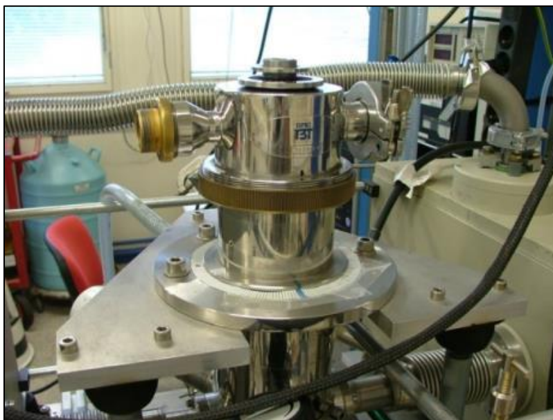
Figure 2.2 - The cryostat is the heart of the MICMOC apparatus where the samples are produced. Several openings allow the connection to the infrared spectrometer (visible on the right), the introduction line, and the UV lamp.
