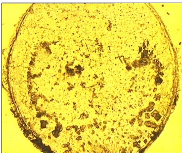
Figure 6.8 - The re-deposited residue mixed with enstatite film fragments after hot water extraction, viewed through the microscope. The diameter of the circular spot is about 8 mm. The yellow color is due to the ZnSe window substrate.
