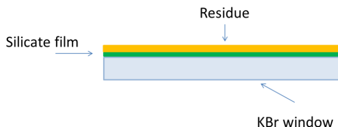
Figure 6.1 - Scheme of a sample constituted by an organic residue produced onto an amorphous silicate thin film (enstatite or forsterite) previously deposited on a KBr window.
