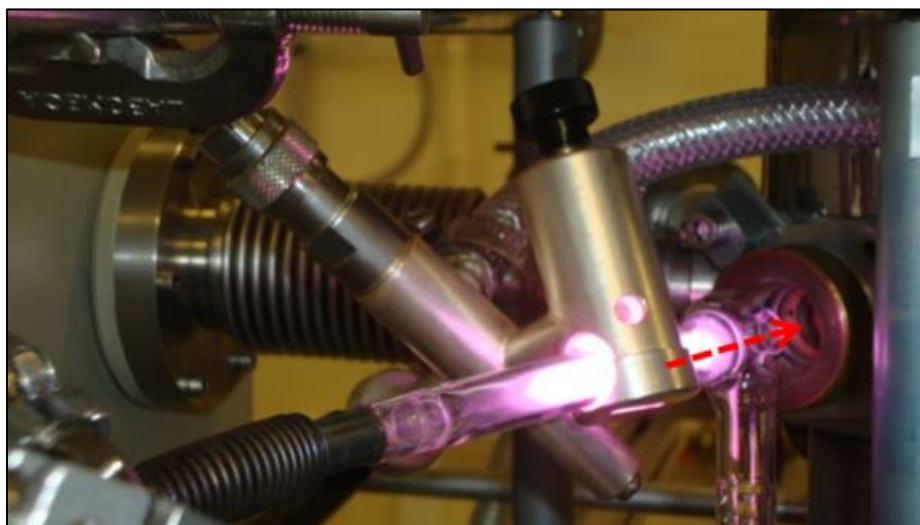
Figure 2.3 - The microwave-stimulated hydrogen flow discharge lamp provides the UV photon flux to irradiate the ice sample. The pink color is a characteristic of pure hydrogen plasma. The arrow indicates the direction toward the sample through the interface with the cryostat.
