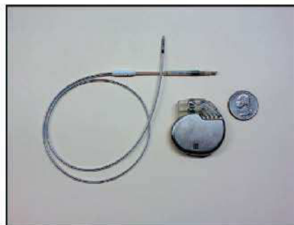
Figure 3.1 Pacemaker lead (left) and canister (right). The helix of the lead tip is extended. Shown is a dual-chamber pacemaker (atrial and ventricular ports).
