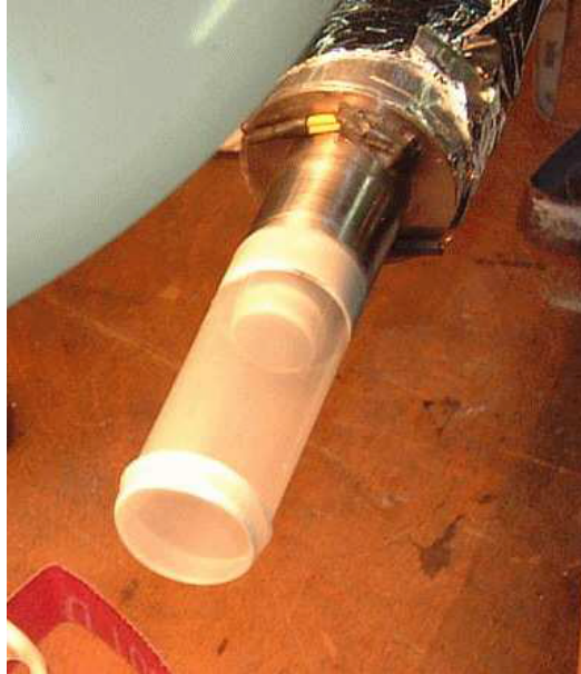
Figure 2.2: The liquid hydrogen target vessel with a diameter of 2.5 cm. The entrance window is glued on a stainless steel cylinder.
