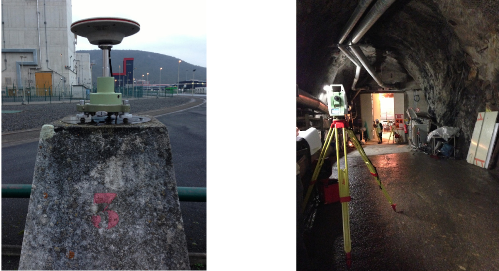
Figure 7.3: ( left ) GPS acquisition of the reference pillar #3 at the Chooz nuclear power plant. ( right ) A step of the polygonal route to the far laboratory, from [181].
