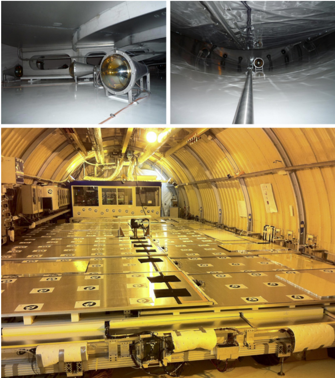
Figure 3.7: Pictures of the Double Chooz far detector, from [112]. ( top ) Inner veto views with the special orientation of the PMTs. ( bottom ) Outer veto covering the detector with the chimney in the middle for the deployment of radioactive sources.
